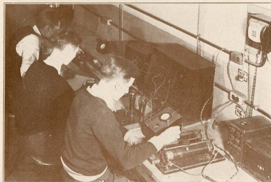
RADIO RECEPTION—TESTING RECTIFIER TUBES FOR POWER PACKS
