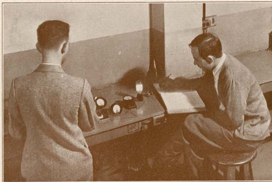
THE GLOW TUBE—DETERMINING CHARACTERISTICS OF A TELEVISION GLOW TUBE
