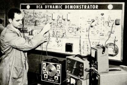
Important in the study of electronics is a knowledge of the triode. Here the student is obtaining the plate characteristics of a high vacuum triode, to determine the characteristics of the tube. Career Note: National Association of Broadcasters estimated the U. S. had 37,600,000 families in 1947, of whom 35,000,000, or 93 per cent, had radios.
