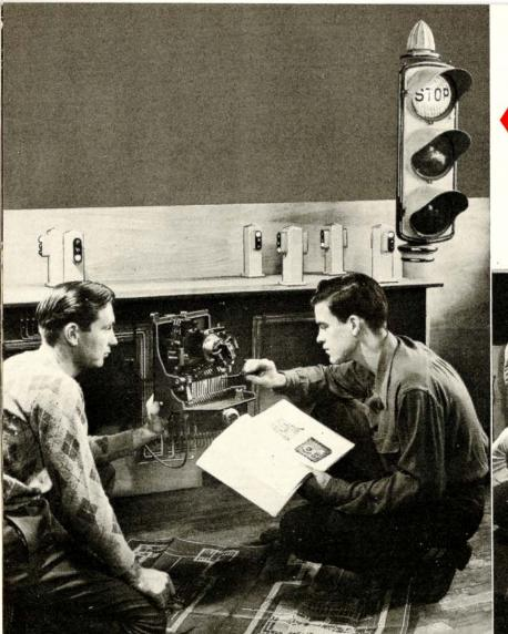
A model traffic signal system is used in this experiment to check for continuity, to study the circuits and to learn the operating characteristics of the various mechanisms.
