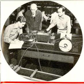
Under the guidance of an instructor, this student measures characteristics of 220-110 volt transformers in the Milwaukee School of Engineering's A-C testing laboratory. Career Note: Power is the common physical denominator of modern civilization.
