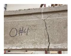
Figure E- 46. Offset #4 side cracks.
