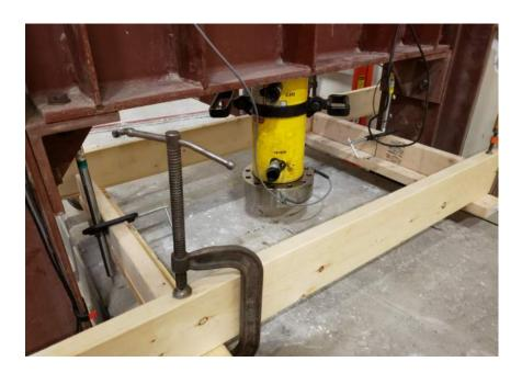
Figure 17. LVDT setup at midspan.
