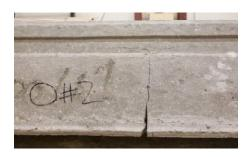
Figure E- 34. Offset #2 side cracks.
