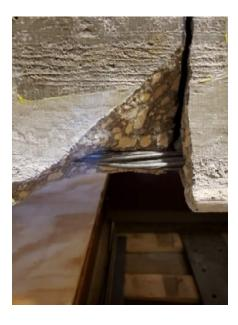
Figure E- 22. Center #3 exposed strand in crack.
