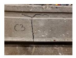
Figure E- 20. Center #3 side cracks.
