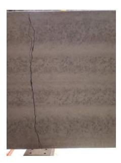
Figure E- 45. Offset #4 tension cracks.
