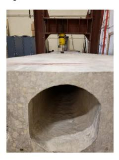
Figure E- 26. Offset #1 concentrated load location.
