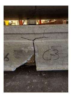
Figure E- 21. Center #3 side cracks.
