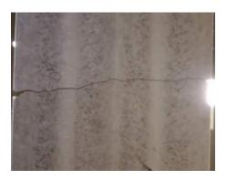
Figure E- 33. Offset #2 tension cracks.
