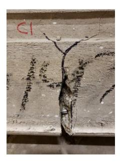
Figure E- 6. Center #1 side cracks.
