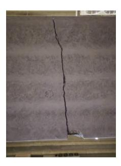
Figure E- 19. Center #3 tension cracks.
