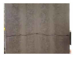
Figure E- 39. Offset #3 tension cracks.
