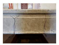
Figure E- 5. Center #1 side cracks.
