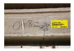
Figure E- 40. Offset #3 side cracks.
