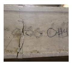
Figure E- 47. Offset #4 side cracks.
