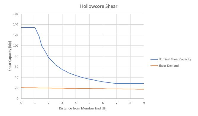
Figure 12. Shear envelope and member capacity.
