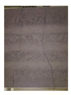
Figure E- 4. Center #1 tension cracks.
