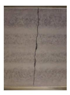
Figure E- 13. Center #2 tension cracks.
