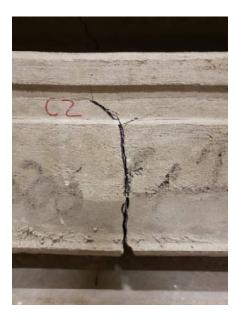
Figure E- 14. Center #2 side cracks.
