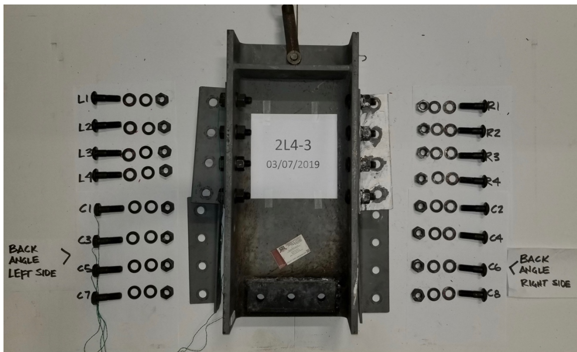
Figure 4.4-16: Typical underside view of specimen post-test showing angle deformation.
