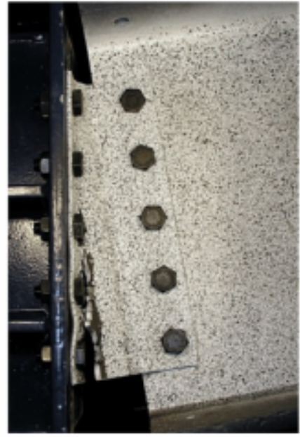
Figure 2.2-5: Tear propagation near column bolts (Oosterhof & Driver, 2015).
