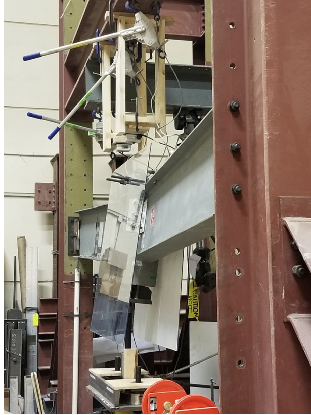
Figure 4.4-2: Typical LTB behavior of a 2L3 series specimen during testing.
