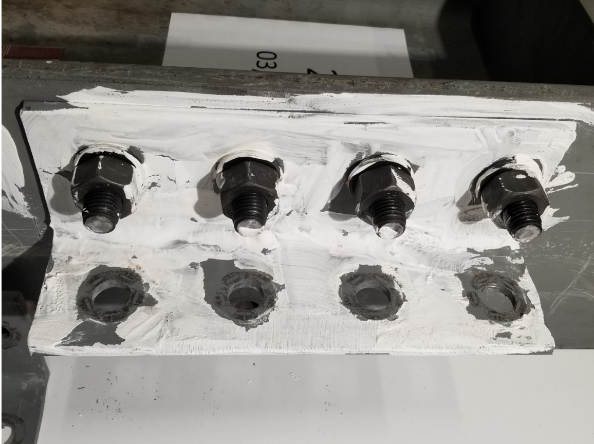
Figure 4.4-20: Plaster flake on specimen 2L4-1.
