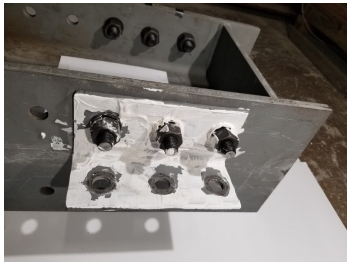
Figure 4.4-7: Enlargement of plaster application on test specimen 2L3-2, typical of 2L3 series tests.
