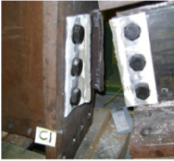
Figure 2.3-4: Specimen C1 failure (Gong, 2017).
