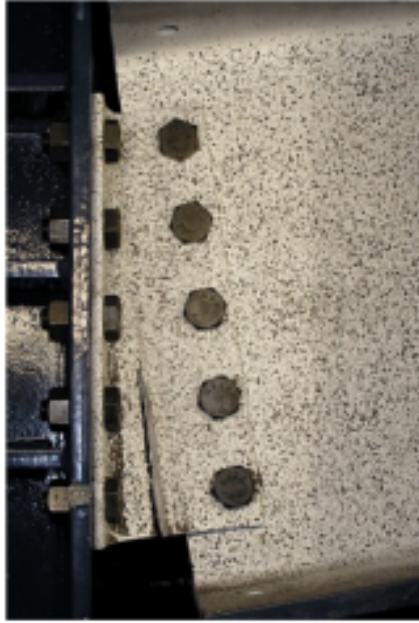
Figure 2.2-4: Tear propagation near the heel (Oosterhof & Driver, 2015).
