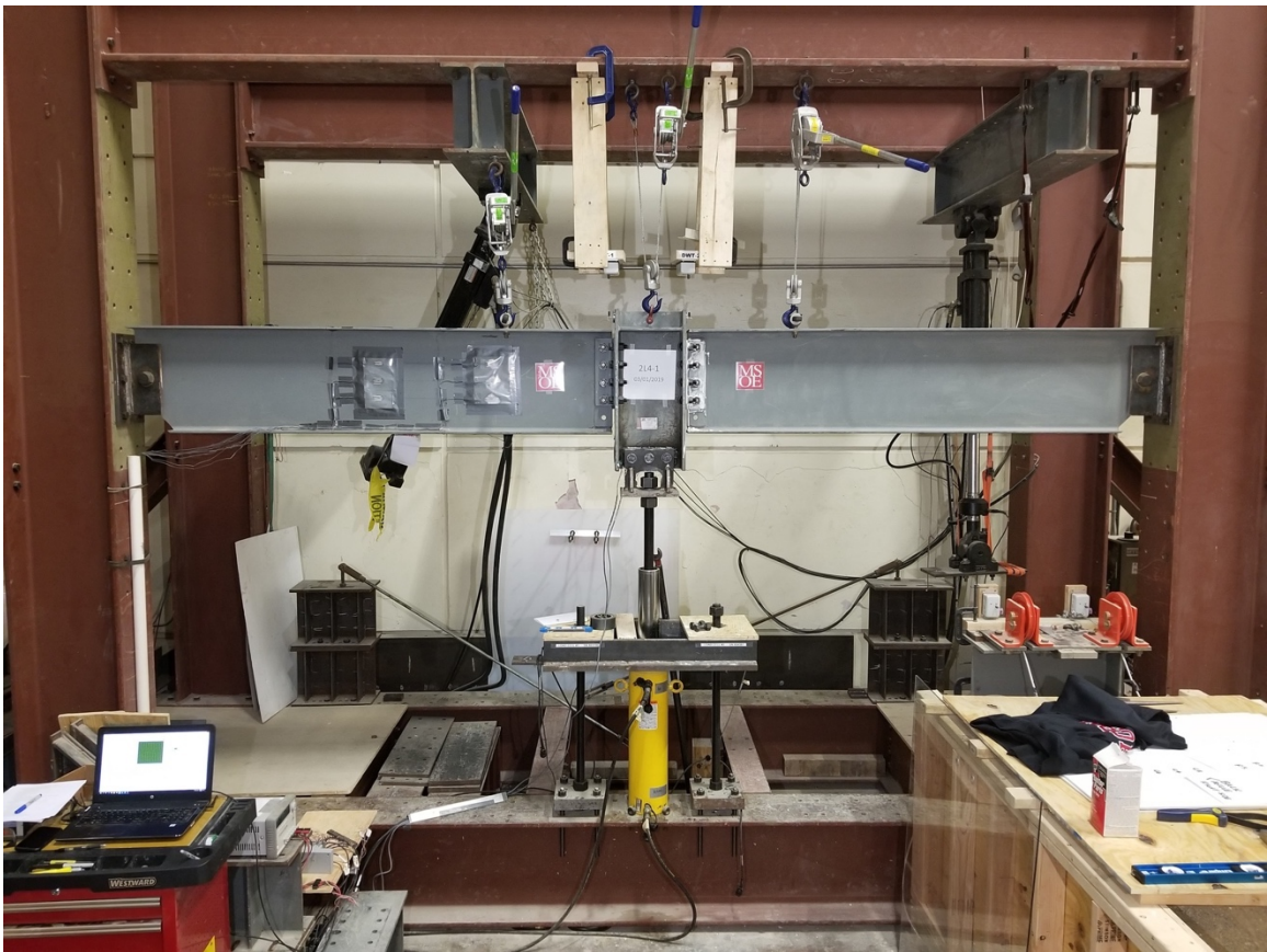
Figure 4.4-13: Typical 2L4 assembly before testing.
