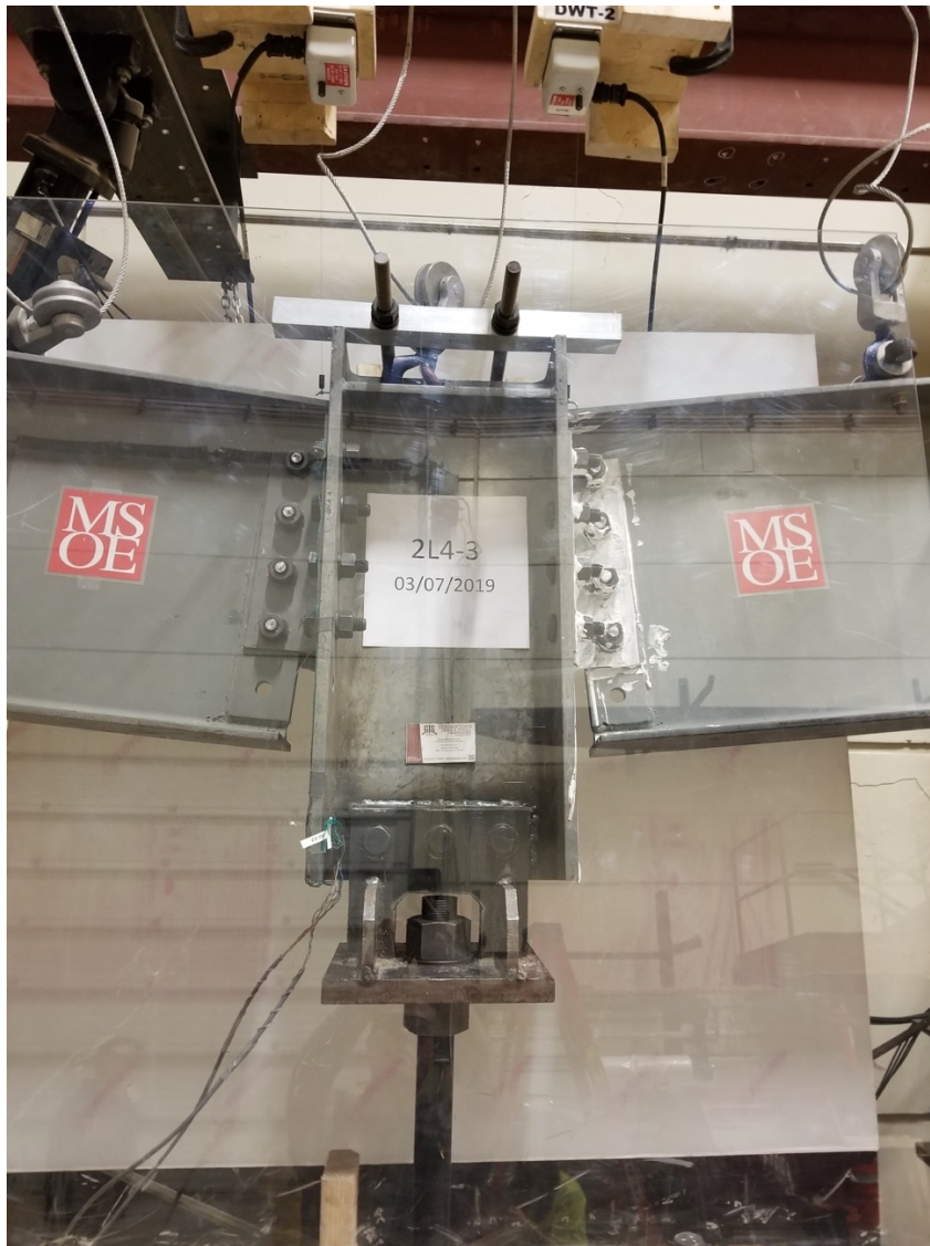
Figure 4.4-15: Typical 2L4 specimen post-test.
