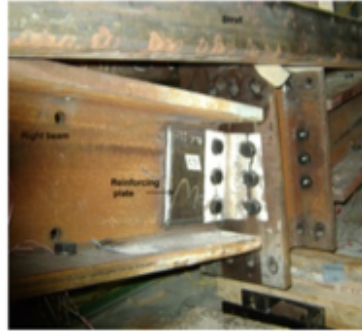
Figure 2.3-5: Specimen C2 failure (Gong, 2017).
