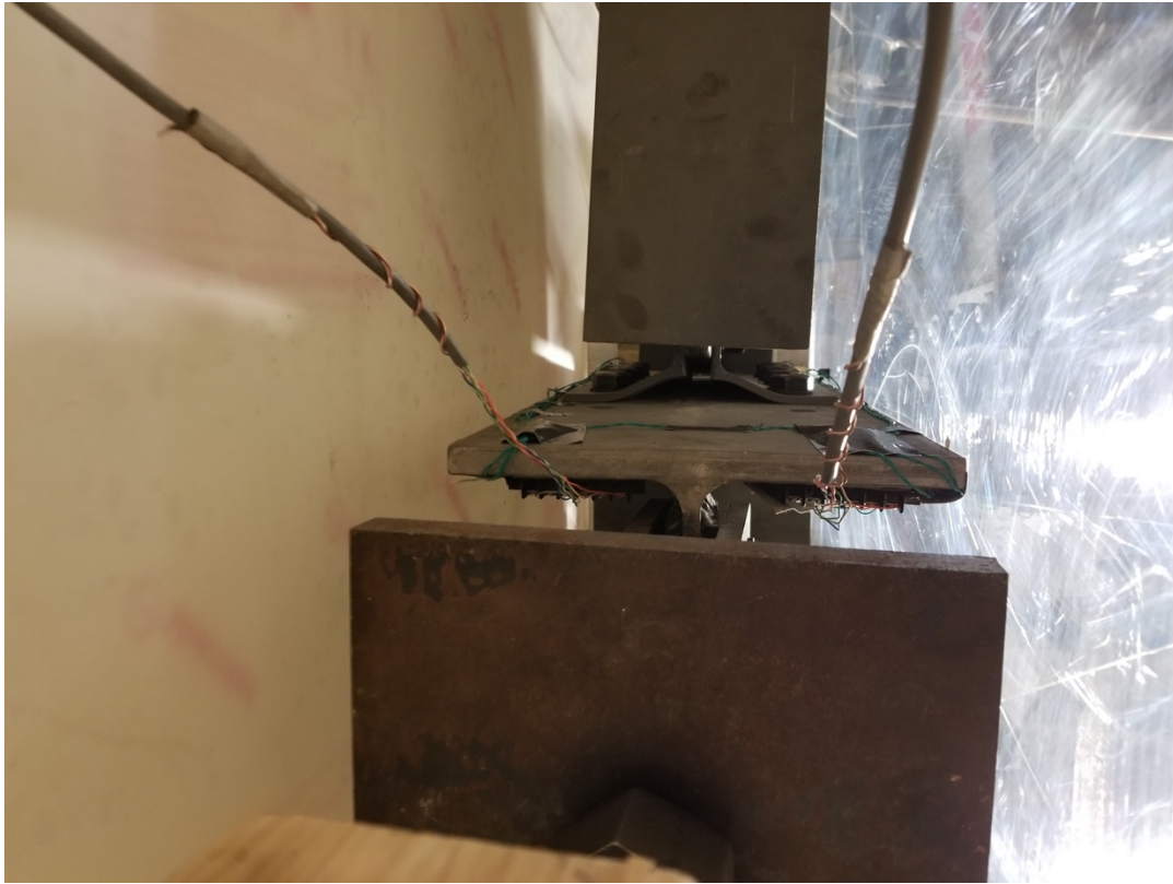
Figure 4.4-16: Typical underside view of specimen post-test showing angle deformation.
