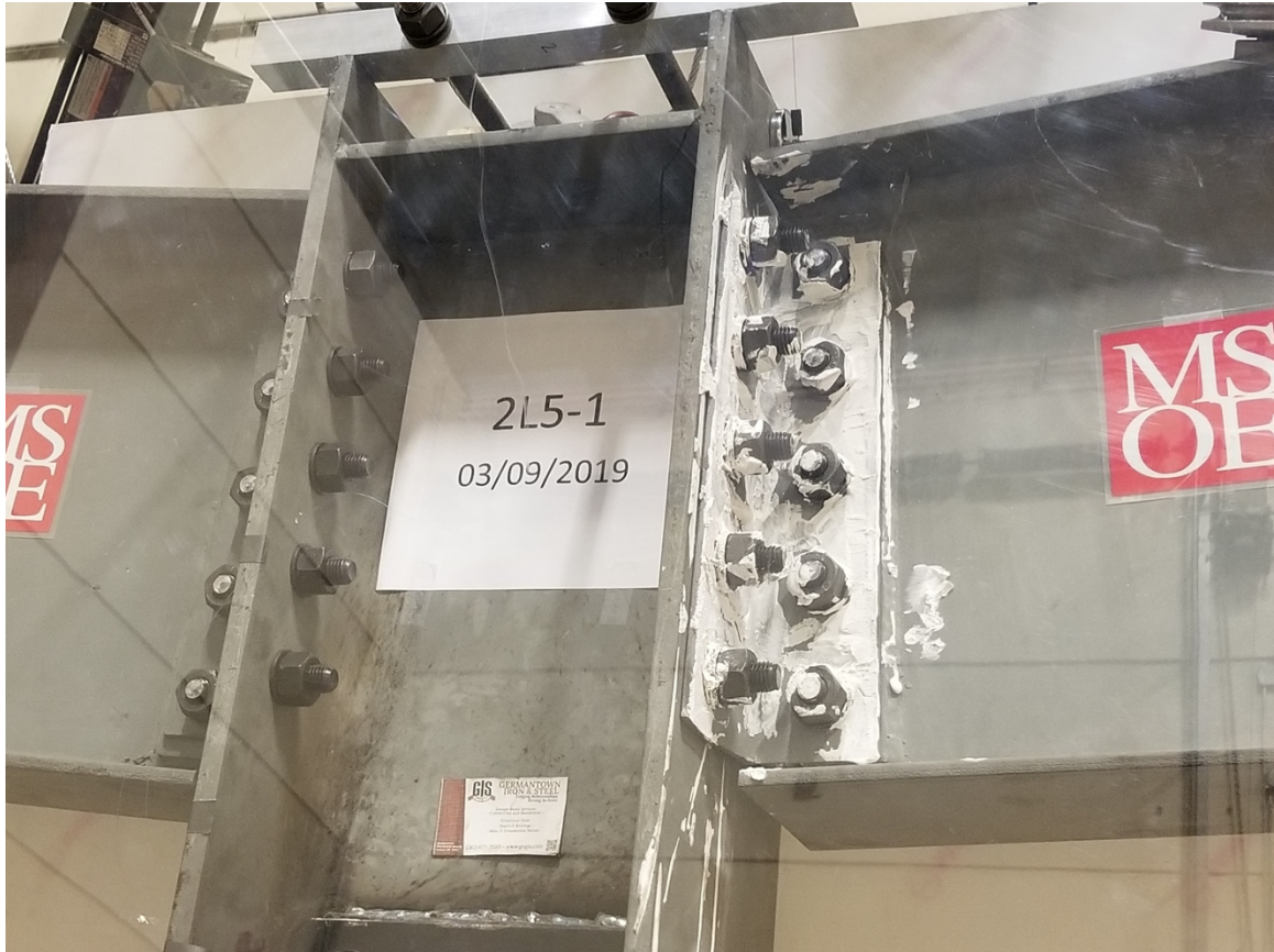
Figure 4.4-32: Plaster flake on specimen 2L5-1. Typical for 2L5 series of tests.
