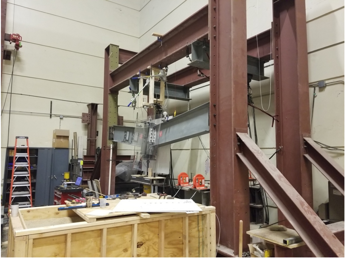
Figure 4.4-14: Typical LTB behavior of 2L4 series specimen during testing.
