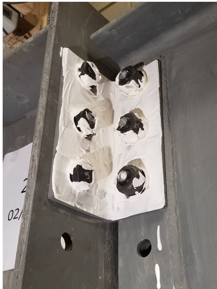
Figure 3.4-1: Plaster application on 2L3 specimen.
