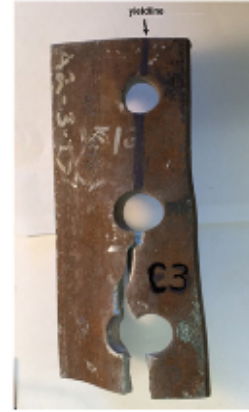
Figure 2.3-6: Tear along C3 specimen (Gong, 2017).
