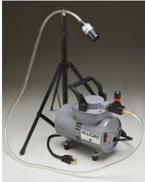
Figure 3. Air pump with cassette as used in sampling lead entrained in air. Adapted from “Detectors” by AFC International, Inc., n.d., para. 1. Retrieved from http://www.afcintl.com/diaphragm-area-sampling-pmp-1.aspx .
