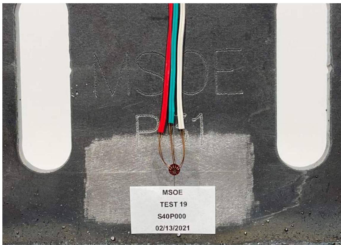
Figure D-70: Close-up View on Rosette of S40P000.
