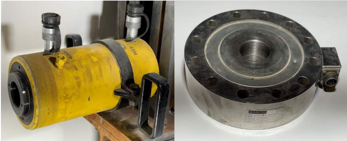
Figure 3-8: Enerpac Hydraulic Actuator (left) and Sensotec Load Cell (right).
