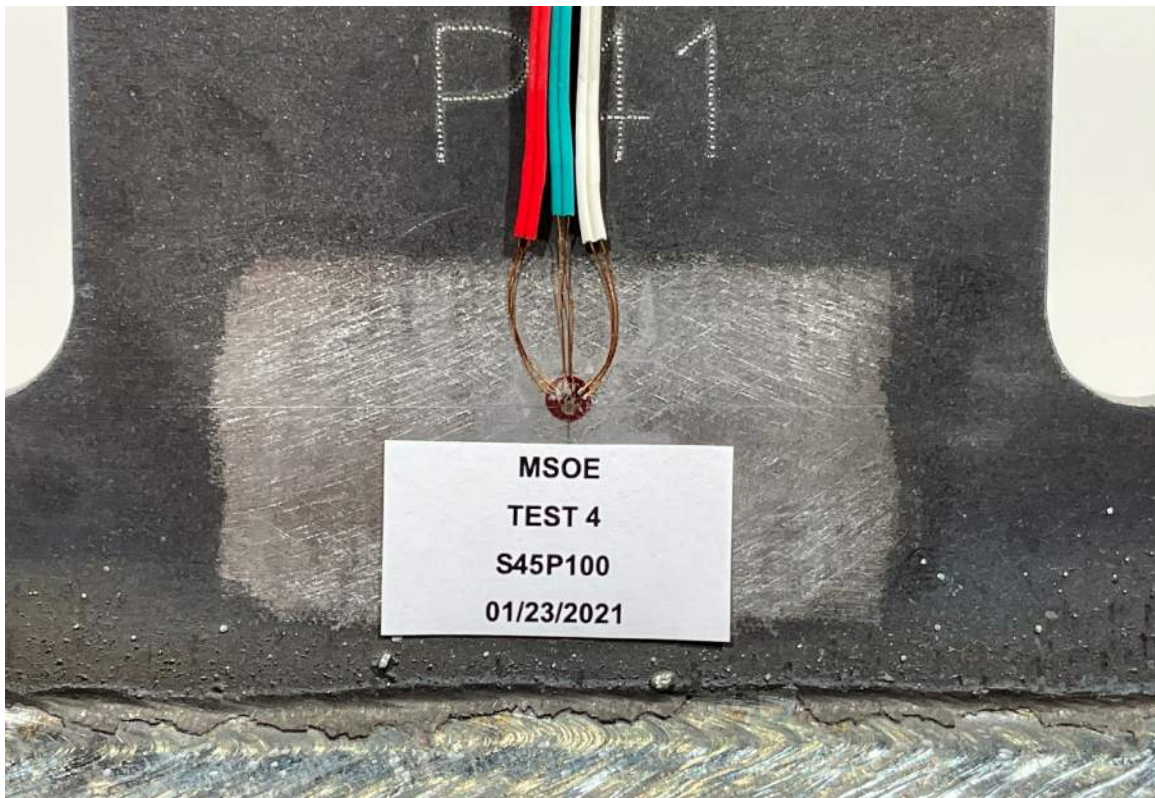
Figure D-16: Close-up View on Rosette of S45P100.
