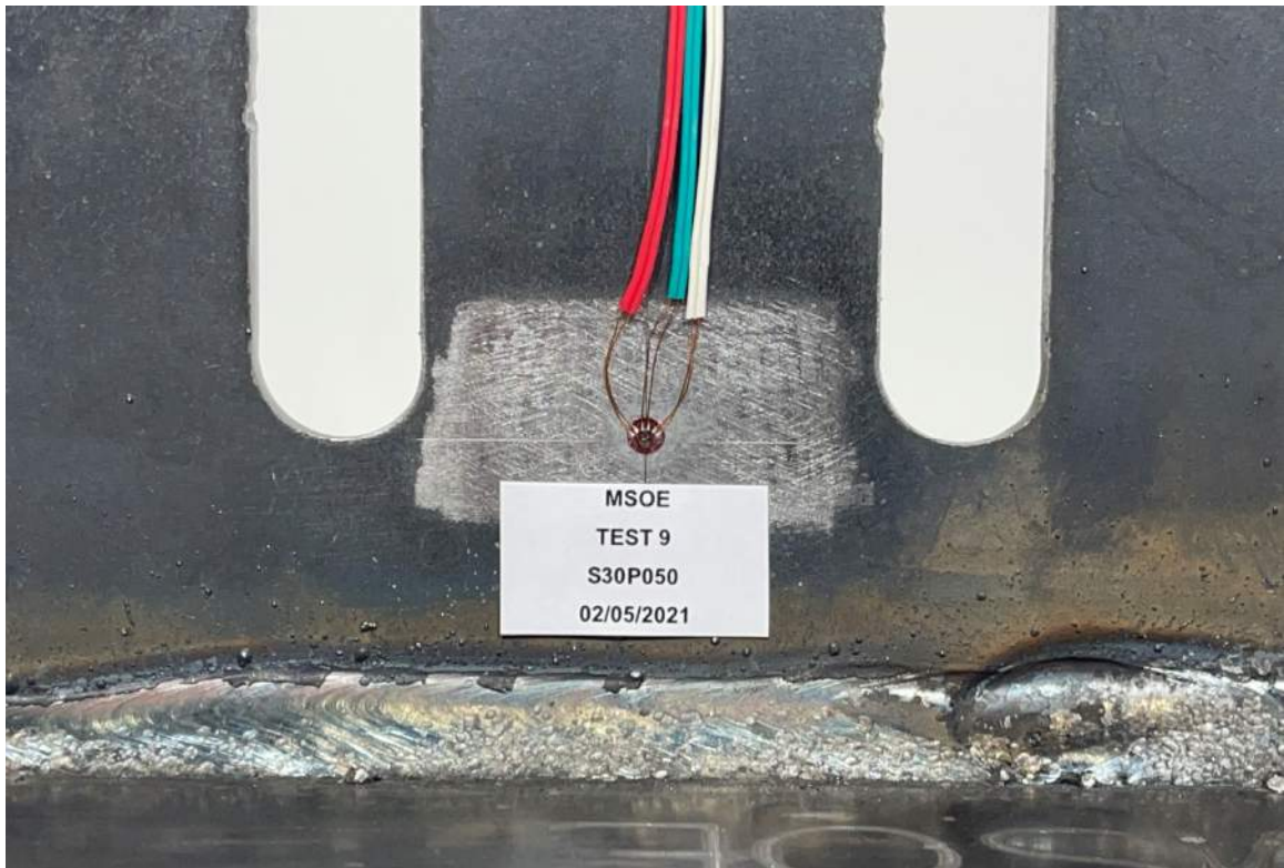
Figure D-33: Close-up View on Rosette of S30P050.
