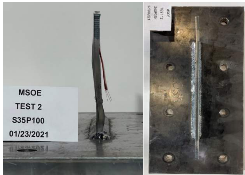
Figure 4-2: Local Out-of-Plane Buckling on Loaded Edge (Left) and Top of Specimen (Right).
