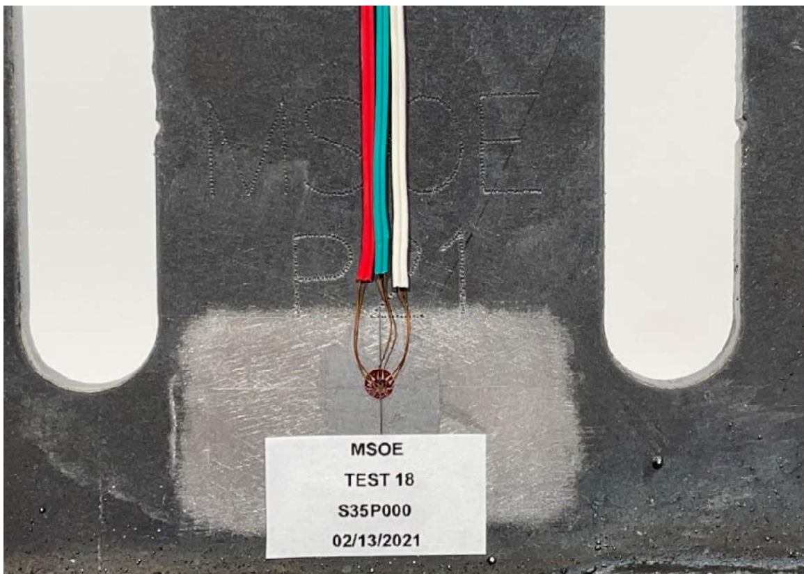
Figure D-66: Close-up View on Rosette of S35P000.
