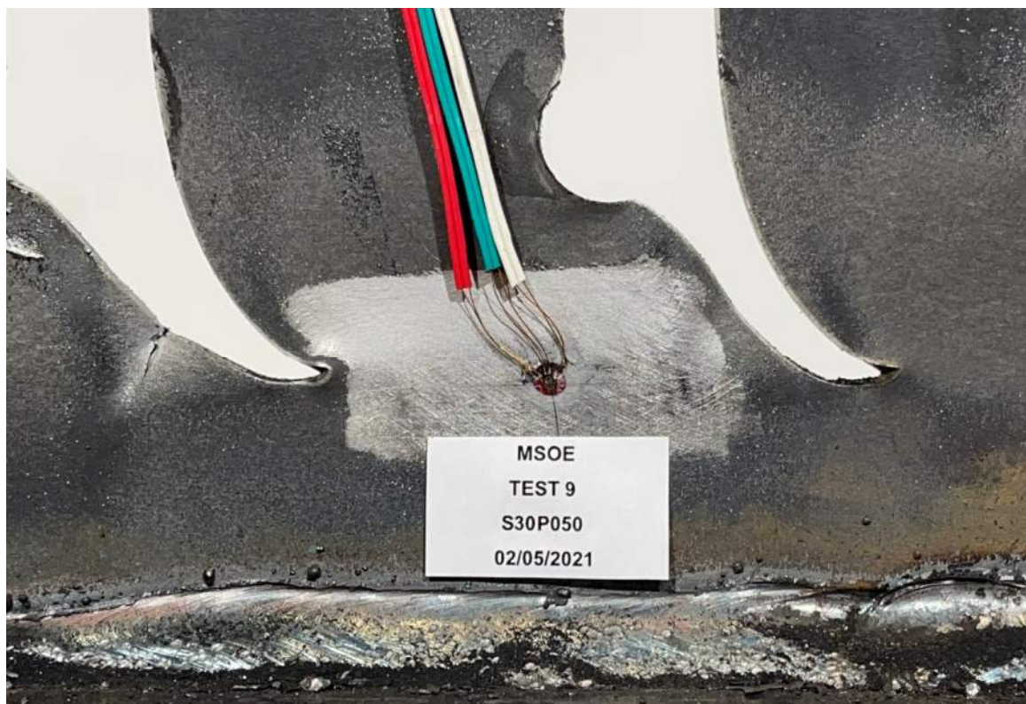
Figure E-34: Close-up View on Rosette of S30P050.
