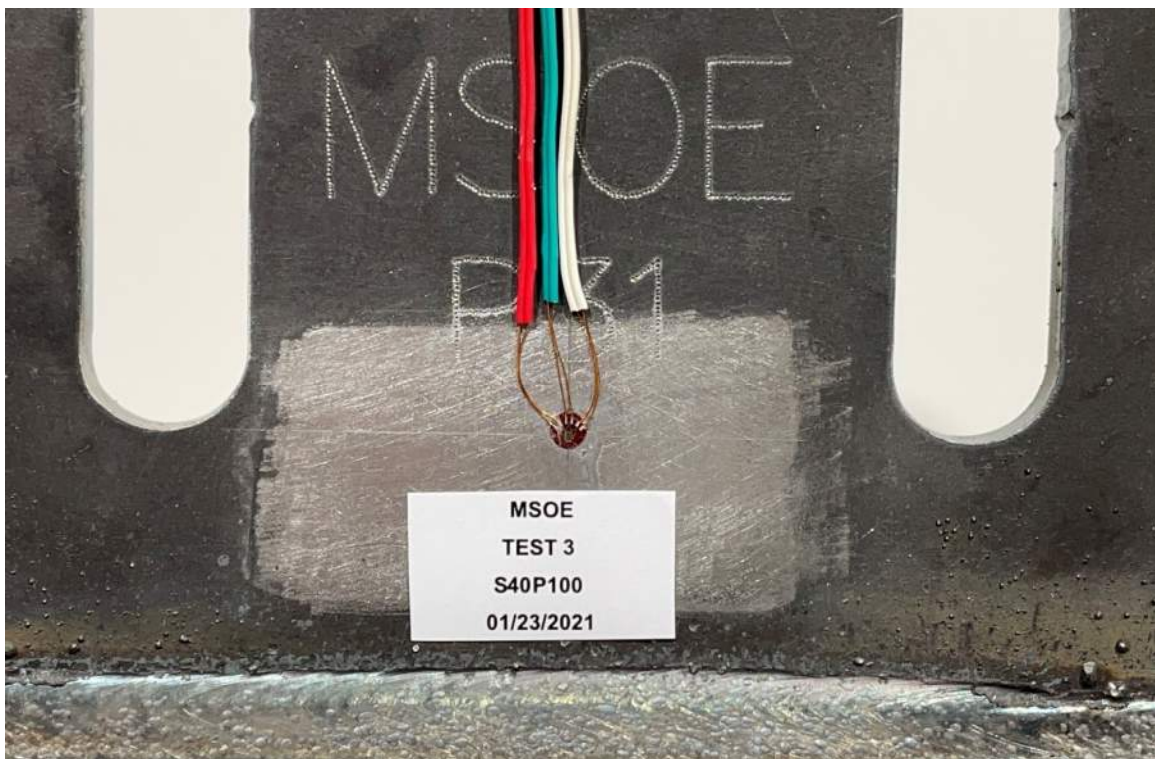
Figure D-12: Close-up View on Rosette of S40P100.
