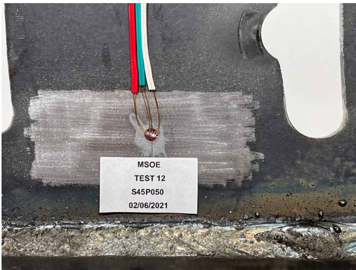
Figure E-47: Close-up View on Rosette of S45P050.
