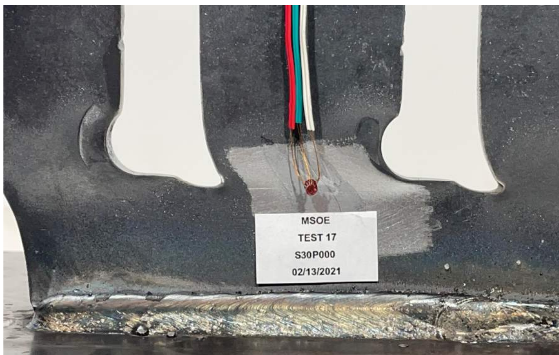
Figure E-64: Close-up View on Rosette of S30P000.
