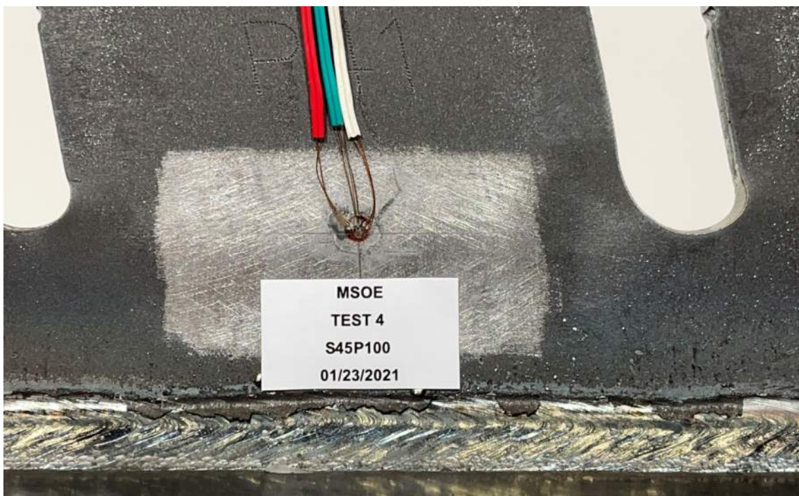
Figure E-16: Close-up View on Rosette of S45P100.
