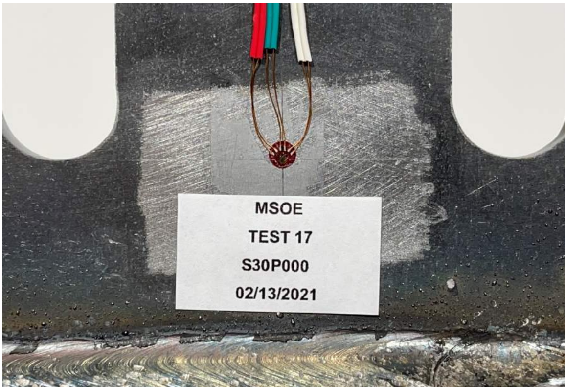
Figure D-62: Close-up View on Rosette of S30P000.
