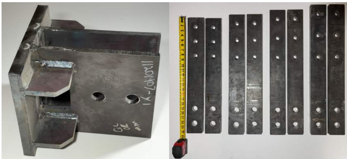
Figure 3-9: Yoke Assembly (left) and Sandwich Plates (right).
