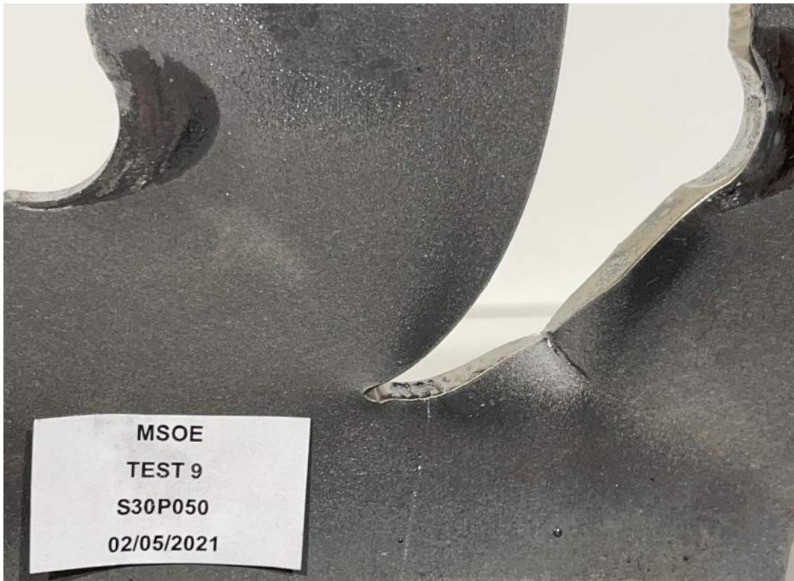
Figure E-35: Close-up View on Plate Tear of S30P050.
