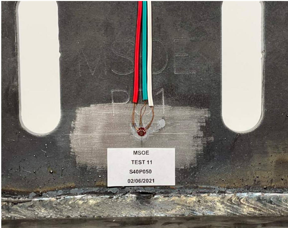
Figure D-41: Close-up View on Rosette of S40P050.
