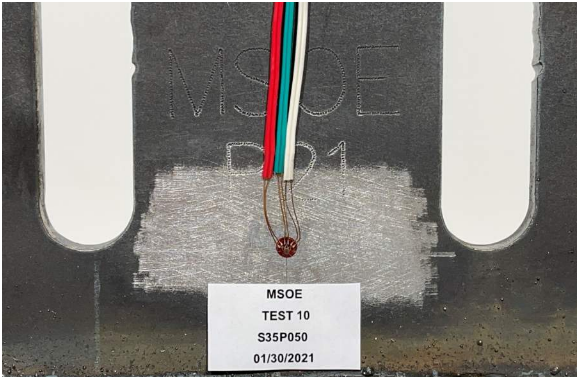
Figure D-37: Close-up View on Rosette of S35P050.
