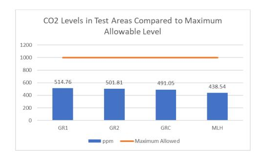
Note. Figure 6 depicts the average carbon dioxide levels of each test area in comparison to the maximum allowable level of 1000 ppm.
