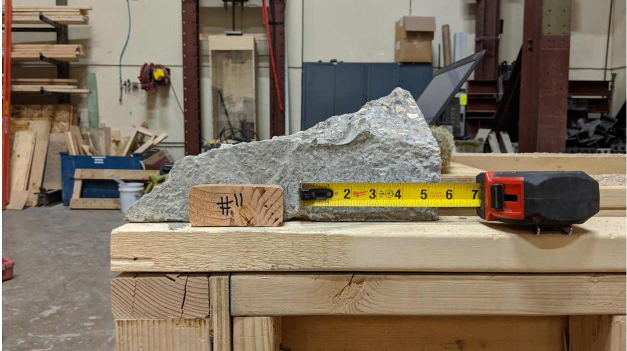
Figure A-43 – Front View of Test 11 Breakout Piece.
