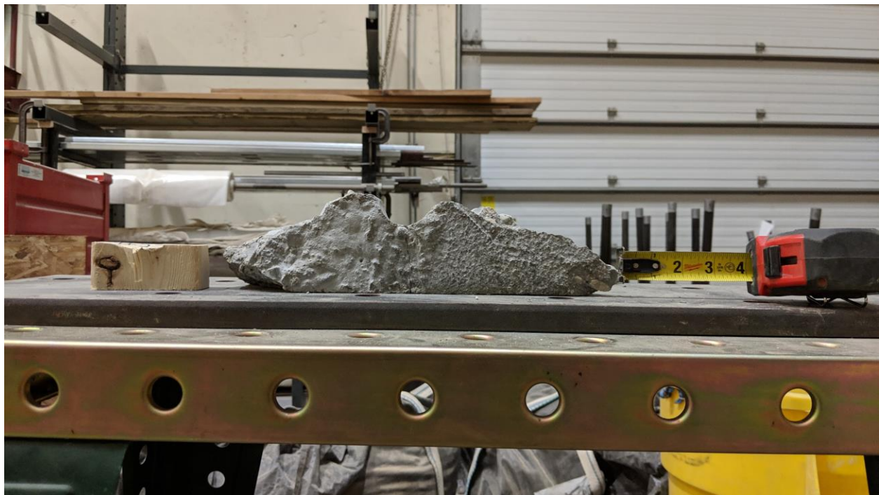
Figure A-82 – Front View of Test 23 Breakout Piece.
