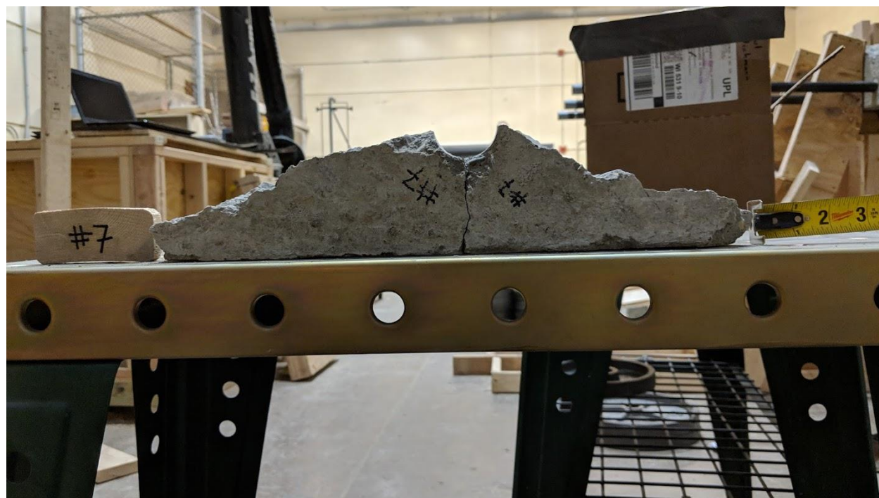
Figure A-32 – Front View of Test 9 Breakout Piece.
