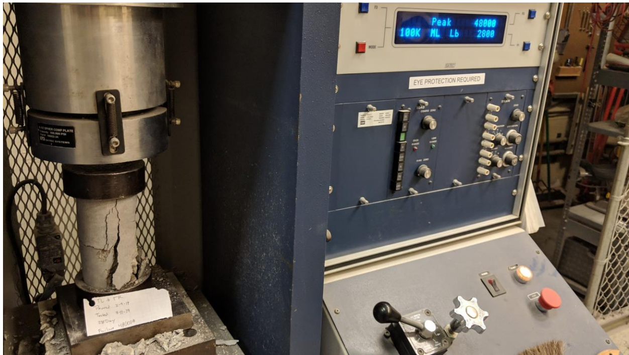
Figure B-25 - View 4 of Cylinder 2 of 30 Day Cylinder Break for Tests 1-10 and 21-30.
