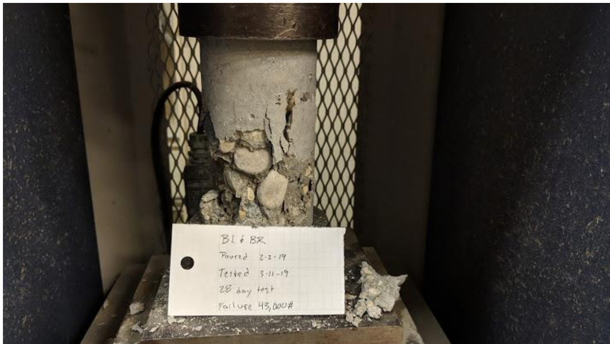
Figure B-8 – View 1 of Cylinder 1 of Cylinder Break for Tests 11-20 and 31-36.
