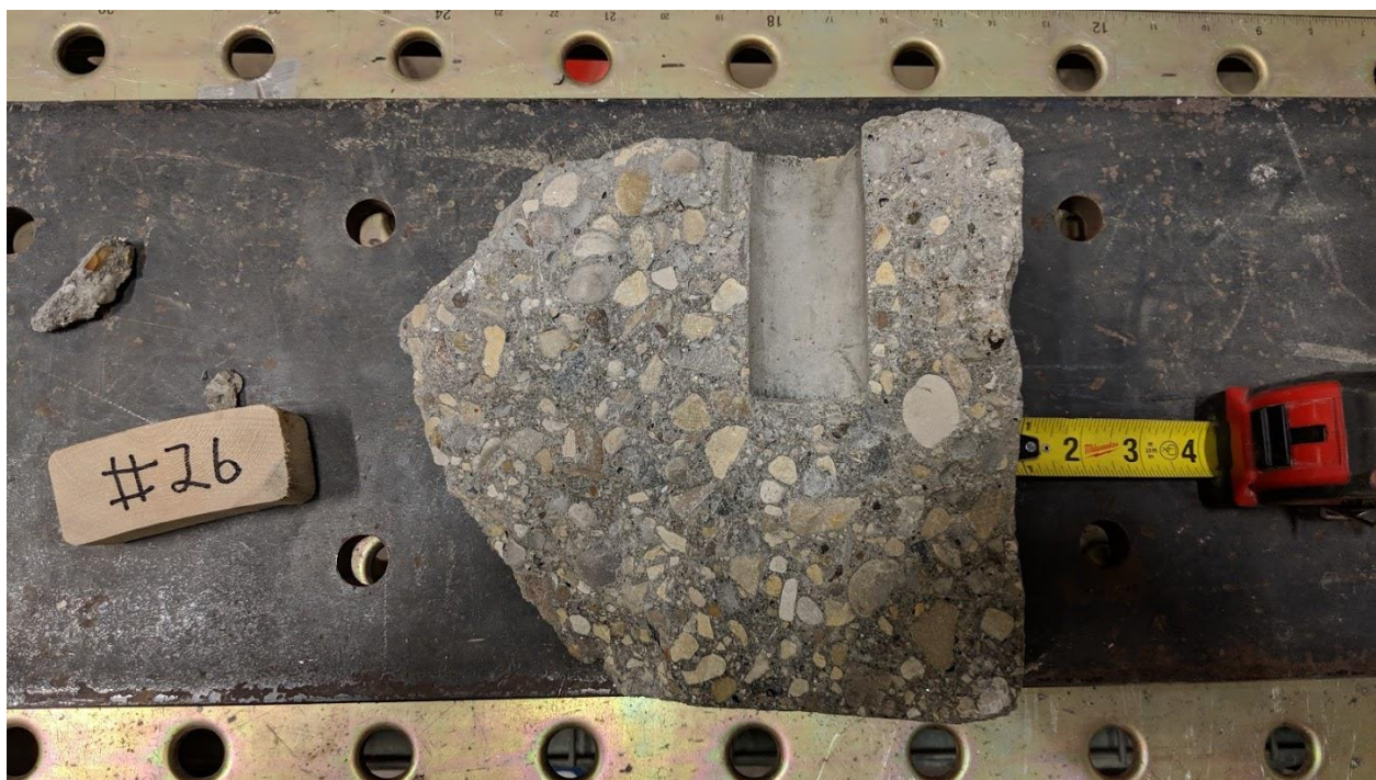
Figure A-98 – Top View of Test 26 Breakout Piece.
