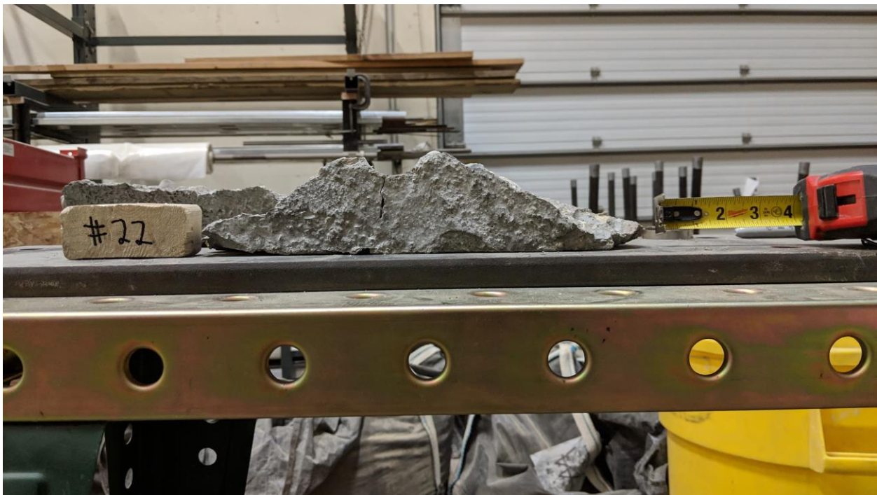
Figure A-78 – Front View 2 of Test 22 Breakout Piece.
