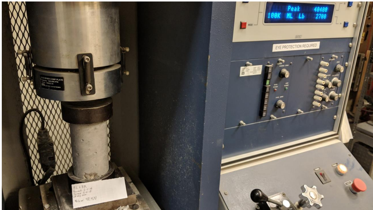
Figure B-13 - View 3 of Cylinder 2 of 37 Day Cylinder Break for Tests 11-20 and 31-36.
