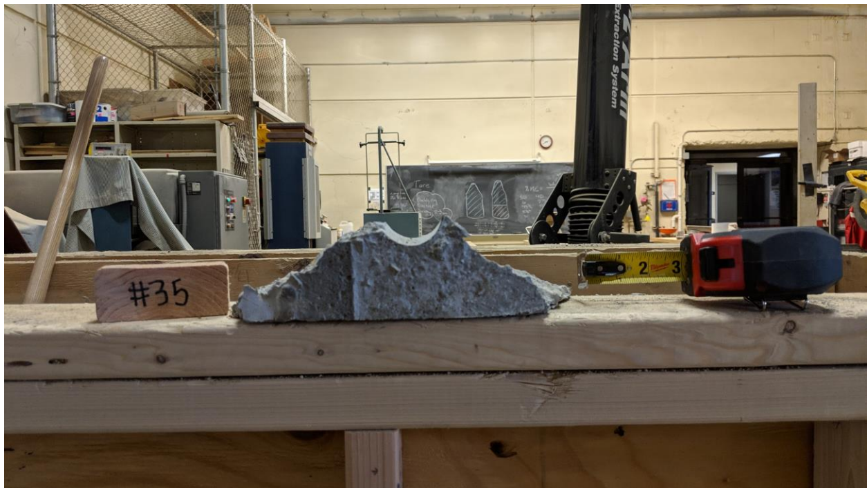
Figure A-124 – Front View of Test 35 Breakout Piece.
