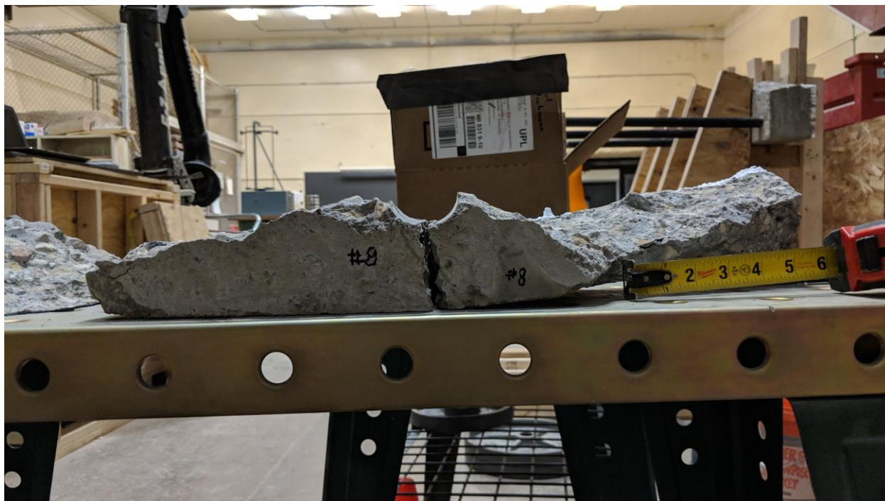
Figure A-27 – Front View 1 of Test 8 Breakout Piece.
