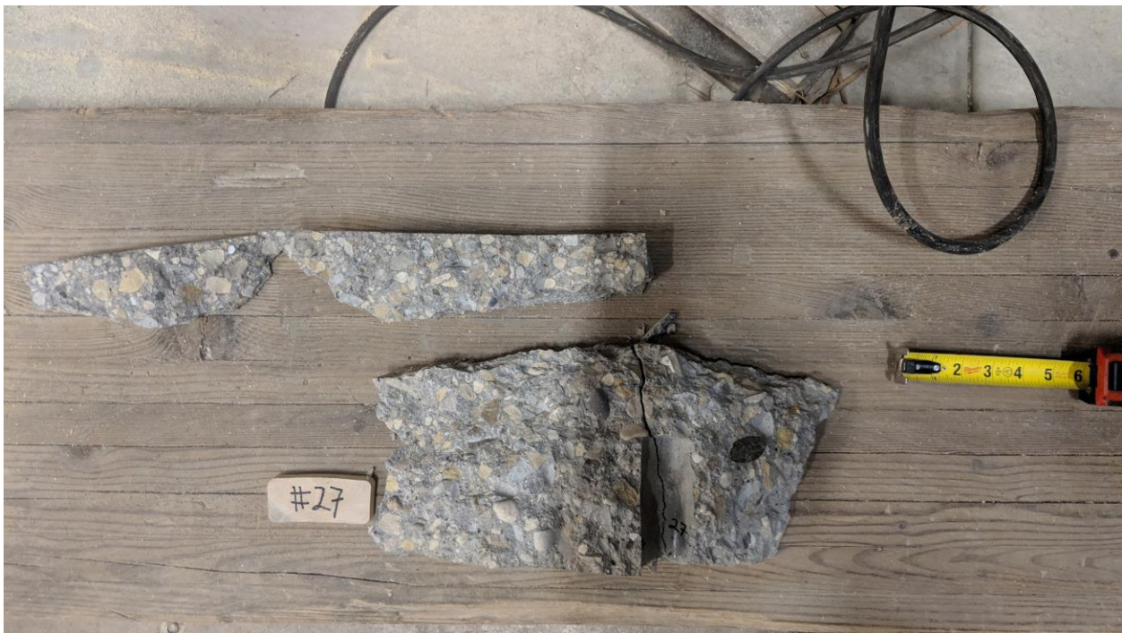
Figure A-106 – Top View of Test 27 Breakout Piece.
