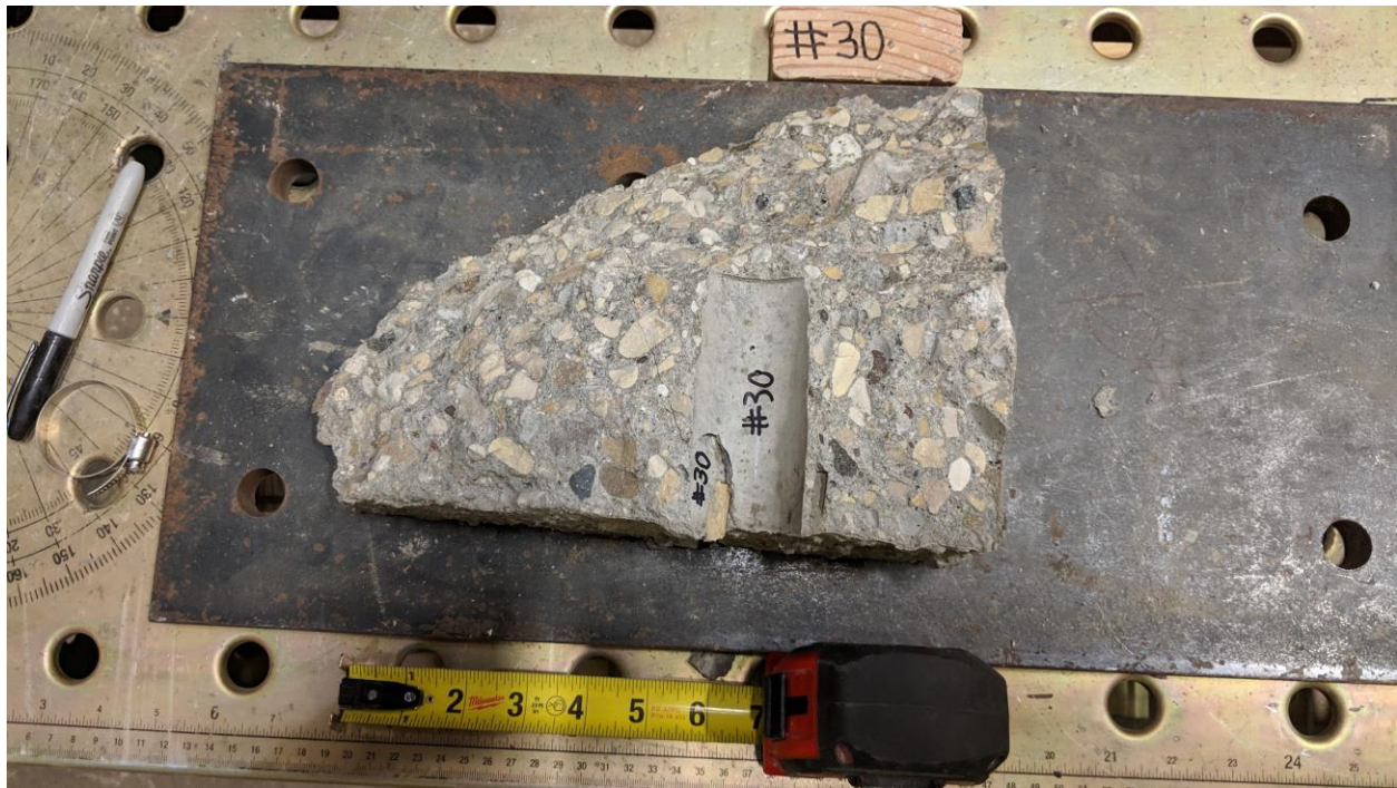
Figure A-113 – Top View of Test 30 Breakout Piece.
