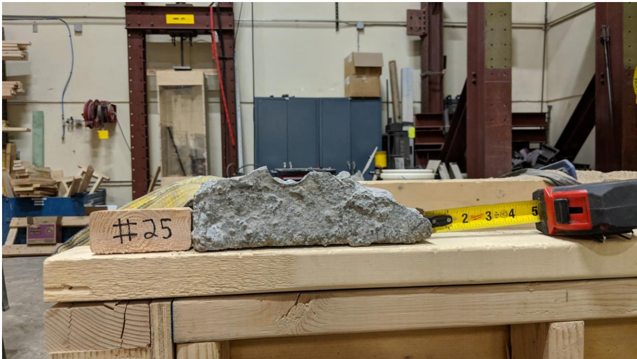
Figure A-92 – Front View of Test 25 Breakout Piece.
