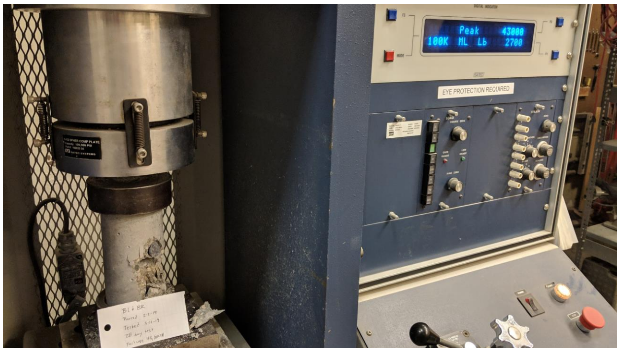
Figure B-10 - View 3 of Cylinder 1 of 37 Day Cylinder Break for Tests 11-20 and 31-36.
