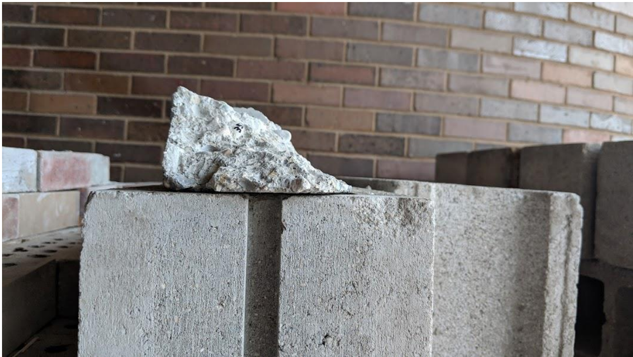
Figure A-126 – Side View 1 of Test 35 Breakout Piece.
