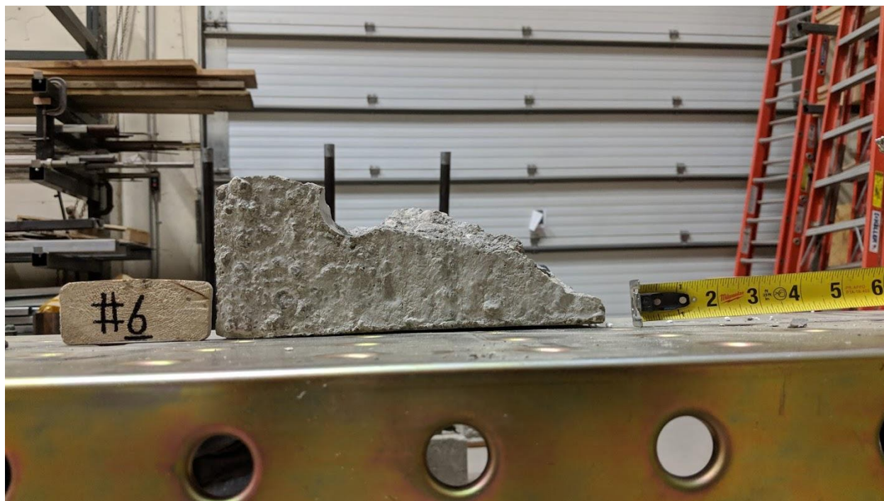
Figure A-17 – Front View of Test 6 Breakout Piece.
