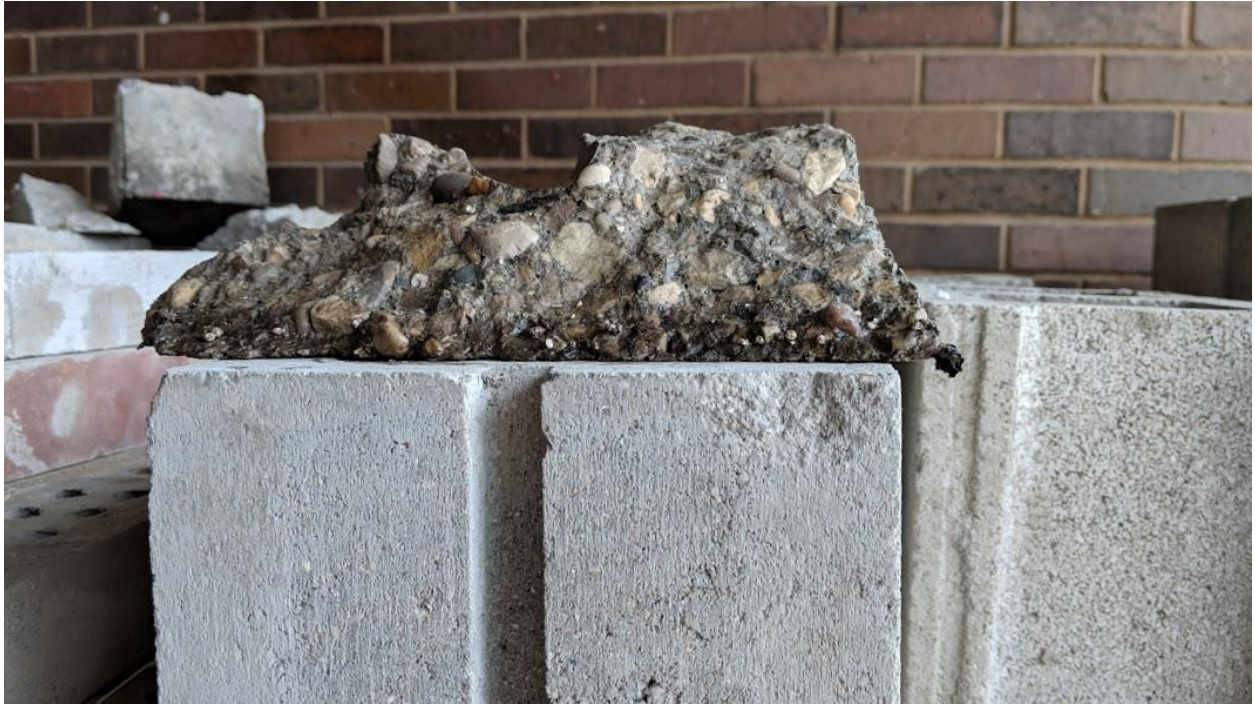
Figure A-121 – Back View of Test 34 Breakout Piece.
