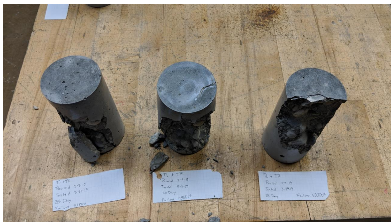
Figure B-32 - View 2 of All 30 Day Cylinder Breaks for Tests 1-10 and 21-30.
