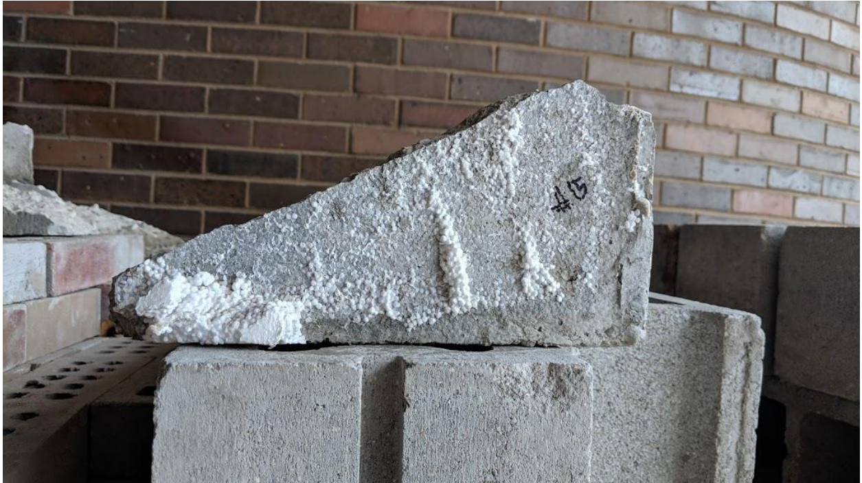
Figure A-57 – Back View of Test 15 Breakout Piece.
