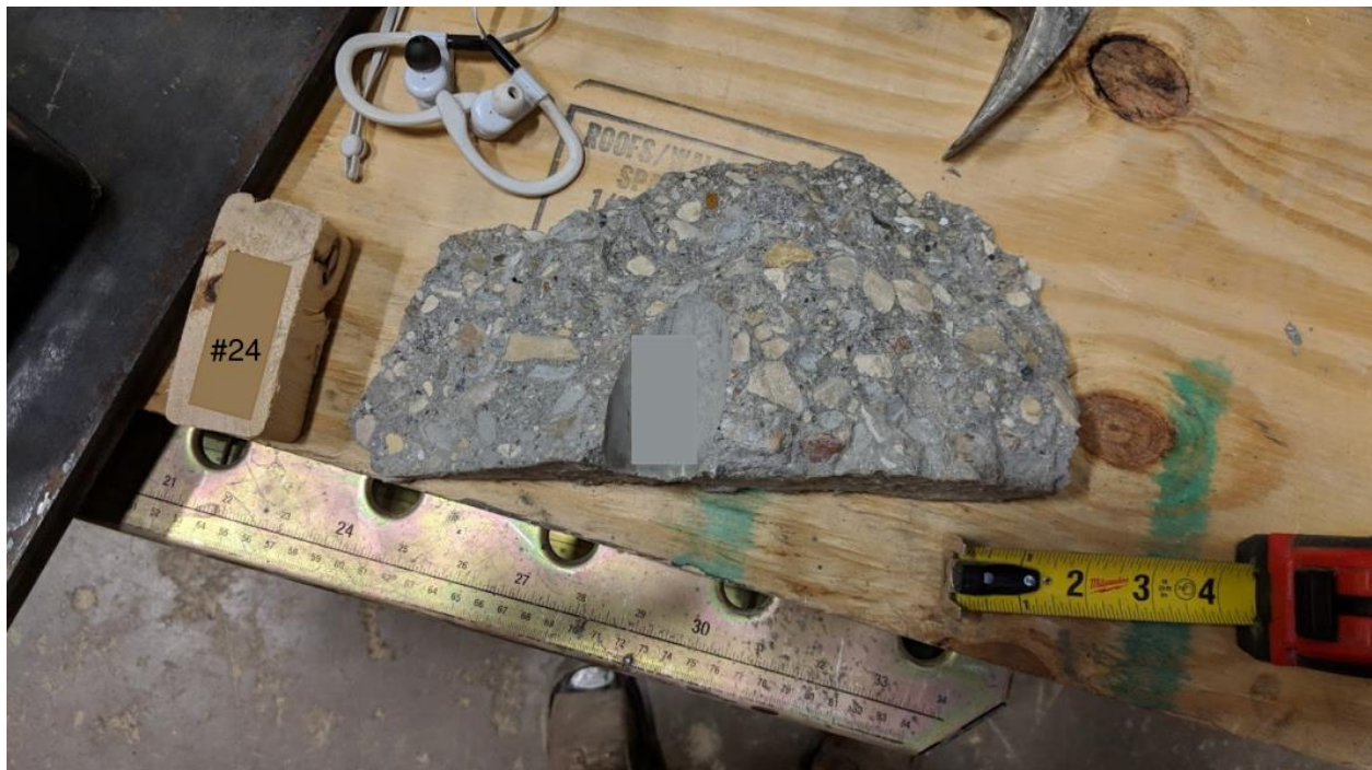
Figure A-88 – Top View of Test 24 Breakout Piece.
