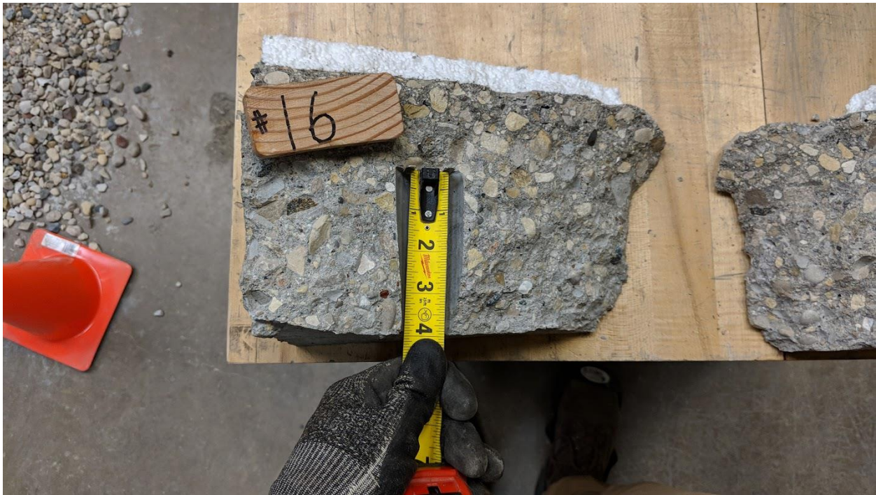
Figure A-64 – Top View of Test 16 Breakout Piece.
