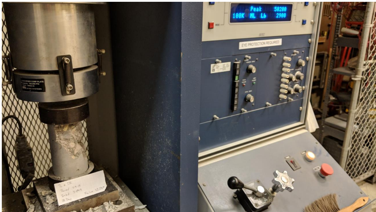
Figure B-28 - View 3 of Cylinder 3 of 30 Day Cylinder Break for Tests 1-10 and 21-30.
