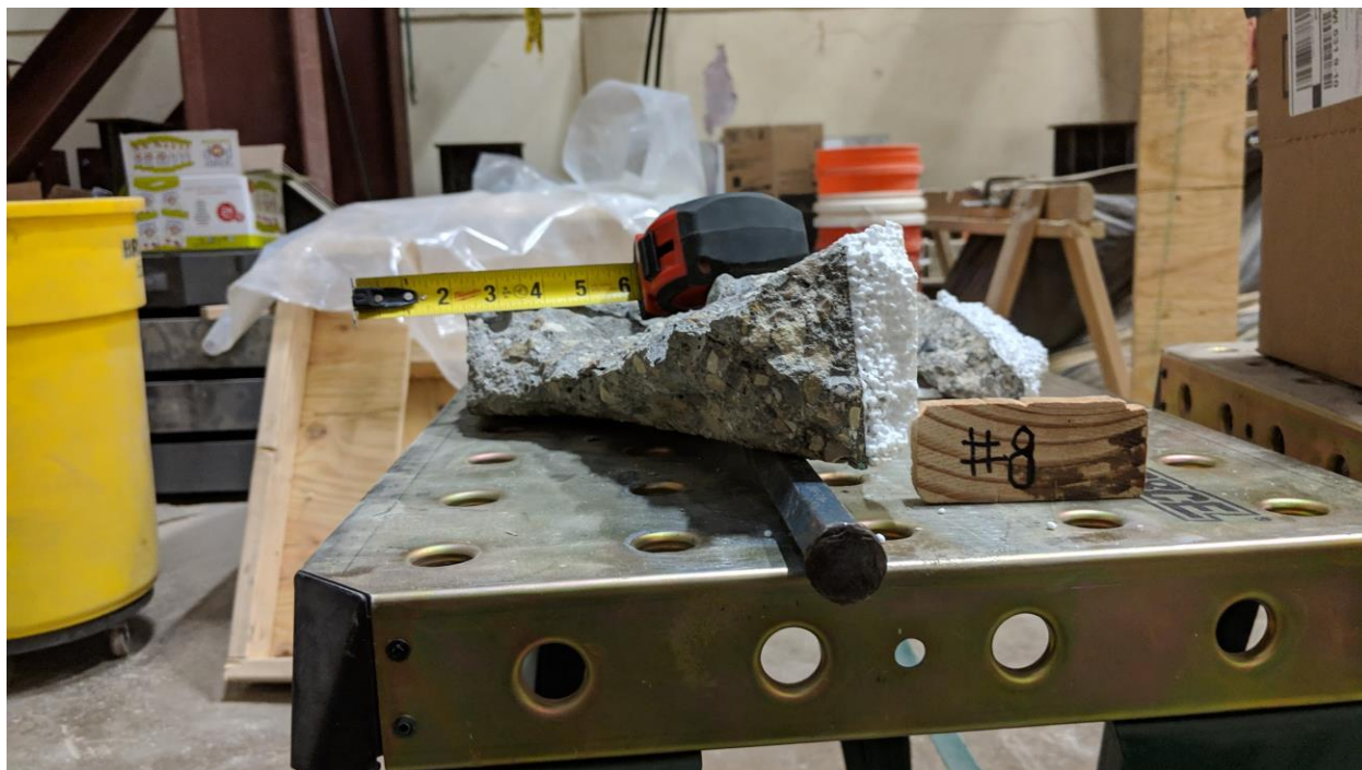
Figure A-29 – Side View of Test 8 Breakout Piece.
