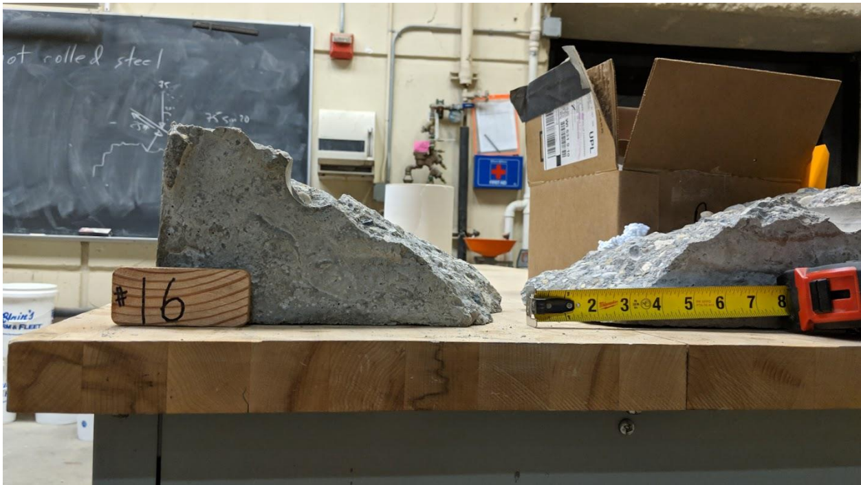
Figure A-62 – Front View of Test 16 Breakout Piece.
