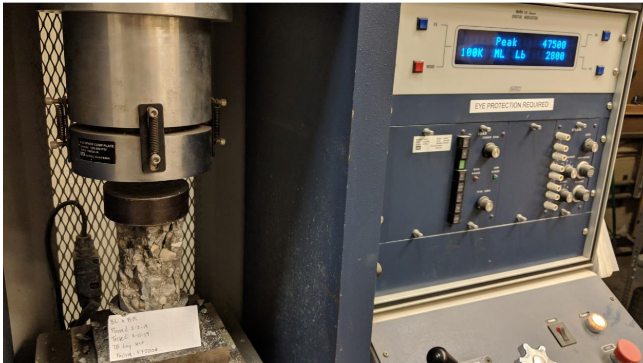
Figure B-17 - View 4 of Cylinder 3 of 37 Day Cylinder Break for Tests 11-20 and 31-36.
