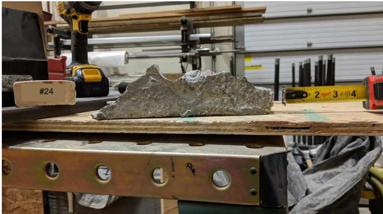
Figure A-87 – Front View of Test 24 Breakout Piece.
