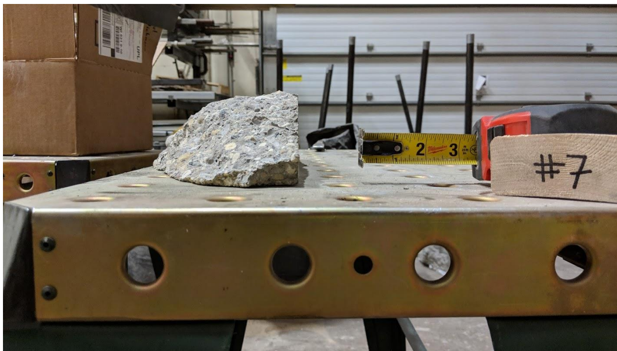
Figure A-33 – Side View 1 of Test 9 Breakout Piece.
