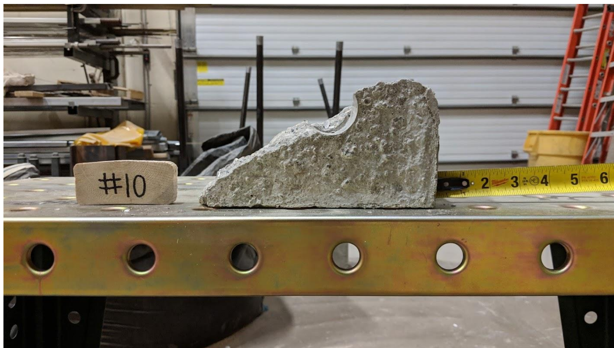
Figure A-37 – Front View of Test 10 Breakout Piece.
