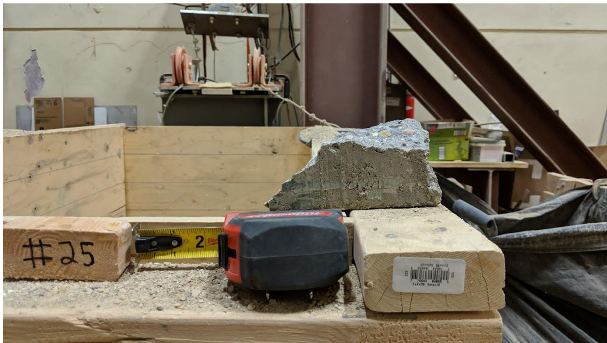
Figure A-94 – Side View of Test 25 Breakout Piece.
