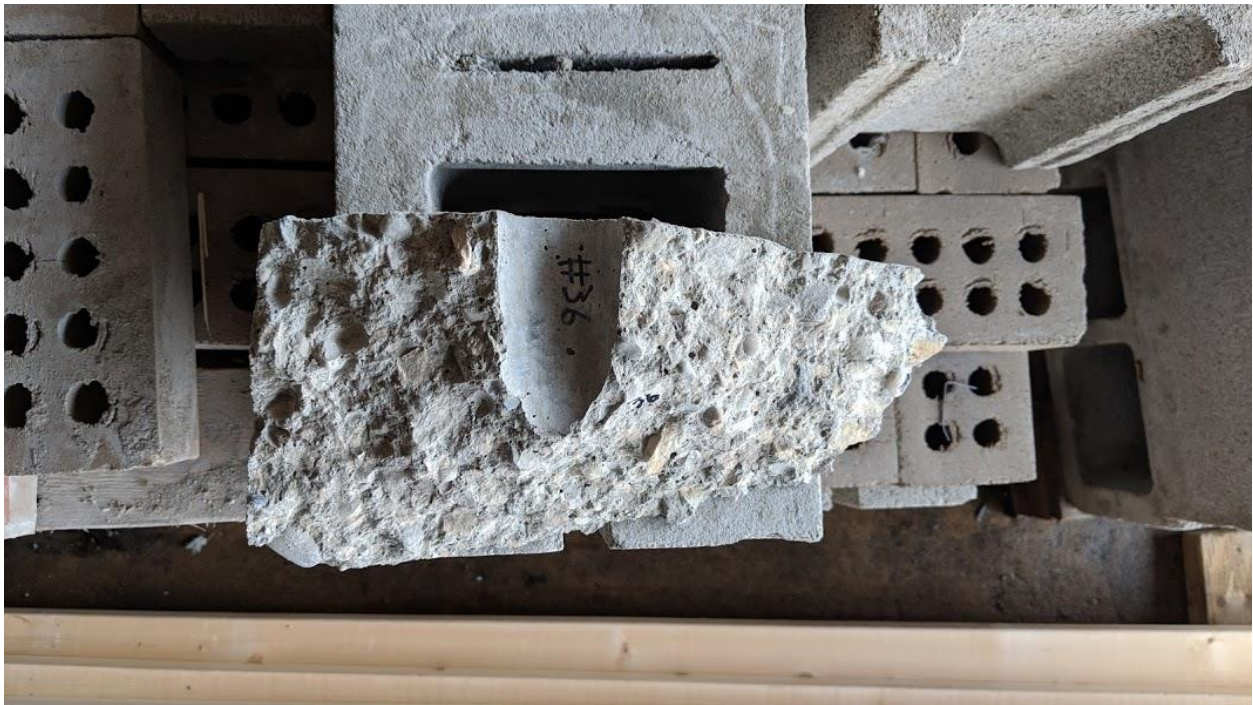
Figure A-134 – Top View of Test 36 Breakout Piece.
