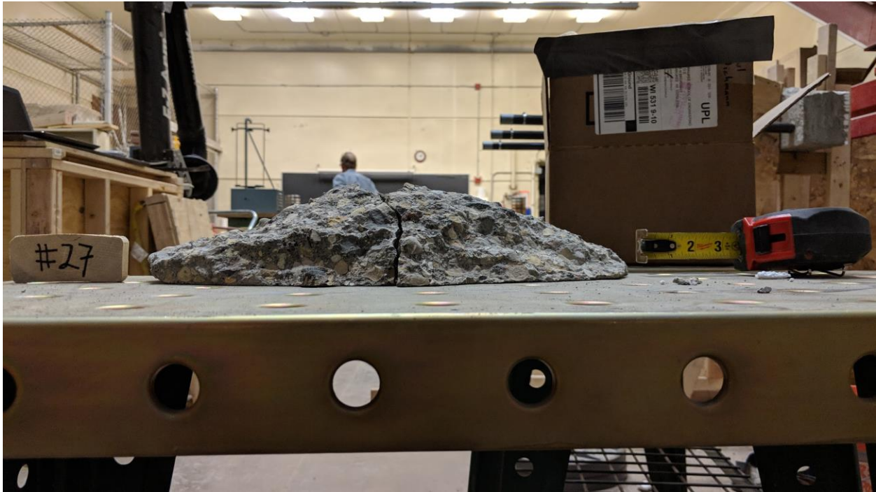
Figure A-103 – Back View of Test 27 Breakout Piece.
