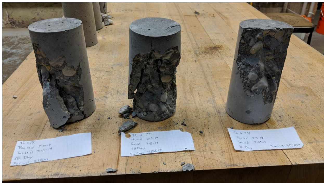
Figure B-31 - View 1 of All 30 Day Cylinder Breaks for Tests 1-10 and 21-30.
