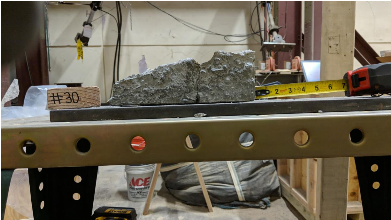
Figure A-110 – Front View of Test 30 Breakout Piece.
