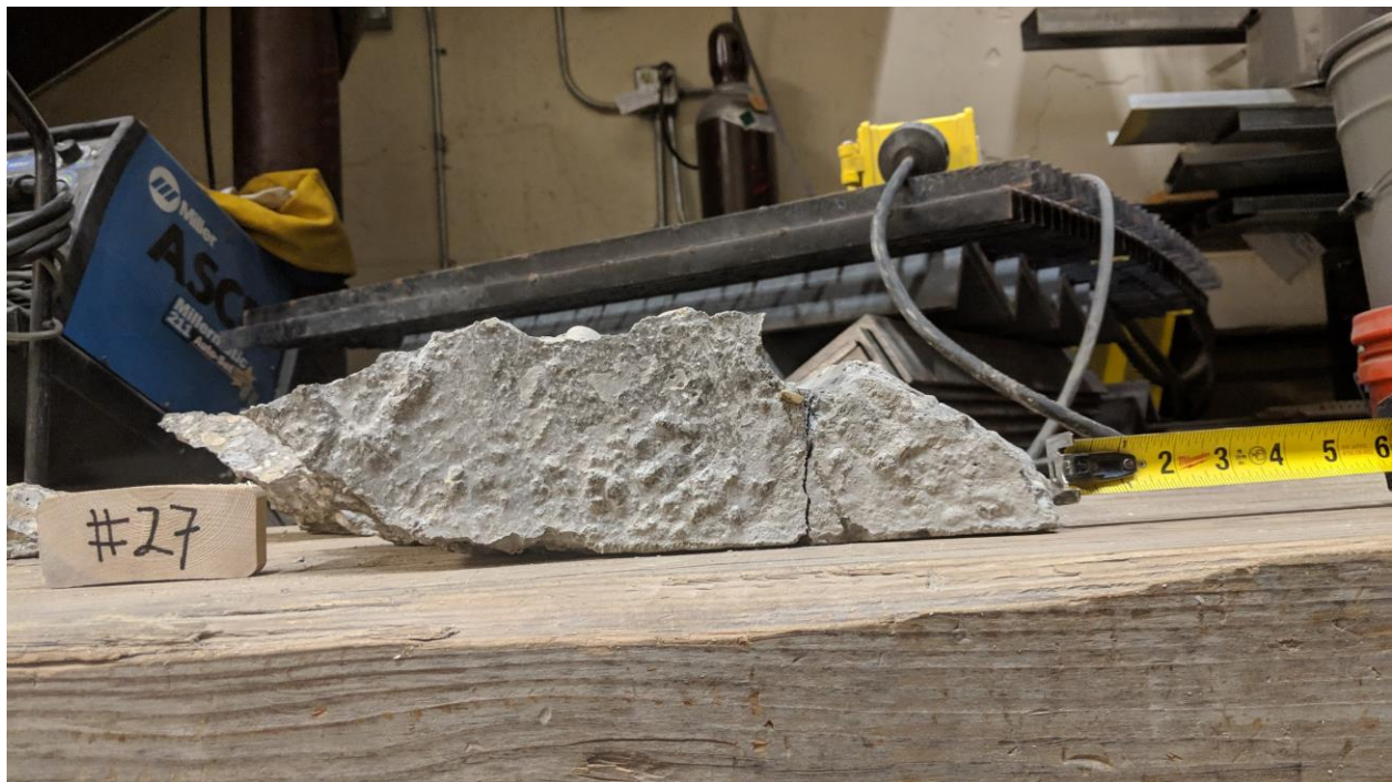
Figure A-102 – Front View of Test 27 Breakout Piece.
