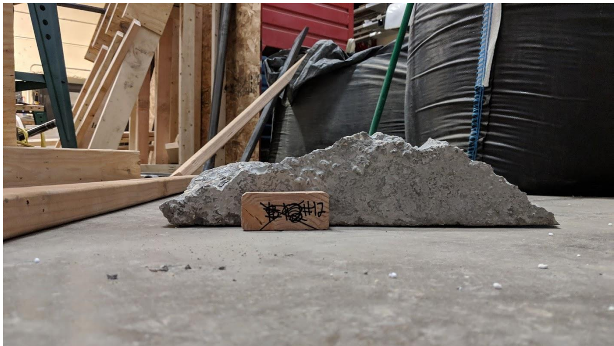
Figure A-48 – Front View of Test 12 Breakout Piece.
