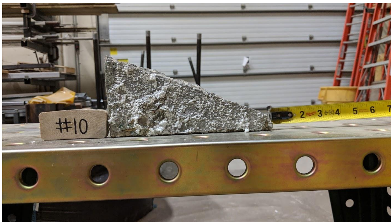
Figure A-38 – Back View of Test 10 Breakout Piece.
