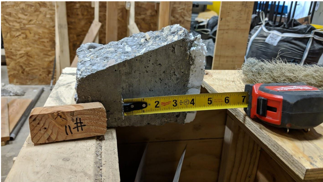
Figure A-46 – Side View of Test 11 Breakout Piece.
