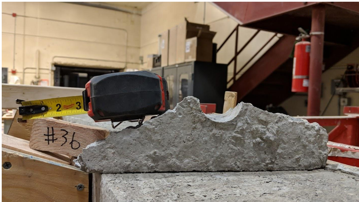
Figure A-130 – Front View of Test 36 Breakout Piece.
