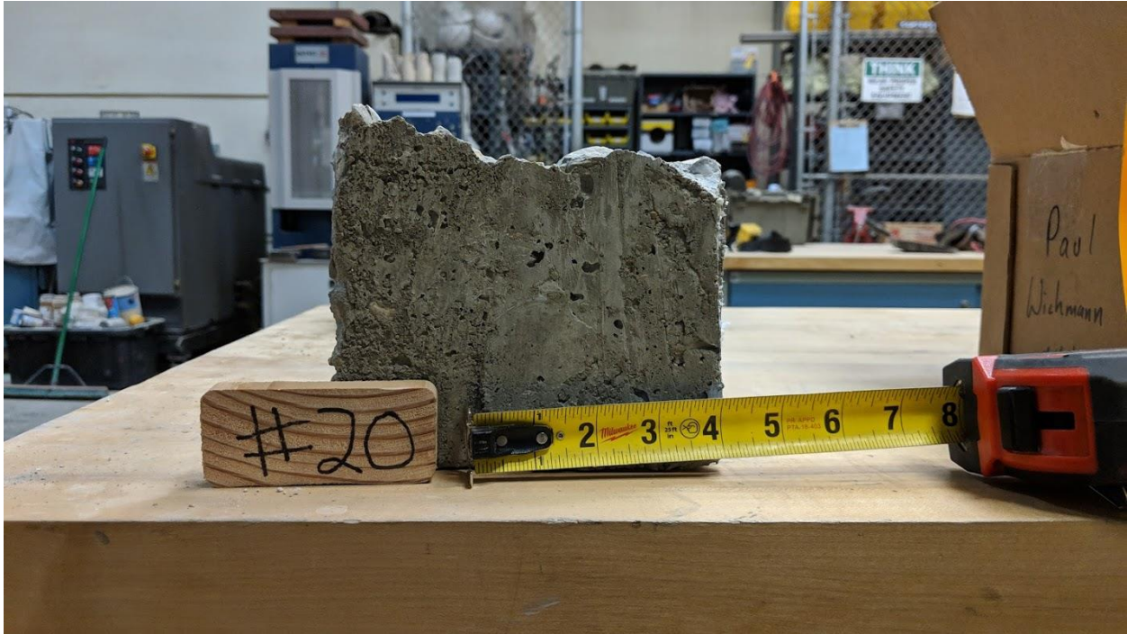
Figure A-73 – Side View of Test 20 Breakout Piece.
