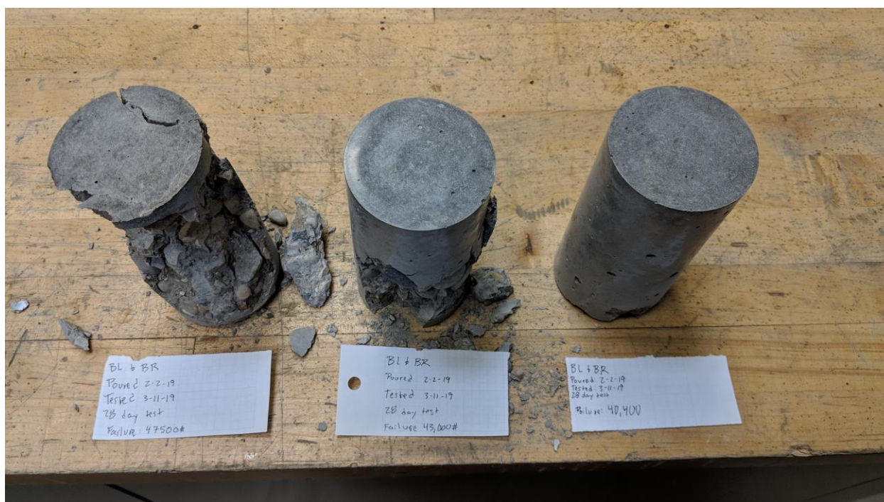
Figure B-30 - View 2 of All 37 Day Cylinder Breaks for Tests 11-20 and 31-36.
