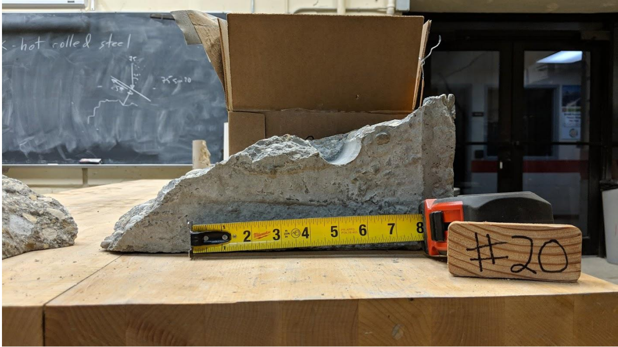
Figure A-71 – Front View of Test 20 Breakout Piece.
