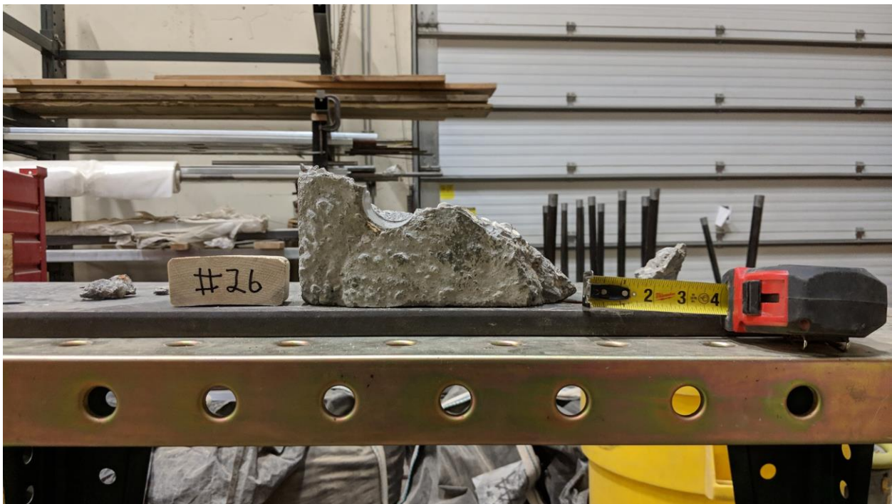
Figure A-96 – Front View of Test 26 Breakout Piece.
