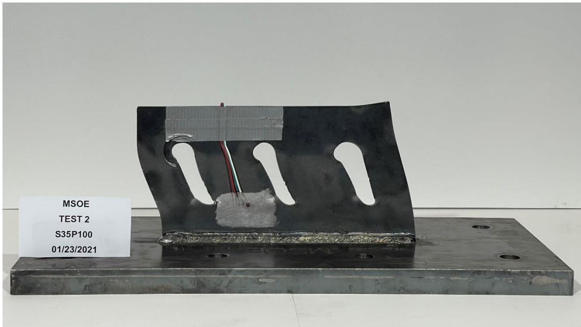
Figure G-3: Specimen S35P100 Post-Test, Front.
