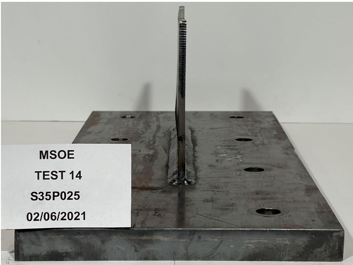
Figure G-30: Specimen S35P025 Post-Test, Loaded Edge.
