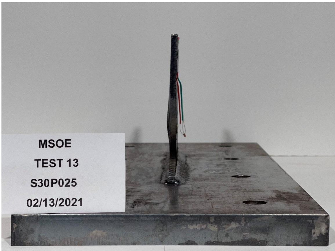
Figure G-28: Specimen S30P025 Post-Test, Loaded Edge.
