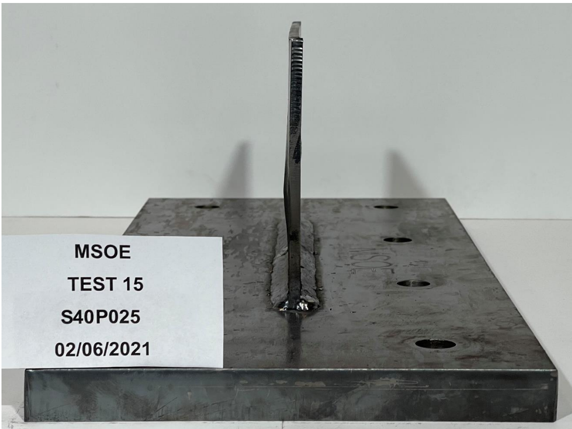
Figure G-32: Specimen S40P025 Post-Test, Loaded Edge.
