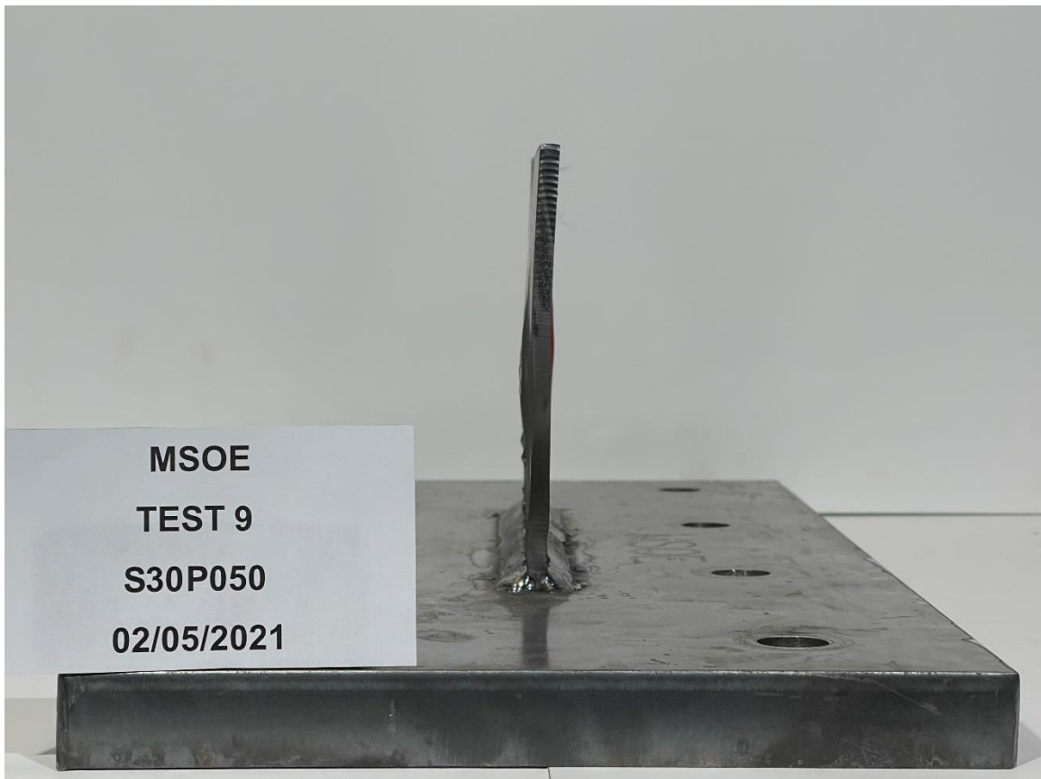
Figure G-19: Specimen S30P050 Post-Test, Loaded Edge.
