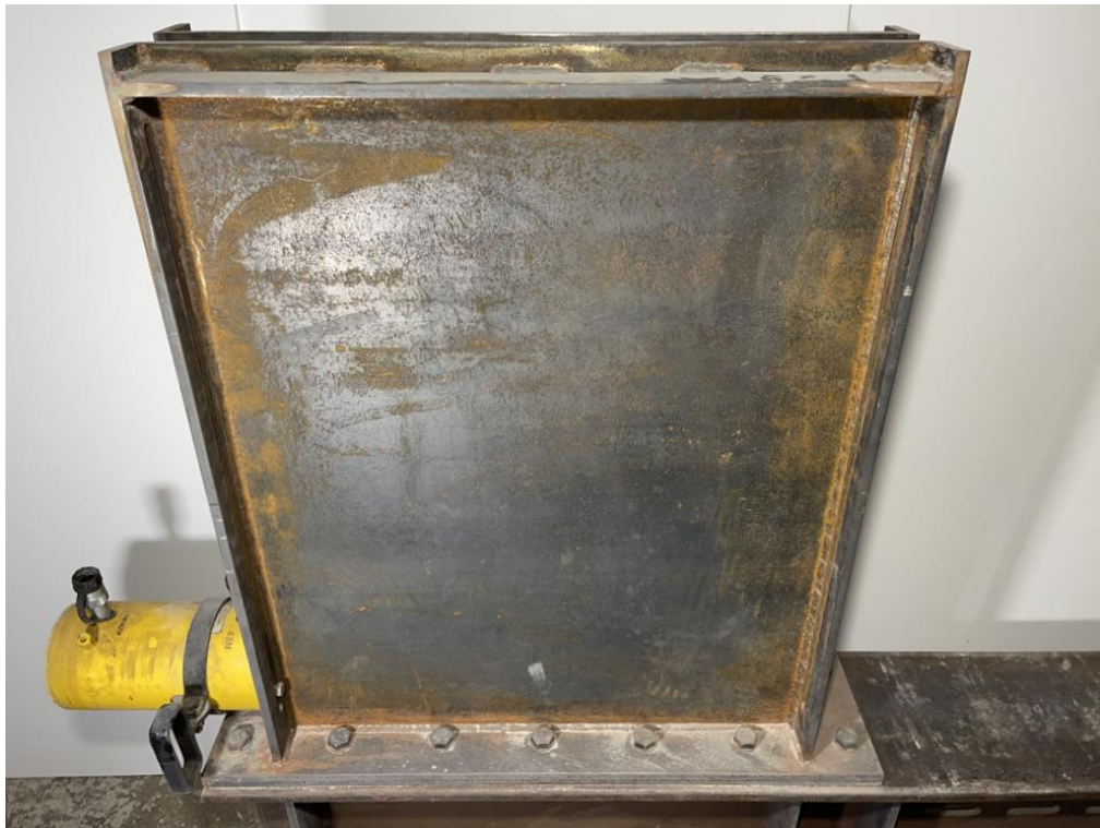
Figure 3.5-3: Reaction Plates in Test Setup.
