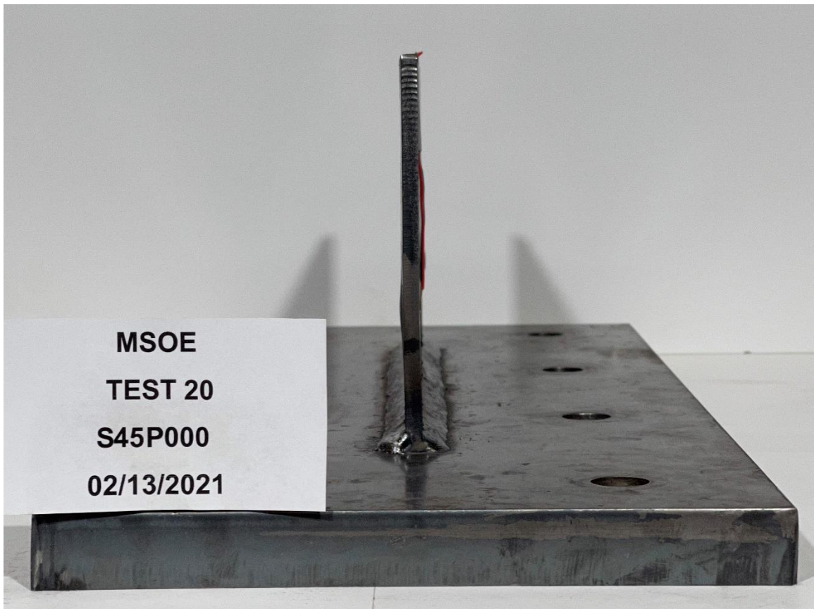
Figure G-42: Specimen S45P000 Post-Test, Loaded Edge.
