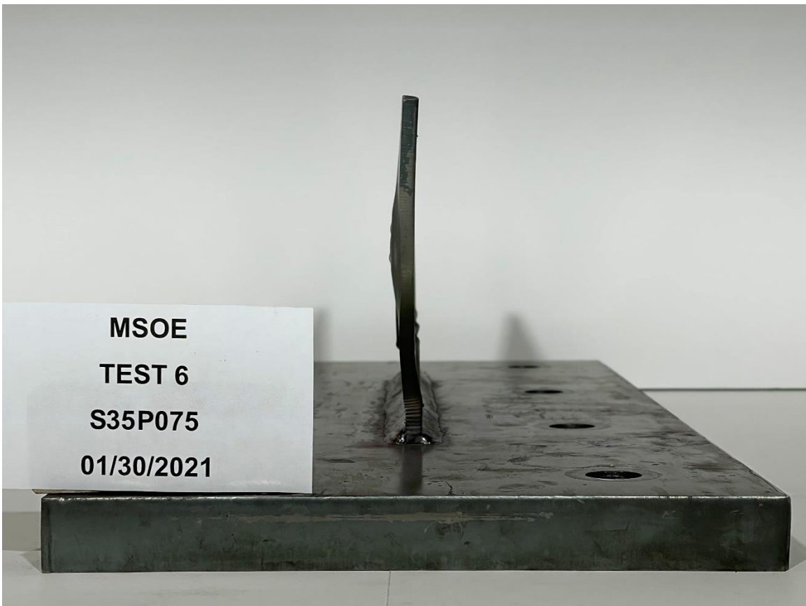
Figure G-12: Specimen S35P075 Post-Test, Loaded Edge.
