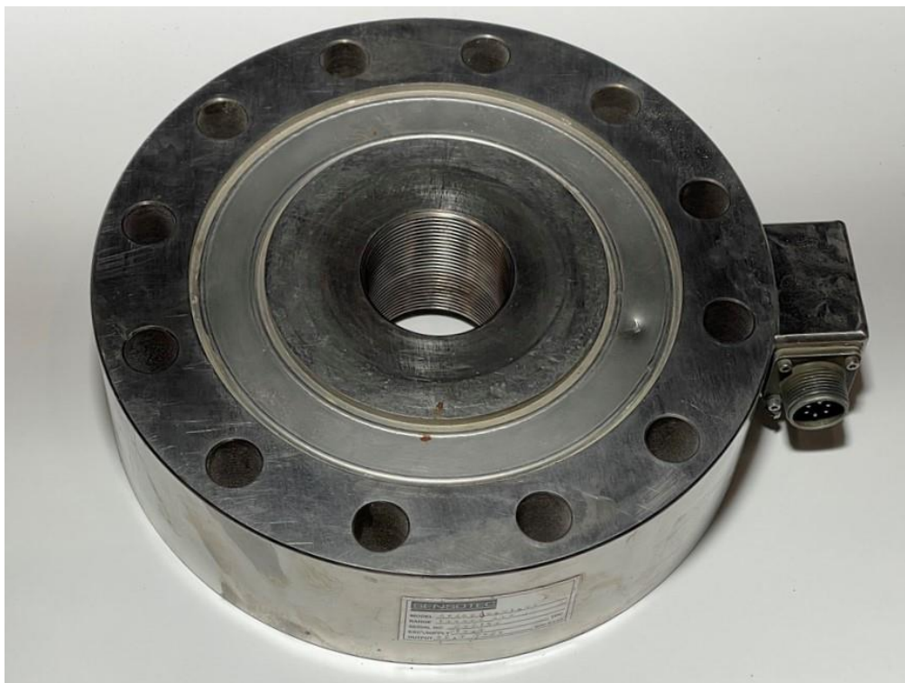
Figure 3.5-5: Sensotec 41-A530-01-03 Load Cell.
