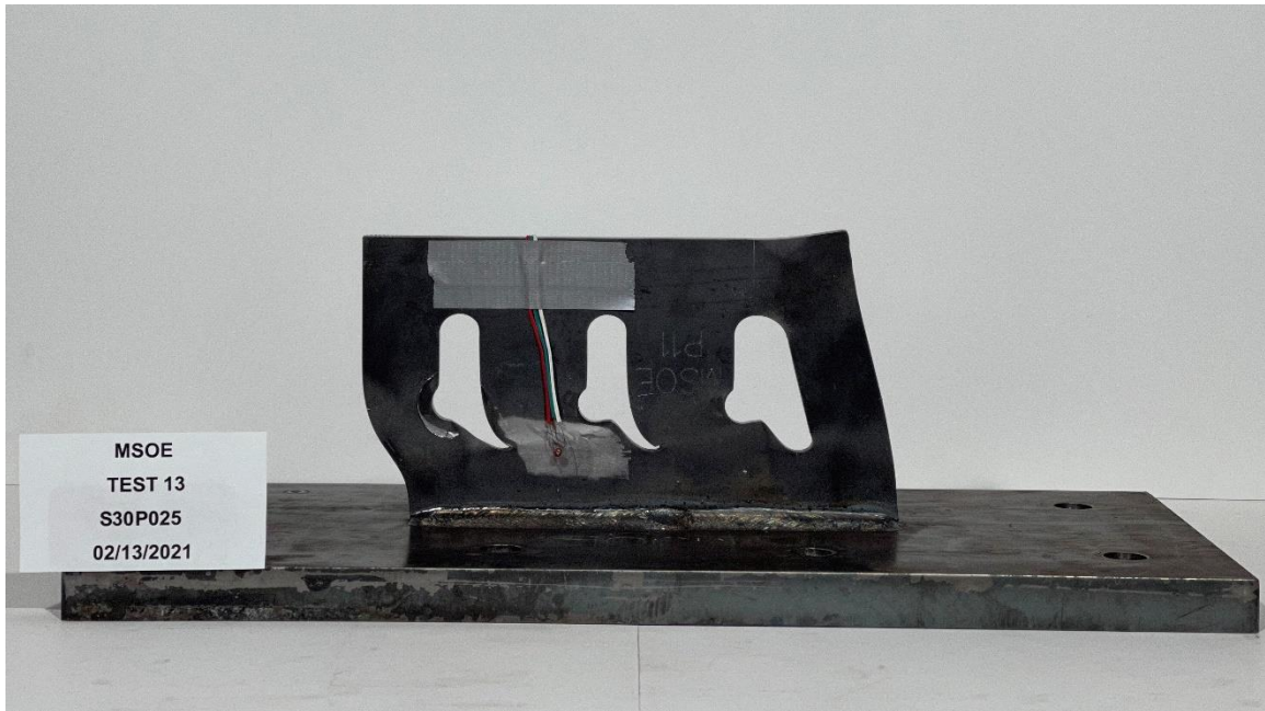
Figure G-27: Specimen S30P025 Post-Test, Front.
