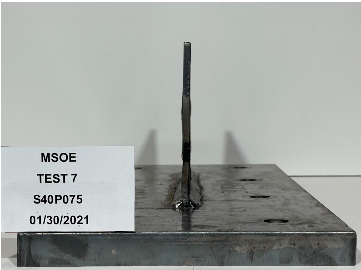
Figure G-15: Specimen S40P075 Post-Test, Loaded Edge.
