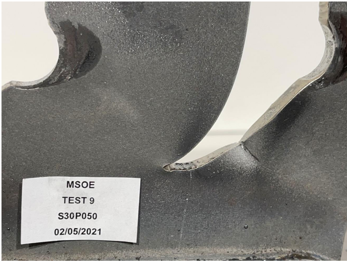
Figure G-20: Specimen S30P050 Post-Test, Plate Tearing.
