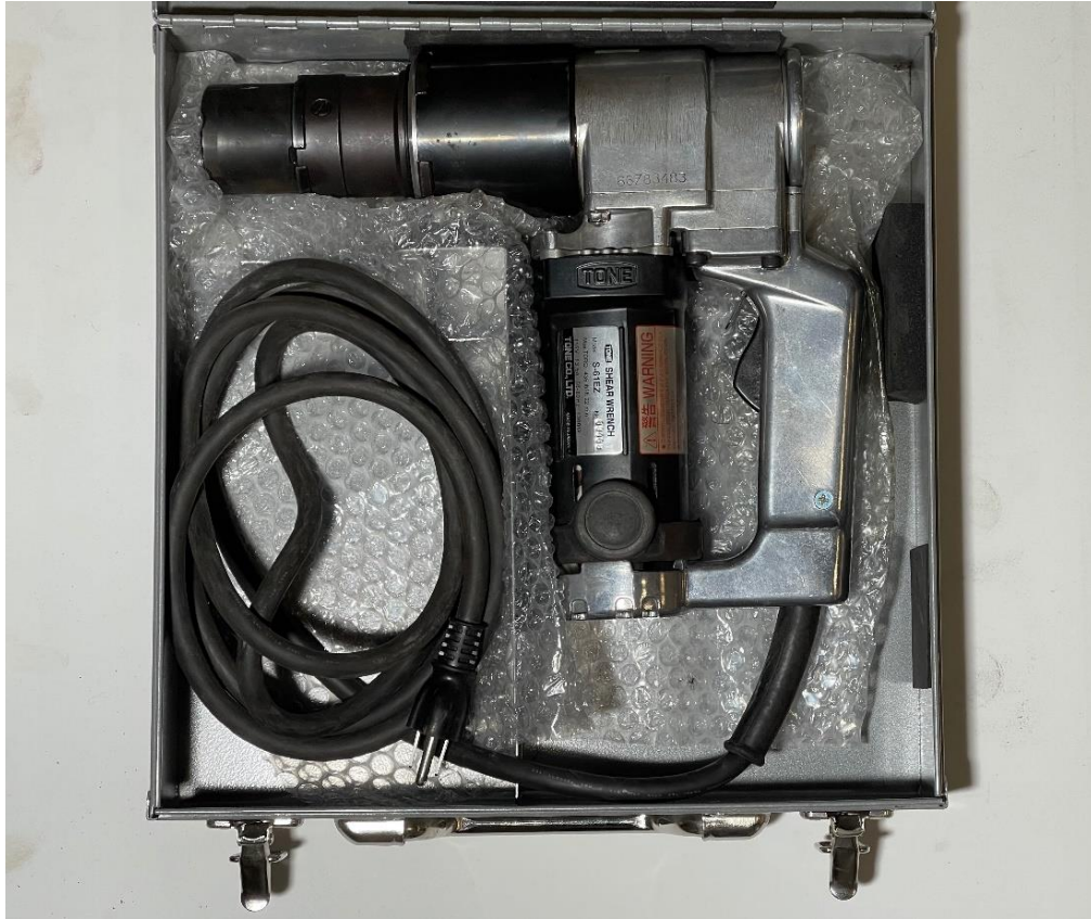
Figure 3.10-2: TONE® Shear Wrench.
