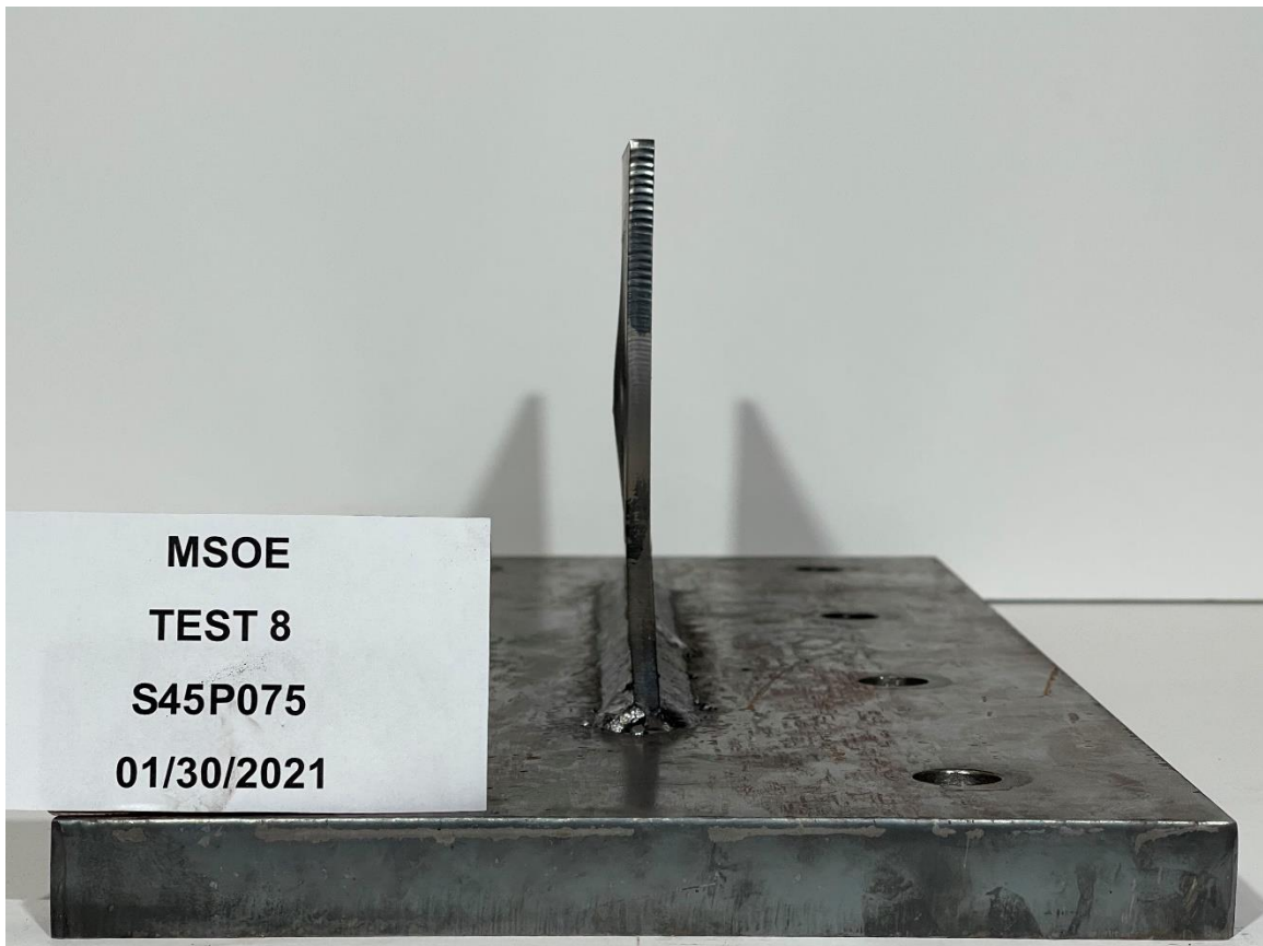
Figure G-17: Specimen S45P075 Post-Test, Loaded Edge.
