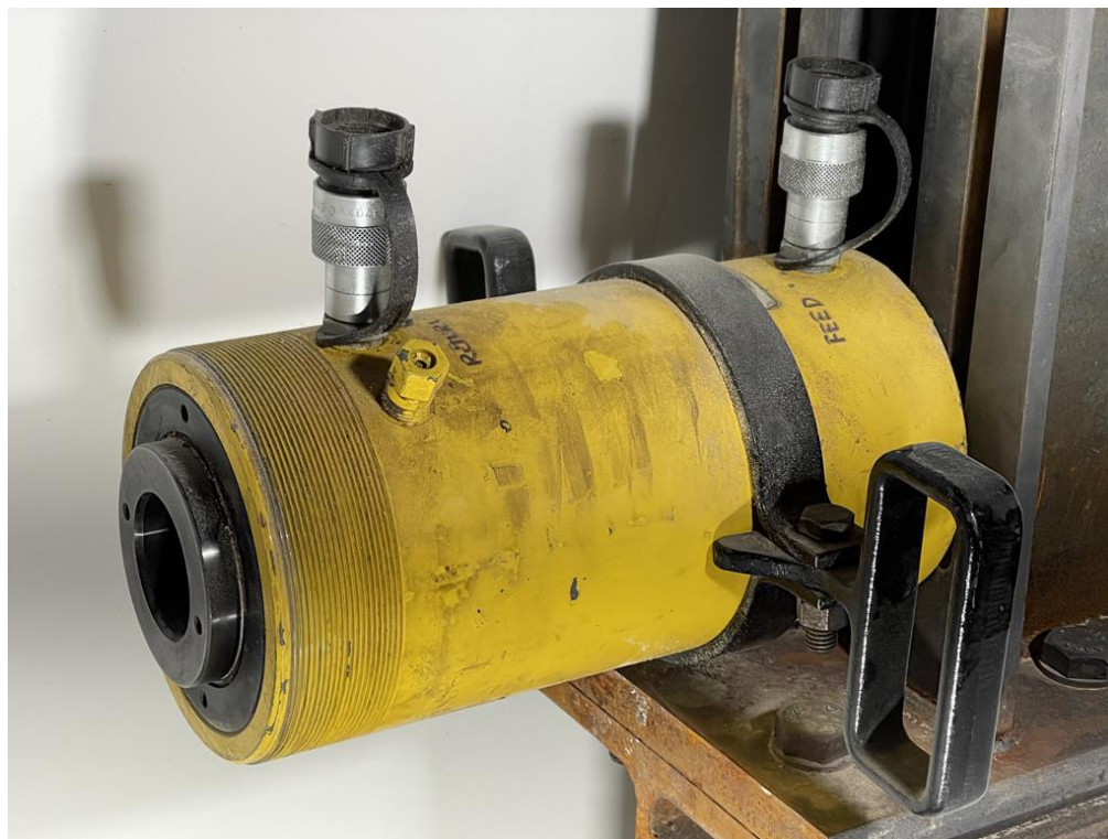
Figure 3.5-4: Enerpac RRH606 “Hollow-Core” Actuator.
