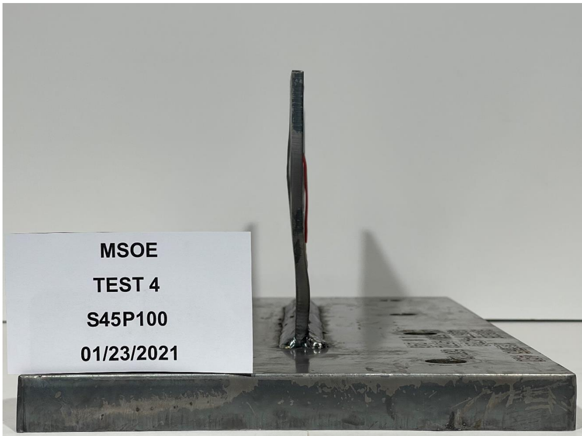
Figure G-8: Specimen S45P100 Post-Test, Loaded Edge.
