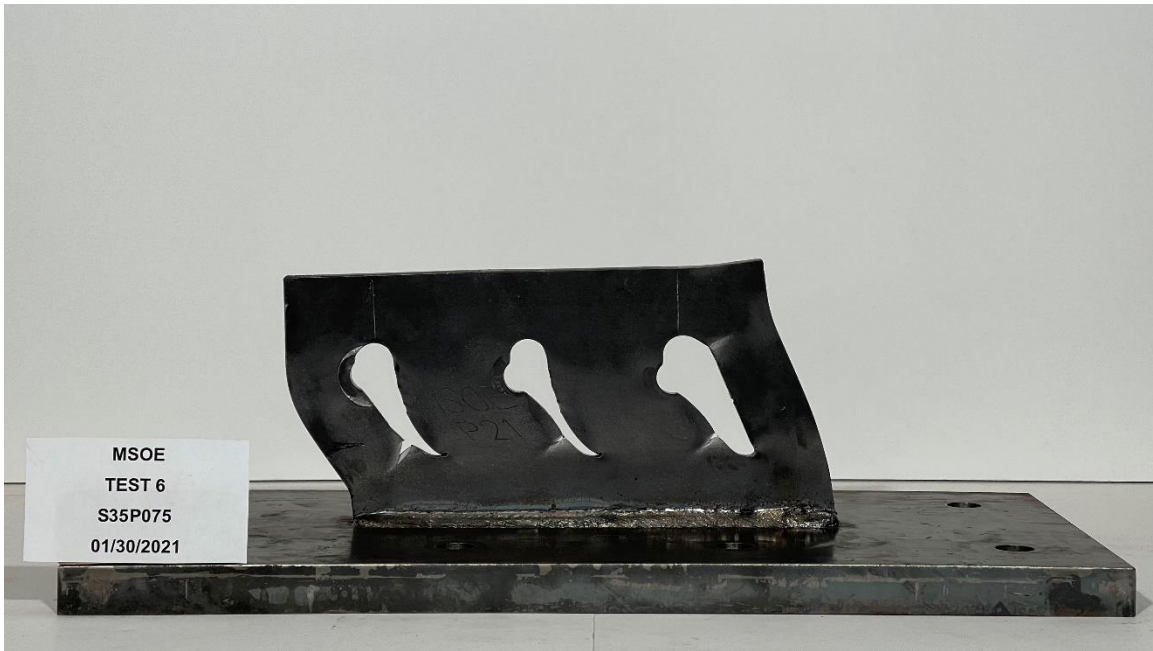
Figure G-11: Specimen S35P075 Post-Test, Front.
