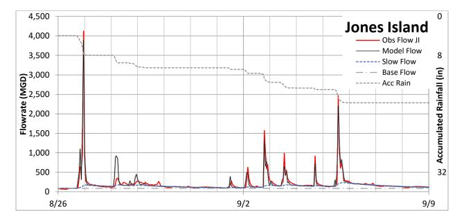
*Note.* Figure 6 shows a two-week representation of the model. The Slow Flow is the Slow Response, representing infiltration in the sewer system. This system is affected most by inflow to the system during rain events. With the Base Flow, or typical flow from daily use, the Slow Flow is shown to have a lasting effect on the system of about three days. The Model Flow Peaks are well defined and match the observed flow well, though the peaks fall short.
