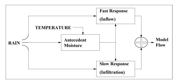
Note. Adapted from "The Application of System Identification to Inflow and Infiltration Modeling and Design Storm Event Simulation for Sanitary Collection Systems," by T. Van Pelt and R. Czachorski, 2002, WEFTEC 2002 Conference Proceedings, Proceedings of the Water Environment Federation, p. 611. The diagram shows how the inputs of the model (RAIN, TEMPERATURE) alter the antecedent moisture, which adjusts the response flow.
