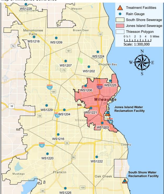
Note. Areas of Milwaukee that are serviced by the Milwaukee Metropolitan Sewerage District. The county is split into areas measured by MMSD rain gauge stations and the different sewerages. Map created by author using ArcGIS Pro with available data from MMSD.
