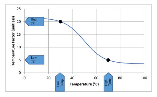
*Note.* Adapted from R. Czachorski (personal communication, 2020). The figure shows a sigmoid curve, which represents the Temperature Factor that corresponds to the timestep's temperature. This example has a set factor of 20 for 30°C and 10 for 70°C. As temperature increases, the temperature factor decreases.
