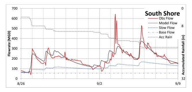
*Note.* Figure 8 shows a two-week representation of the model. The Slow Flow is the Slow Response, representing infiltration in the sewer system. This system is affected most by infiltration after a rain event. With the Base Flow graphed the Slow Flow is shown to have a lasting effect on the system. The Model Flow Peaks are less defined, and the peaks are missed by a significant amount.
