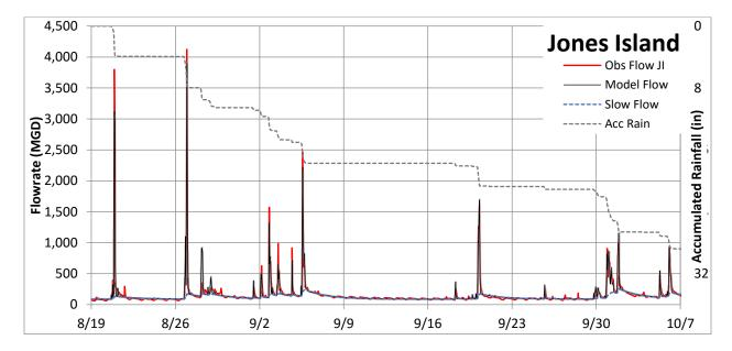
*Note.* Figure 5 shows the total model for Jones Island compared to the observed flow for the combined sewer system. The Fast Flow is the difference of the Slow Flow from the Model Flow. The Slow Flow is the Slow Response, representing infiltration in the sewer system. This system is affected most by inflow to the system during rain events.
