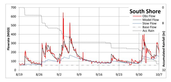
*Note.* Figure 7 shows the total model for South Shore compared to the observed flow for the separate sewer system. The flowrate to South Shore is significantly less than Jones Island.
