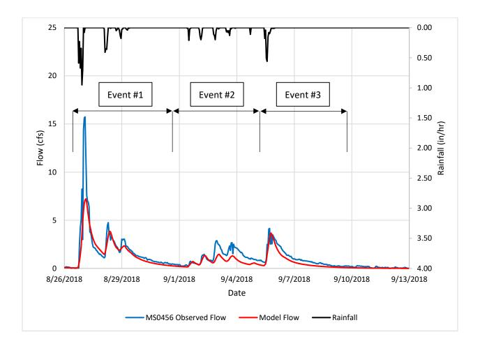
Note. The model substantially underpredicted the peak flow and slightly underpredicted the volume of Event #1 and #2. Peak flow of Event #3 was predicted accurately by the model.
