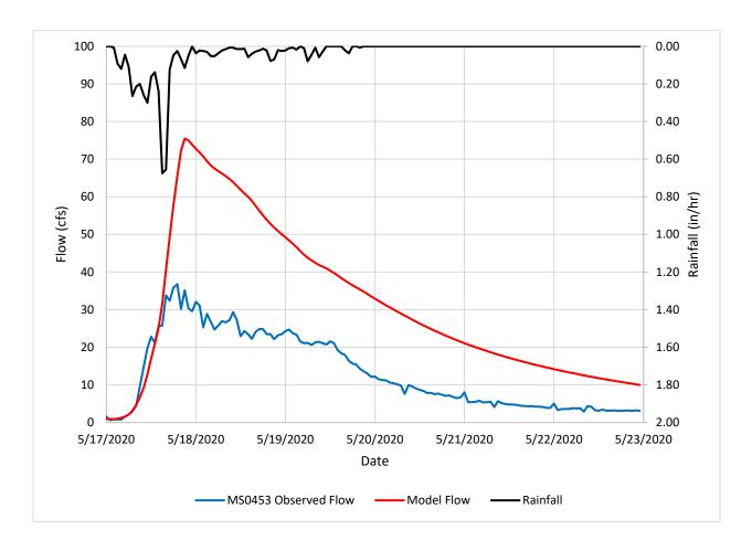
*Note.* The model substantially overpredicted the event in peak flow as well as volume.
