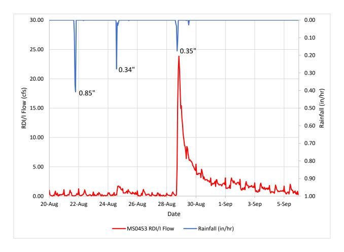
*Note*. Figure 10 shows the RDI/I flow experienced by sewer MS0453 as well as three rainfall events that occurred over its catchment area. The cumulative rainfall depths for each event are listed next to each event's peak rainfall intensity. Though the first event has a cumulative depth more than twice the depth of the third event, the third event was the only event to exhibit an RDI/I response in sewer MS0453.
