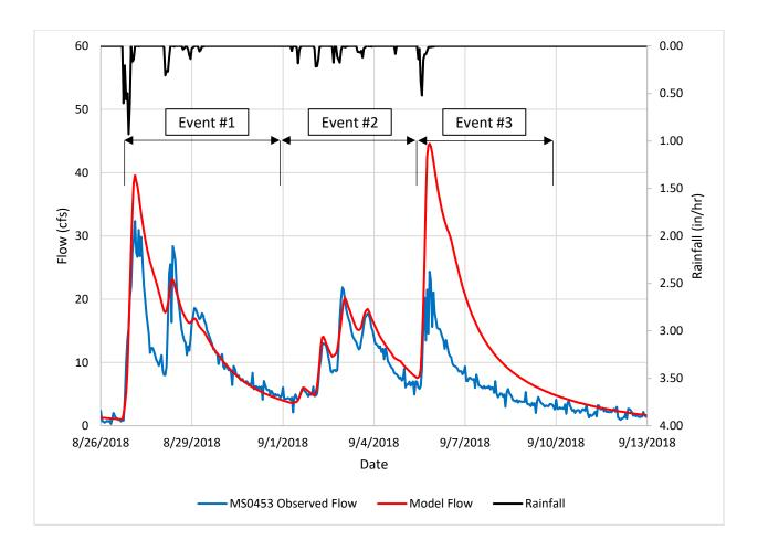
Note. The model slightly overpredicted peak flow for Event #1 while it accurately predicted Event #2's peak flow. Event #3's peak flow is overpredicted substantially. The volumes of Event #1 and #2 were predicted accurately while Event #3's volume was overpredicted.
