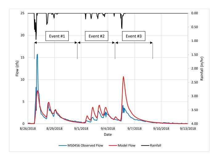
*Note.* The model substantially underpredicted the peak flow of Event #1 while it accurately predicted the volume. Event #2 and #3 were overpredicted by the model in both peak flow and volume.
