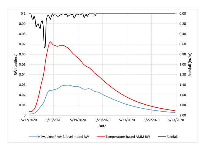
*Note.* The temperature-based AMM method substantially overpredicts the RW value during the RDI/I event for sewer MS0453.
