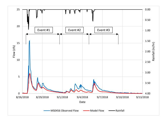
Note. The model substantially underpredicted the peak flow of Event #1 as well as the peak flows of Event #2. Peak flow of Event #3 was predicted accurately by the model. The volume of each event was slightly underpredicted by the model.
