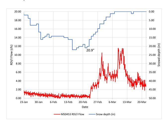
*Note.* Figure 11 shows the RDI/I response of sewer MS0453 due to a snowmelt event beginning around February 20, 2021. As the snow depth decreased from its peak of 20.9 inches, an increase in MS0453's flow was observed.
