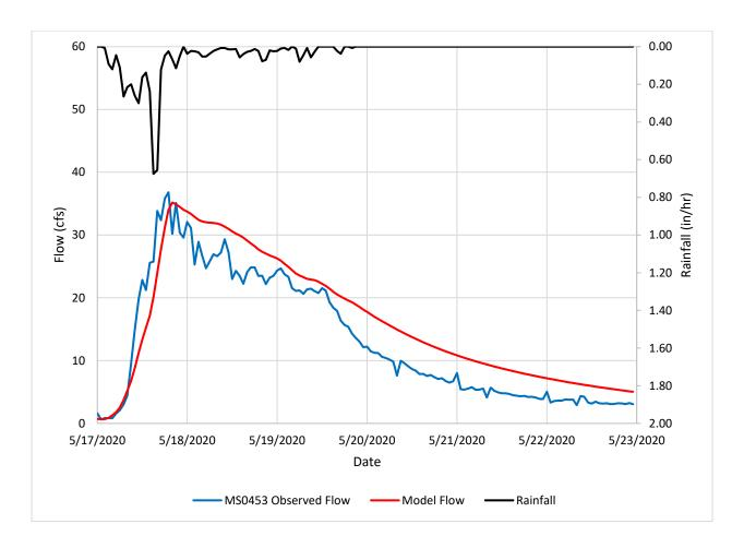
Note. The model accurately predicted the peak flow while it slightly overpredicted the volume.
