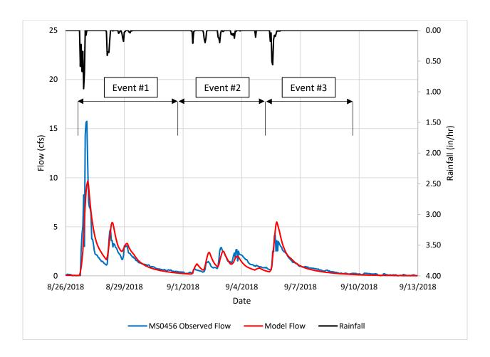
*Note.* The model underpredicted Event #1's peak flow while accurately predicting its volume. The peak flow and volume of Events #2 and #3 were accurately predicted.
