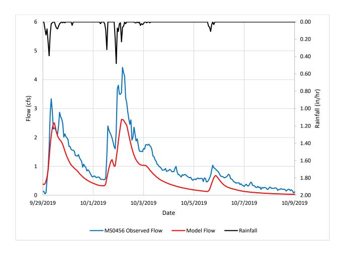
*Note.* The model substantially underestimated the peak flow and slightly underestimated the volume of the event.
