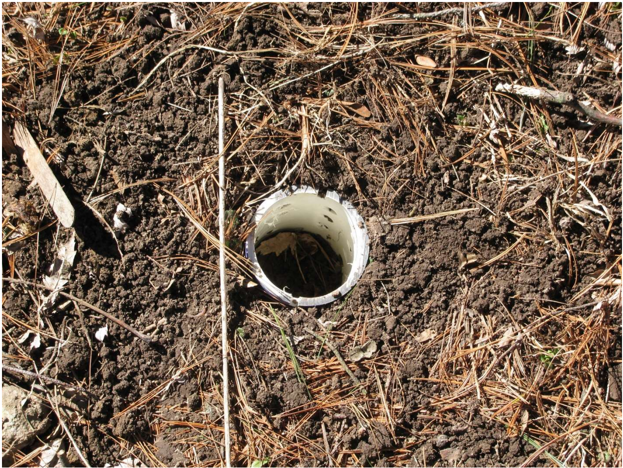
Figure 6. Garden water level sensor mounting tube.
