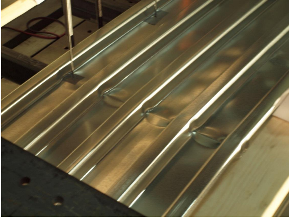
Figure 75: 22 Gage Deck Positive Bending - Further Buckling.
