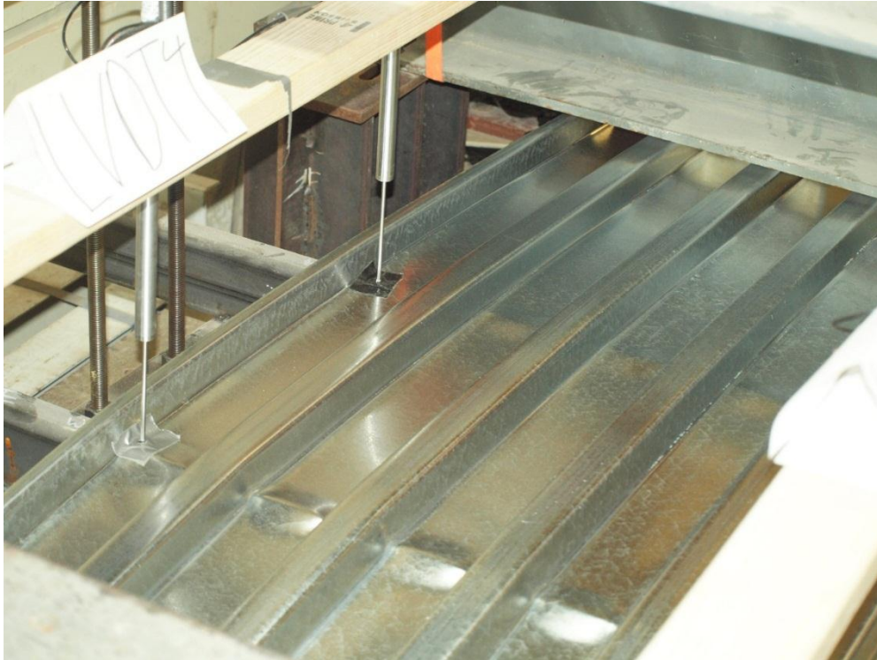
Figure 32: 16 Gage Deck Positive Bending - Further Buckling.
