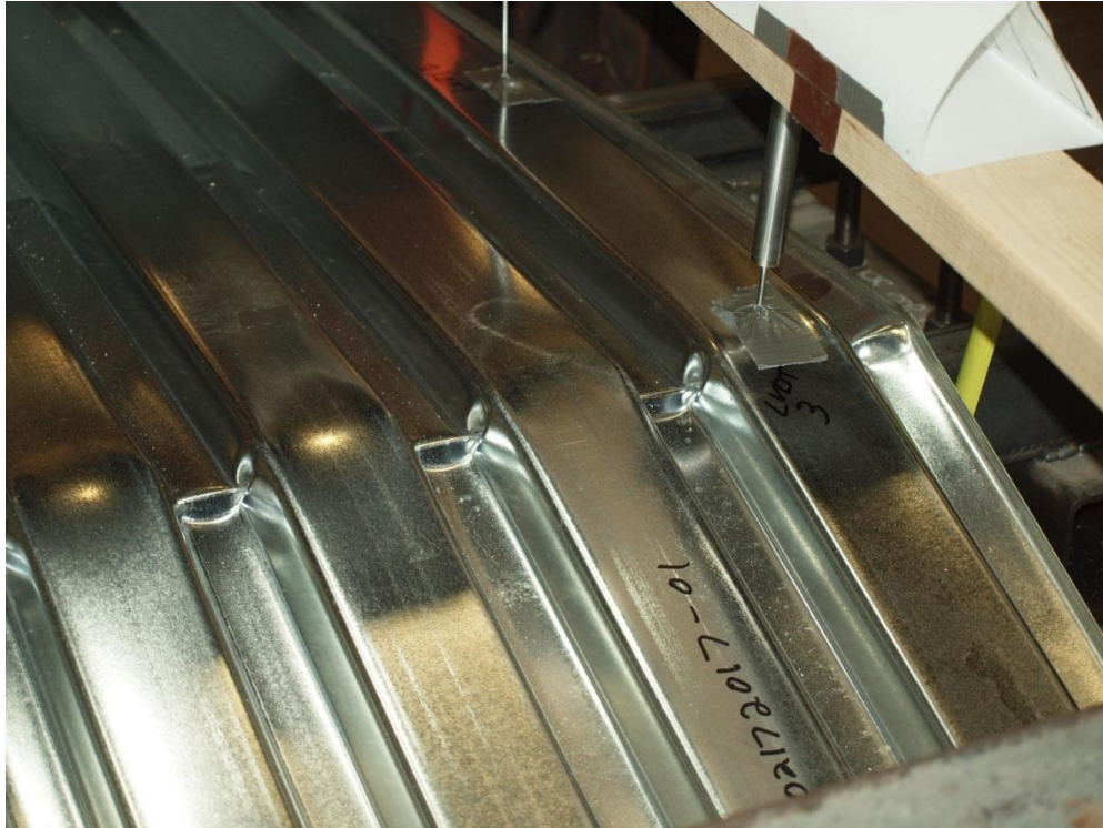
Figure 40: 18 Gage Deck Negative Bending - Further Buckling.
