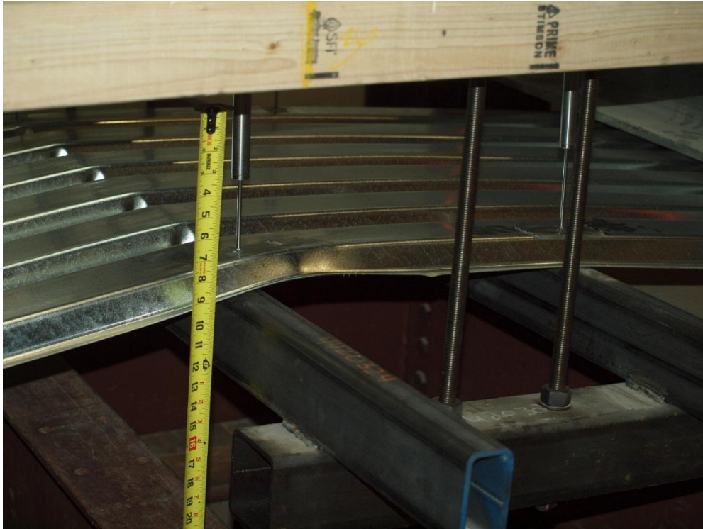
Figure 24: 16 Gage Deck Negative Bending - Final State.
