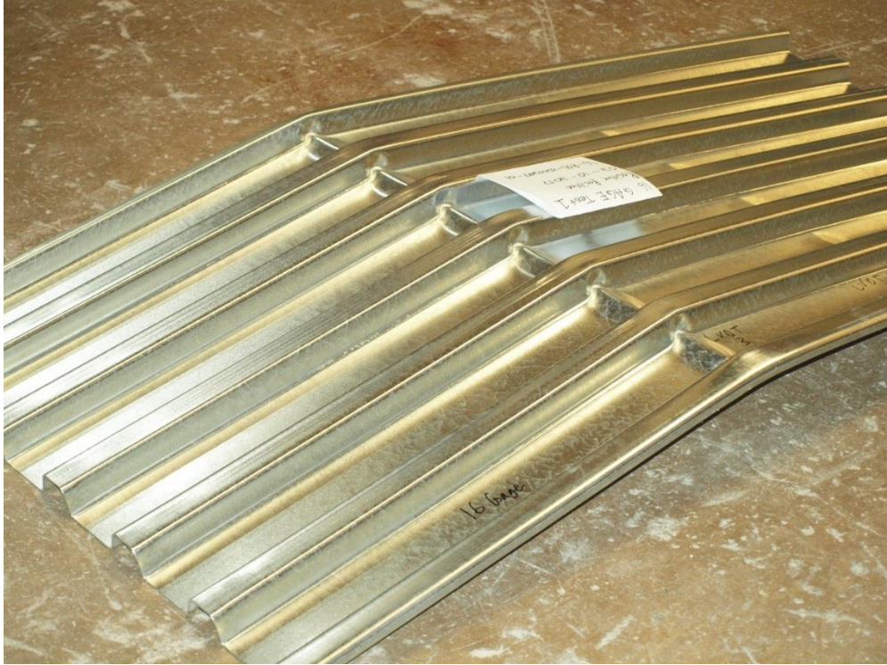
Figure 34: 16 Gage Deck Positive Bending - Final State.
