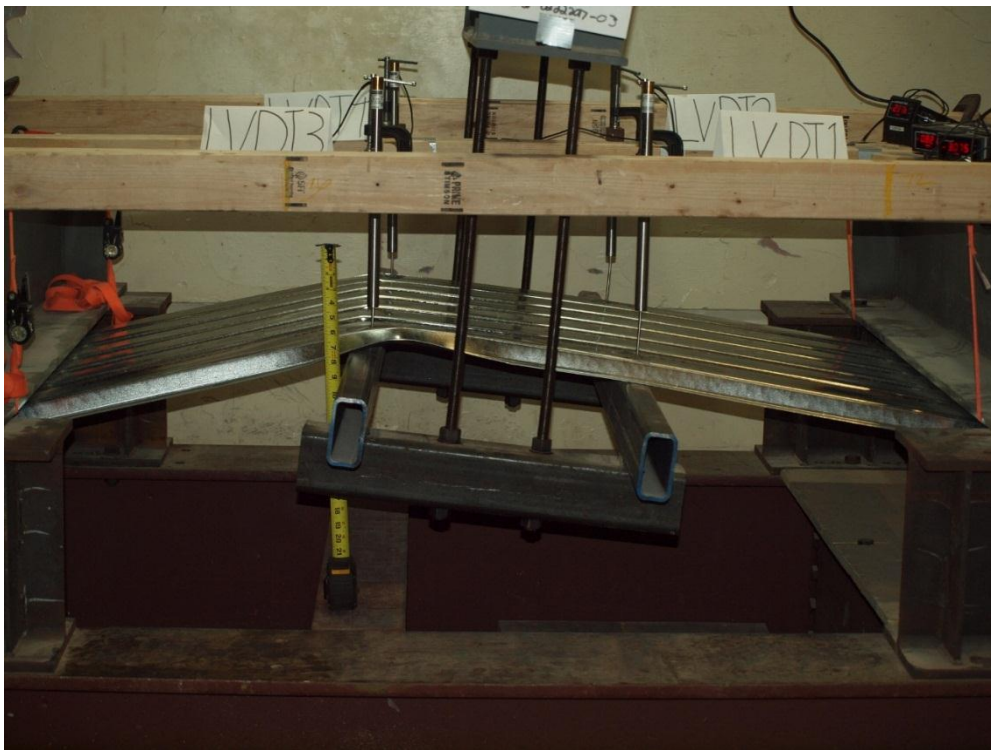
Figure 25: 16 Gage Deck Negative Bending – End of Test.
