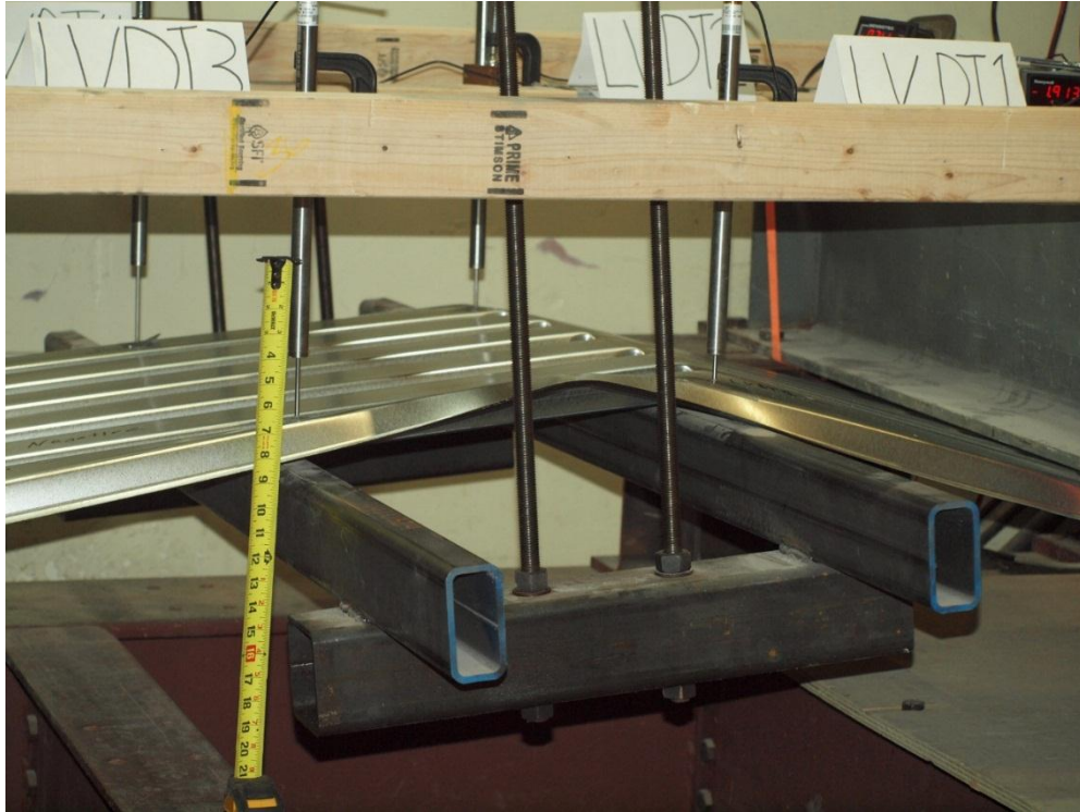
Figure 68: 22 Gage Deck Negative Bending - Final State.
