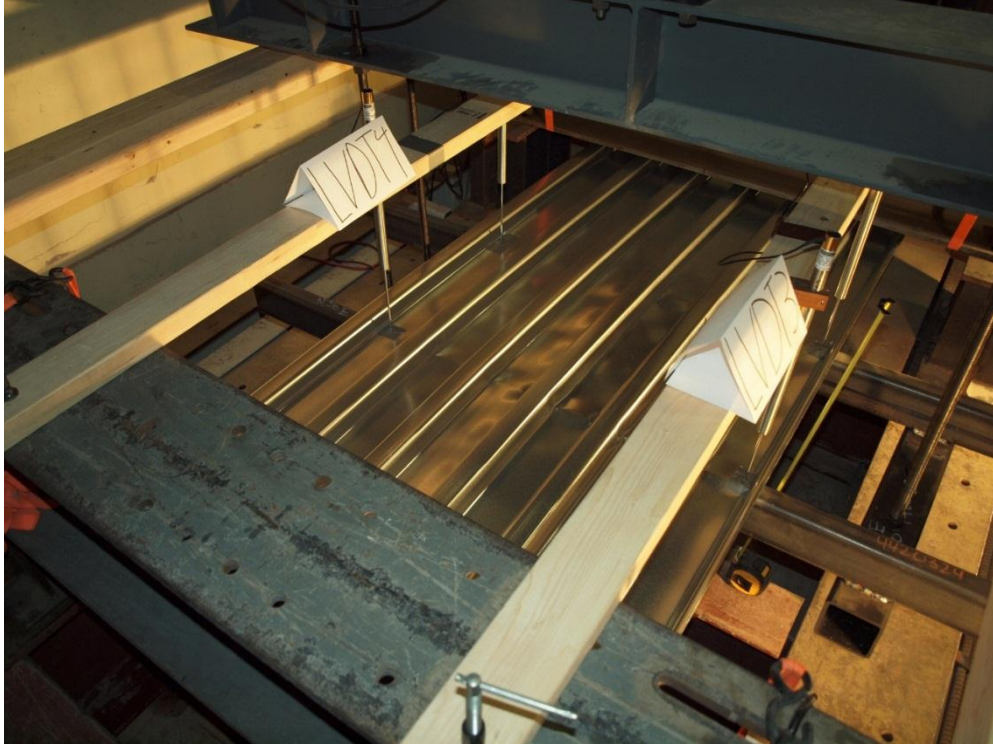
Figure 74: 22 Gage Deck Positive Bending - Initial Buckling.
