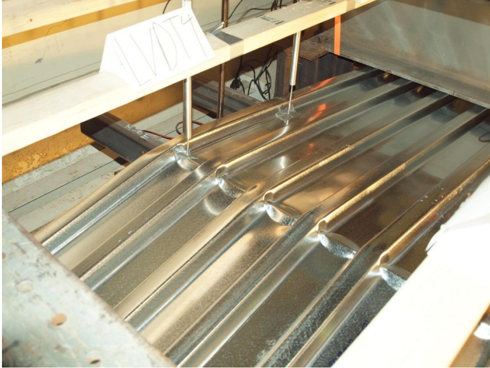
Figure 62: 20 Gage Deck Positive Bending - Final State.
