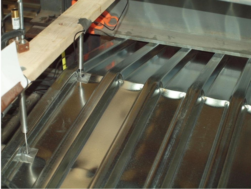
Figure 48: 18 Gage Deck Positive Bending - Further Buckling.
