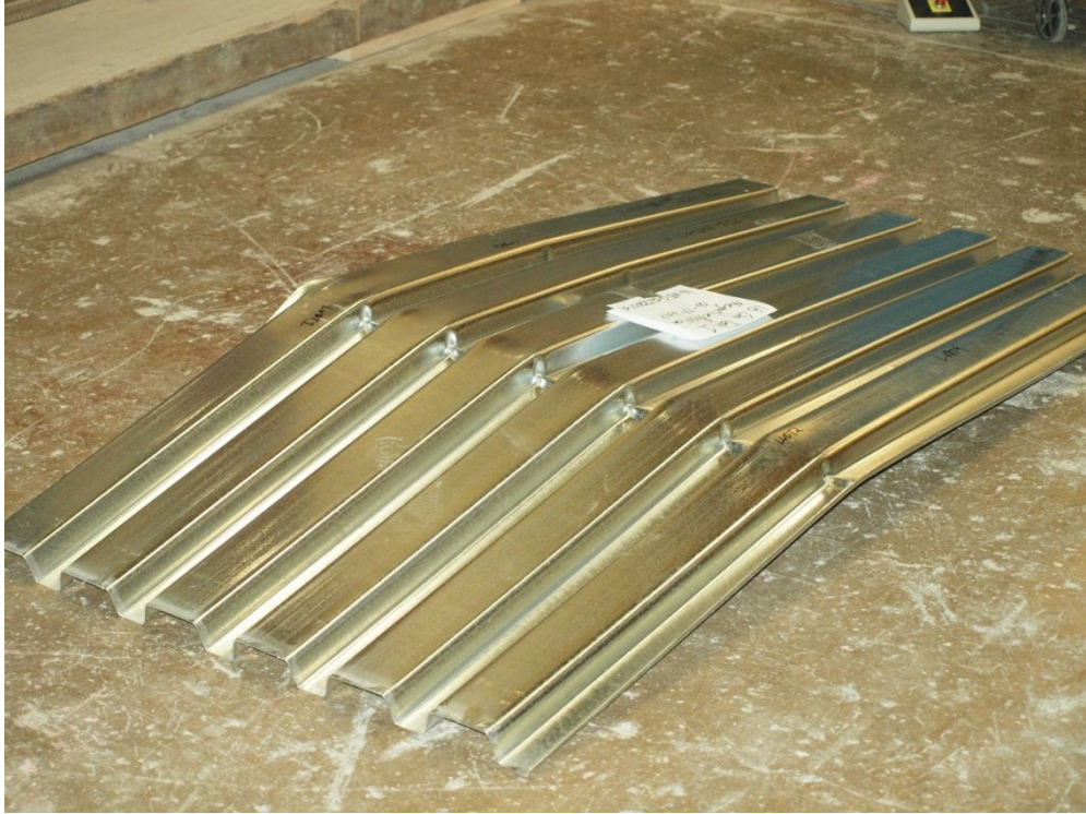
Figure 26: 16 Gage Deck Negative Bending – Specimen Removed.
