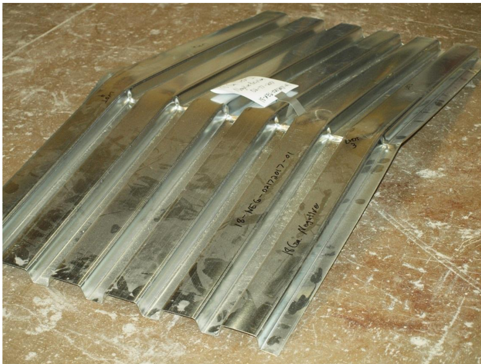
Figure 41: 18 Gage Deck Negative Bending - Final State.
