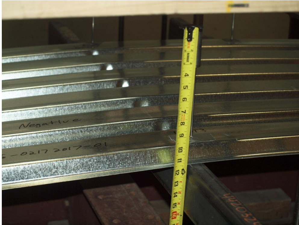
Figure 53: 20 Gage Deck Negative Bending - Initial Buckling.
