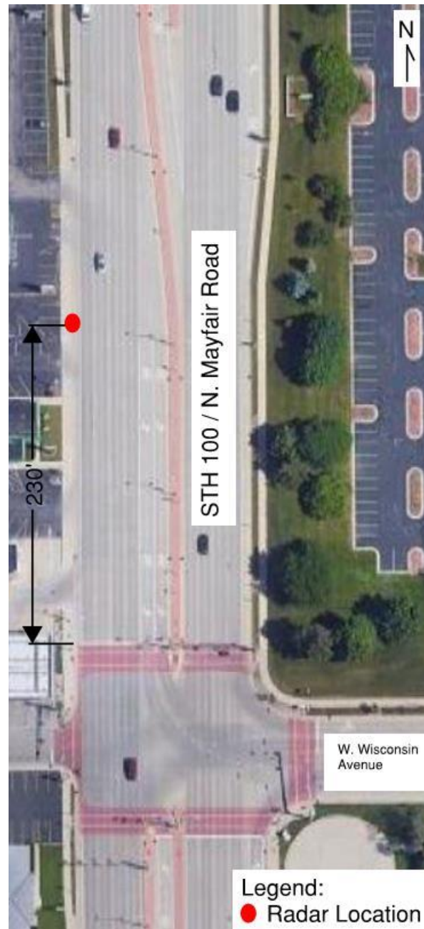
Figure 5: Radar Location for Gathering Deceleration Rate at STH 100 (N. Mayfair Road) and W. Wisconsin Avenue Intersection (Google, n.d.).
