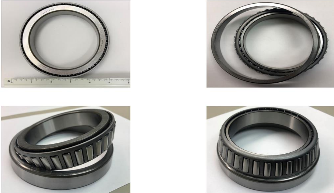
Figure 32: Koyo 32918JR Main Bearing.
