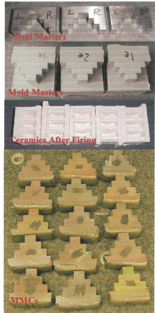
Figure 9. Metal Masters, Mold Masters, Assembled and Fired Ceramics, and Final Metal Matrix Composites (MMCs).
