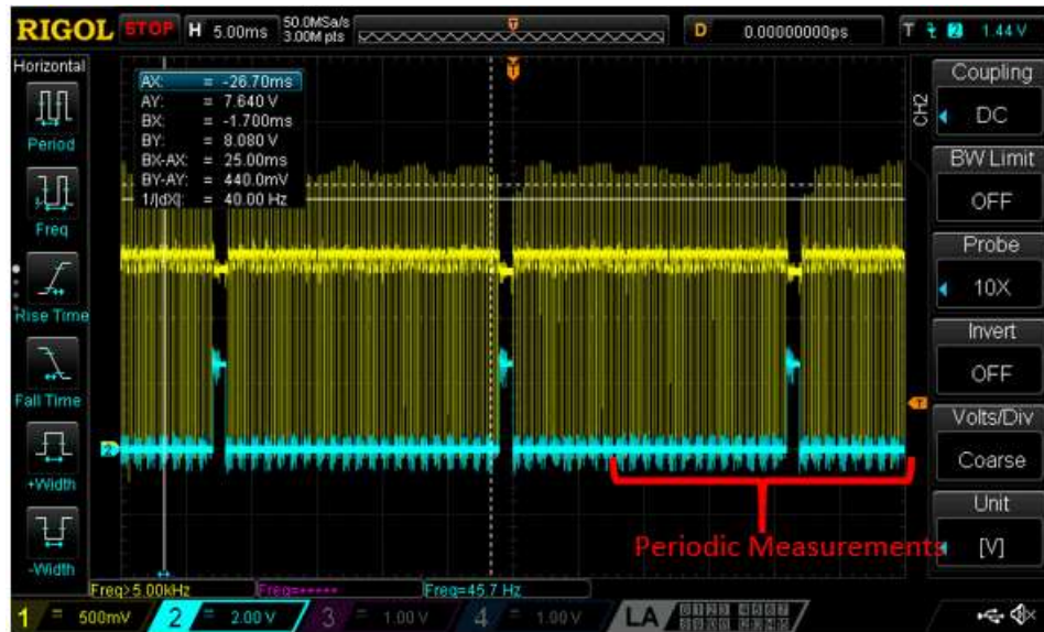
Figure 36: Measurement Frequency - CH1: Negative Motor Terminal Voltage.
