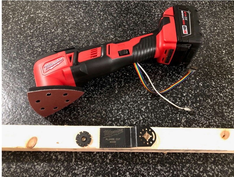
Figure 60: Test Tool with Sanding and Plunge Cutting Attachments.
