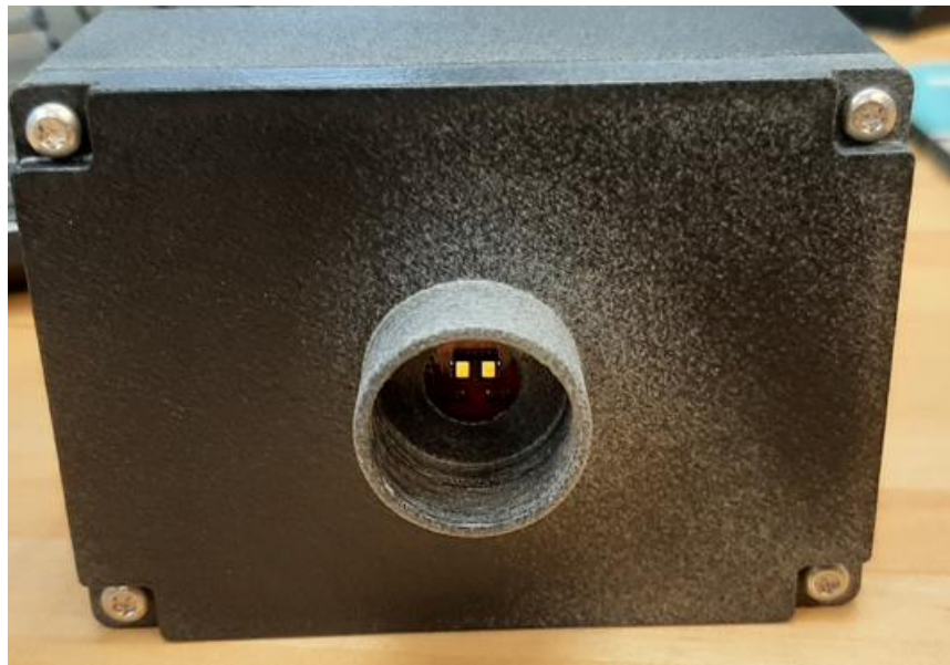
Figure 17: TOF LLI Sensor Unit Bottom View Showing VL53L1X Sensor.
