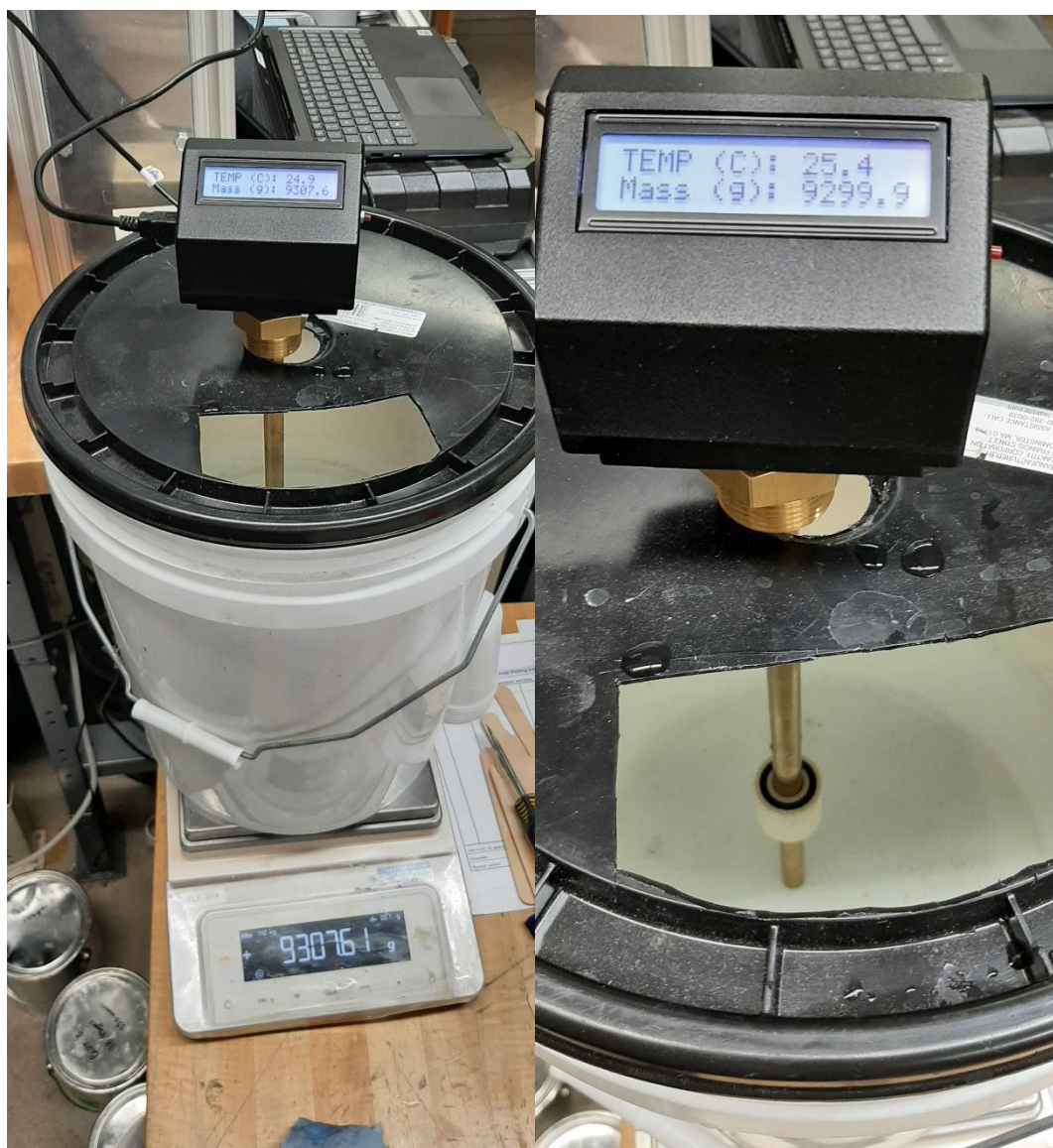
Figure 84: Verification of the LLI's Volume to Weight Conversion Algorithm.
