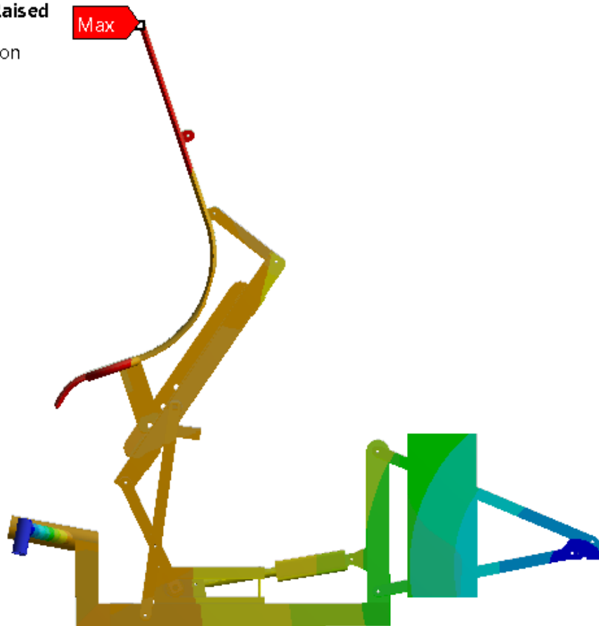
Figure 51: Total Deformation, with Undeformed Model Showing (True Scale).
