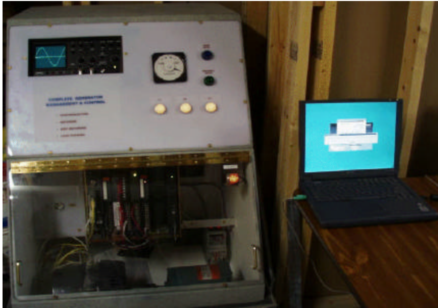
Figure 19: Line Synchronization Module Demonstration Case
