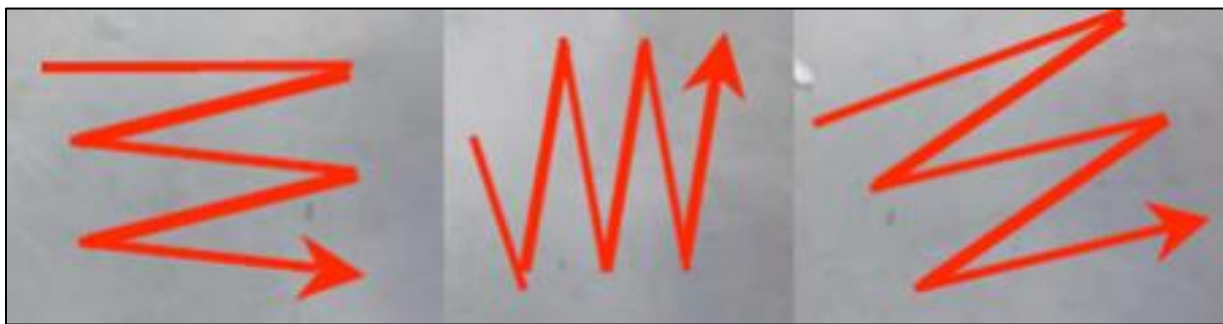
Figure 5: Swabbing Technique Used for Sterile Gown and Reservoir Sampling.
