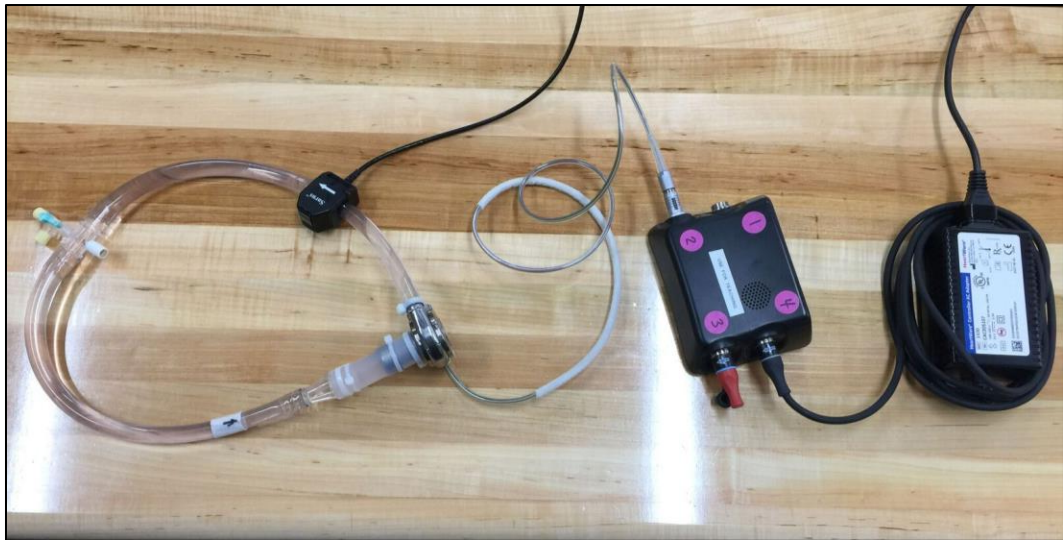
Figure 11: HeartWare VAS Circuit Setup. This circuit was used to test the functionality of the VAD when placed in hyperbaric conditions. The system controller and AC power adapter were placed in the chamber with the circuit.
