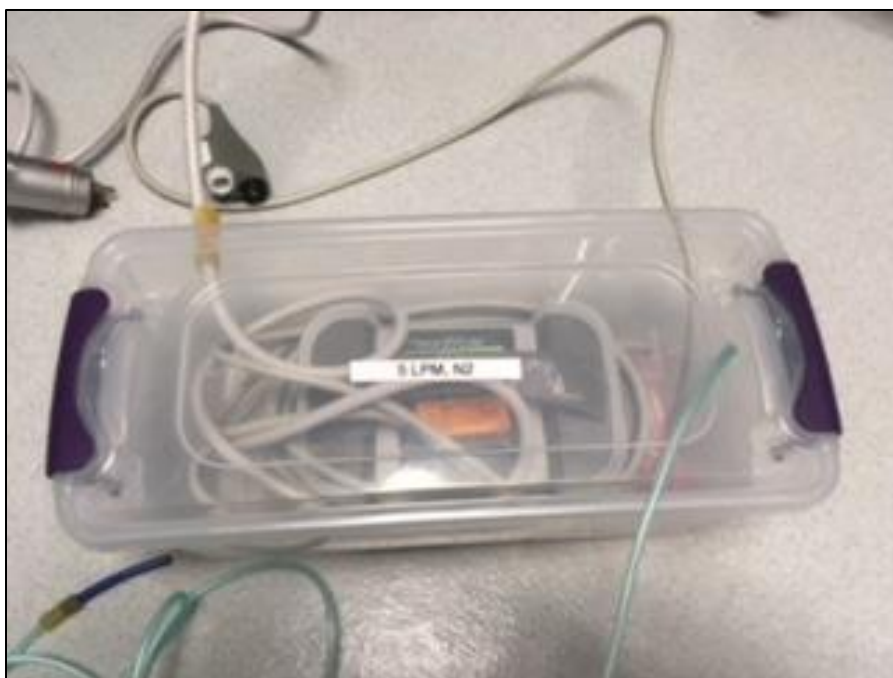
Figure 7: Enclosed Mobile Power Unit [44]. The MPU was enclosed and flushed with 15 LPM of N 2 and 1.3% of O 2 .
