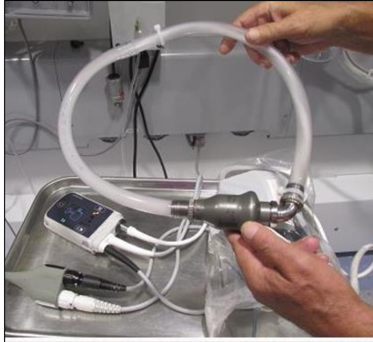
Figure 8: Water Filled Mock Circulatory System [44]. The mock circuit was used to simulate blood flow through the HM II LVAS.
