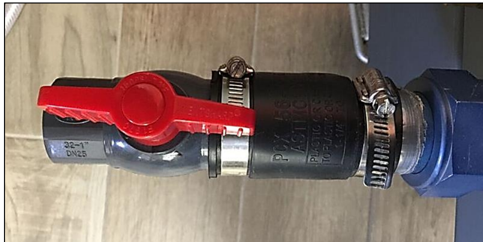
Figure 15: Mono-place Chamber Pressure Release Valve Opened 100%.
