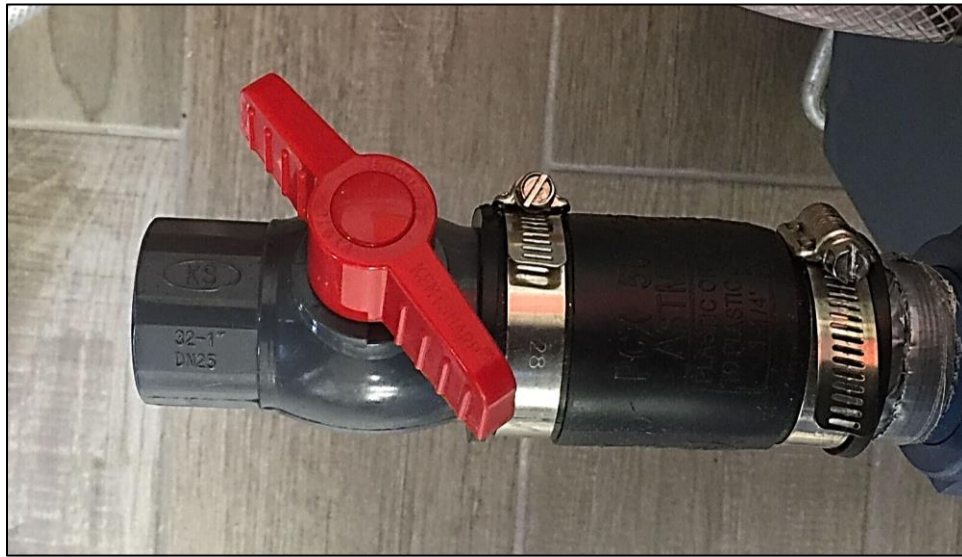
Figure 14: Mono-place Chamber Pressure Release Valve Opened 50%.
