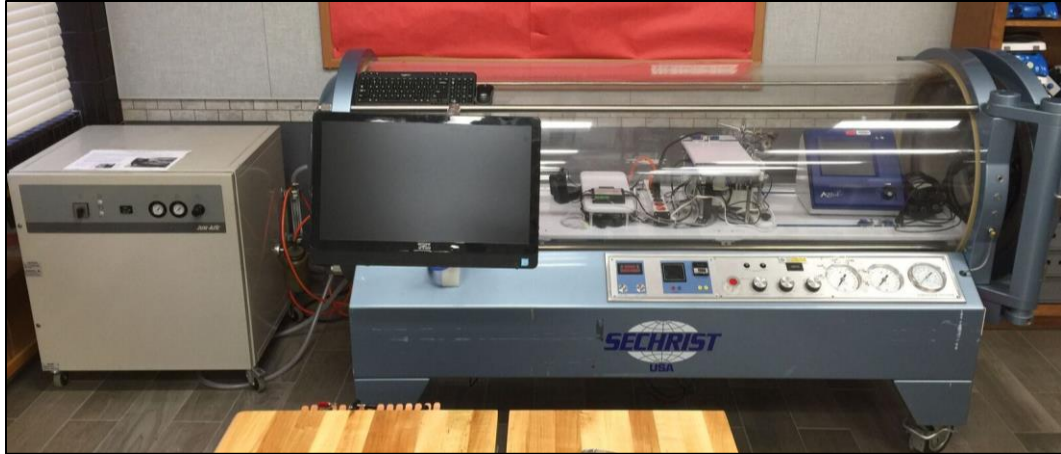
Figure 12: The Mono-Place Chamber Located at MSOE. The chamber was manufactured by Sechrist and pressurized by a Jun-Air Compressor. The mock circuit and monitoring equipment were placed inside the circuit and powered using an AC power strip.
