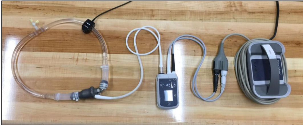
Figure 10: HeartMate II LVAS Circuit Setup. This circuit was used to test the functionality of the VAD when placed in hyperbaric conditions. The system controller and mobile power unit were placed in the chamber with the circuit.
