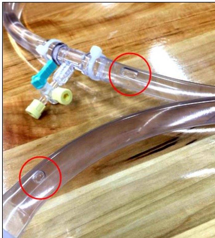
Figure 16: Air in the Water-Filled Mock Circuit Following Trial Completion. The air is circled in red. Both the HM II LVAS water-filled mock circuit and the HW VAS water-filled mock circuit generated air.
