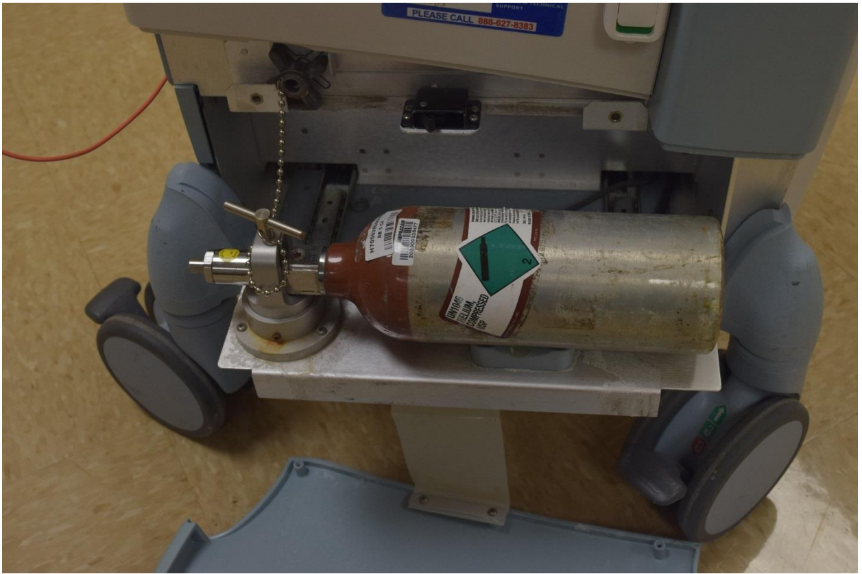
Figure 8. This is a View of the Lower Left Side of the CardioSave Hybrid IABP by Maquet. The lower left panel is removed, exposing the helium tank. The tank is then slid out to be removed.
