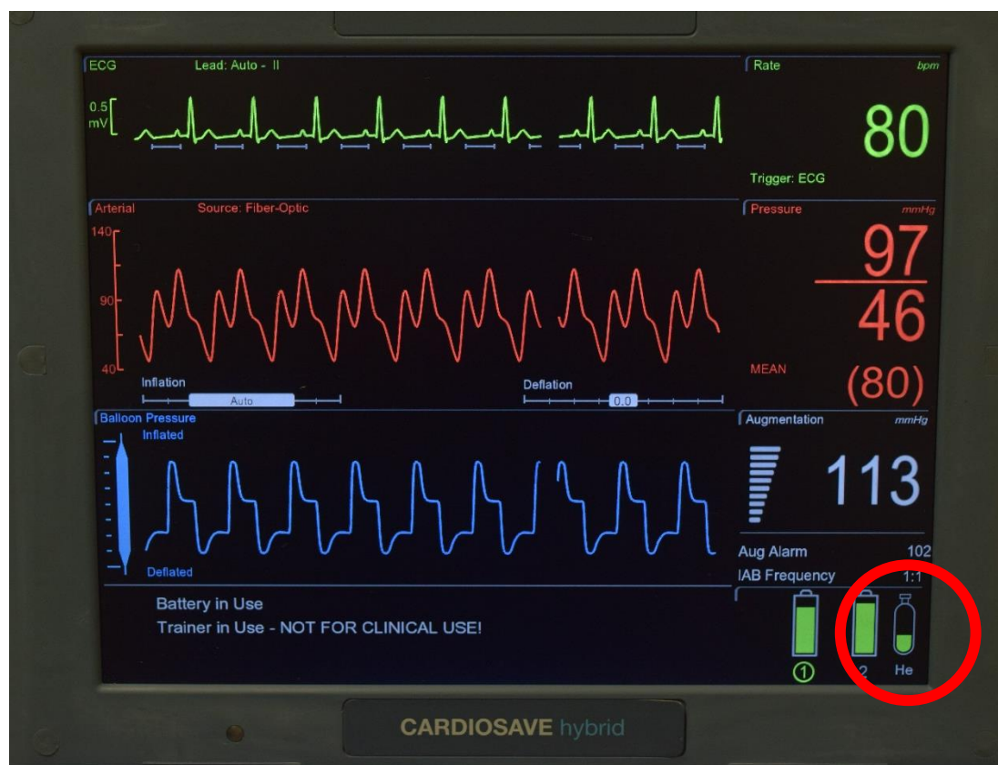
Figure 6. The Helium Tank Level is Indicated by the Helium Tank Symbol in the Lower Right Corner of the Upper Monitor. The helium tank symbol is circled in red.
