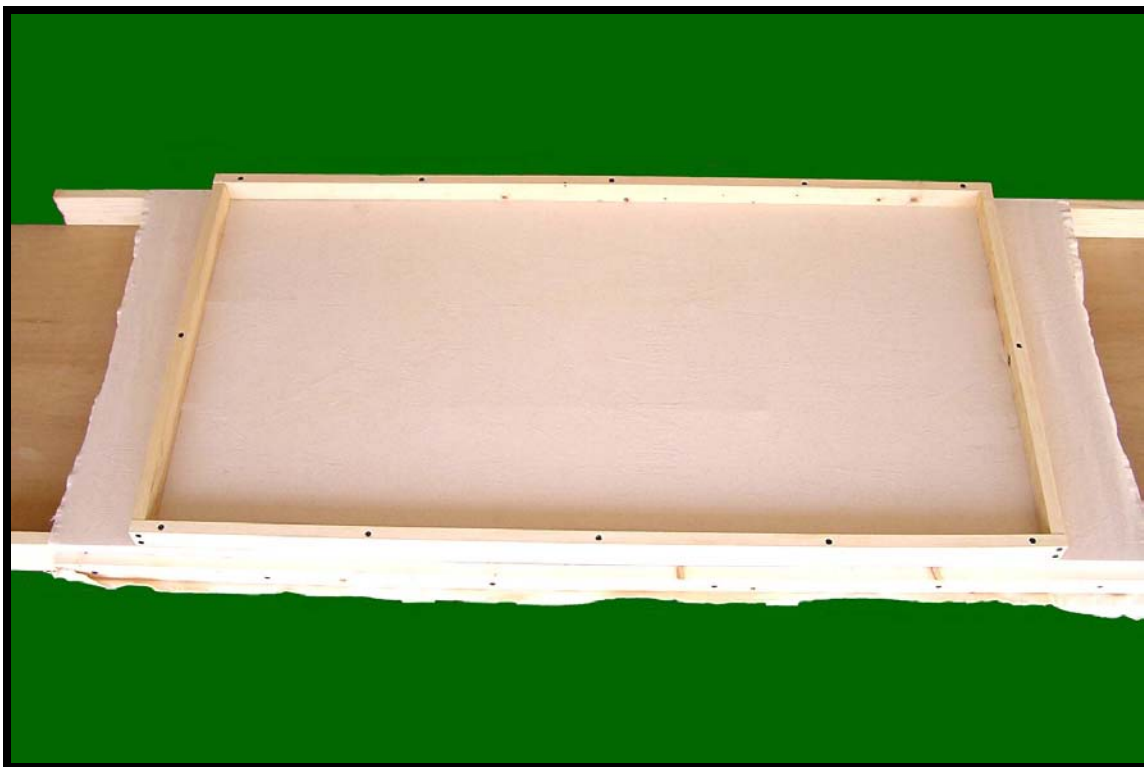
Figure D2. Panel 5 – Fabric Stretched onto Frame.
