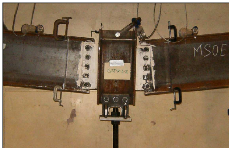
Figure 3.15: Typical Connection Failure Visual Verification.
