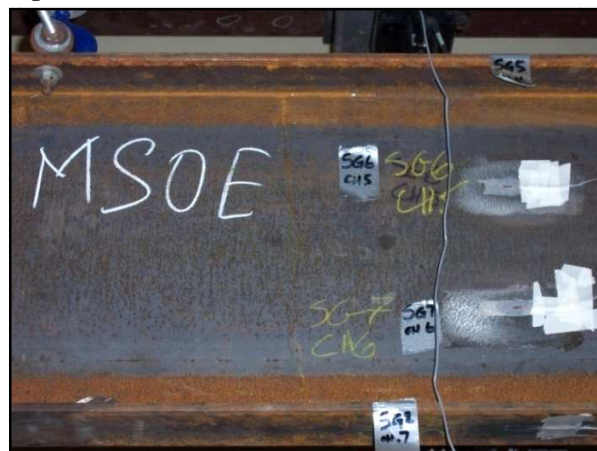
Figure 3.14: Typical Strain Gage Placement on Test Beam.
