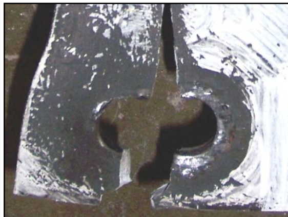
Figure 4.22: Specimen 4STL3 Bottom Hole Failure Mechanism.
