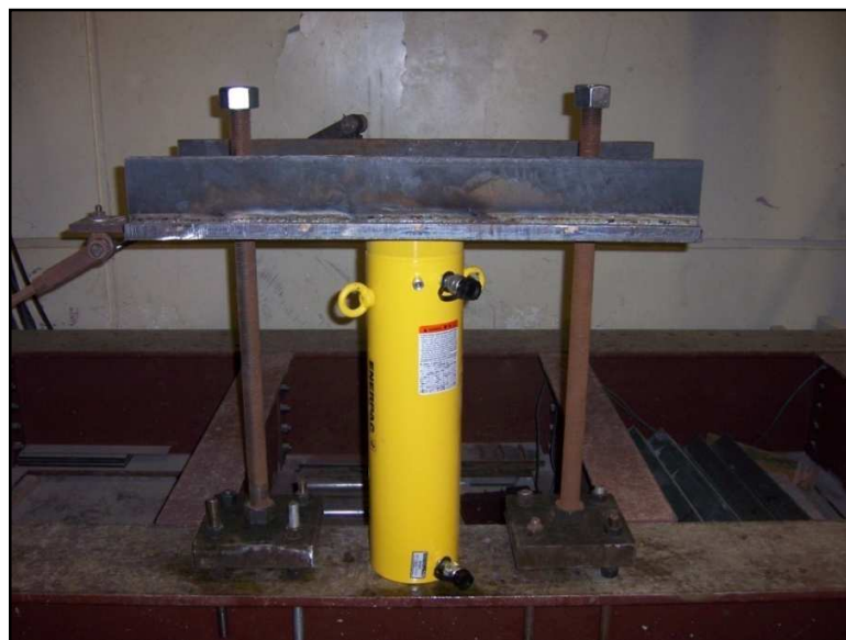
Figure 3.10: Hydraulic Cylinder Erected Condition.
