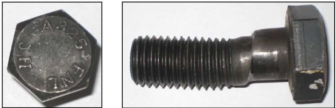
Figure 4.5: Typical Bolt Cross-Section Area Deformation.
