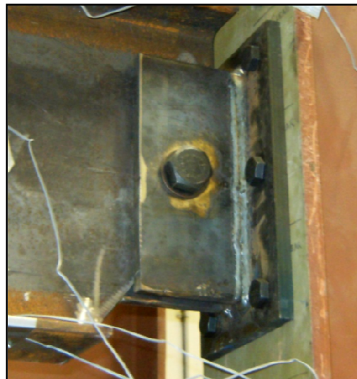
Figure 3.8: Erected True Pin Connection.
