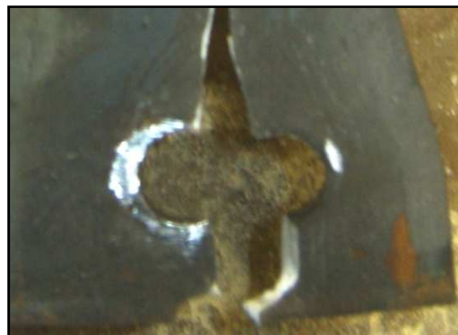
Figure 4.7: Specimen 3STR2 Rupture Source.
