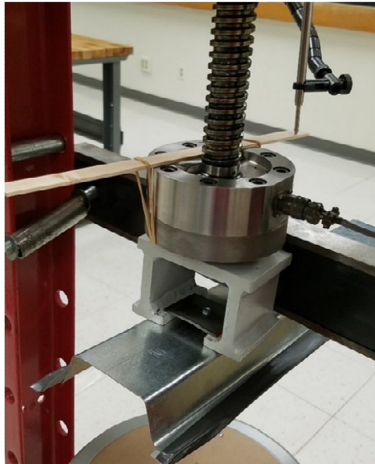
Figure 3.3-1. Screw pullout/rupture capacity setup.
