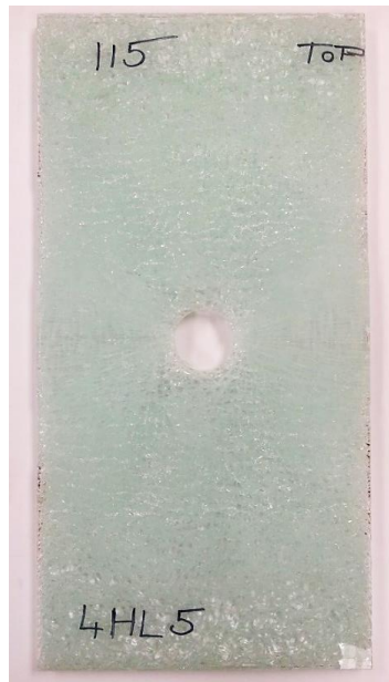
Figure 27: Typical Breakage of Laminated Glass.
