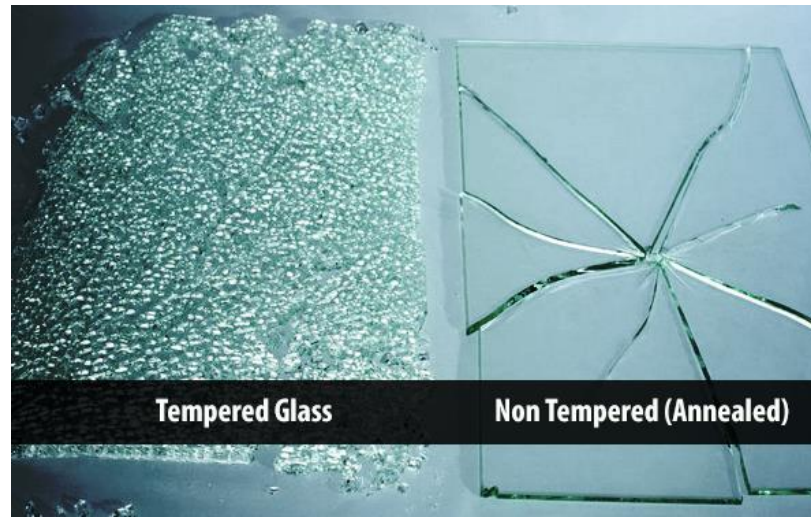
Figure 11: Annealed and Fully Tempered Glass Breakage Patterns [20].
