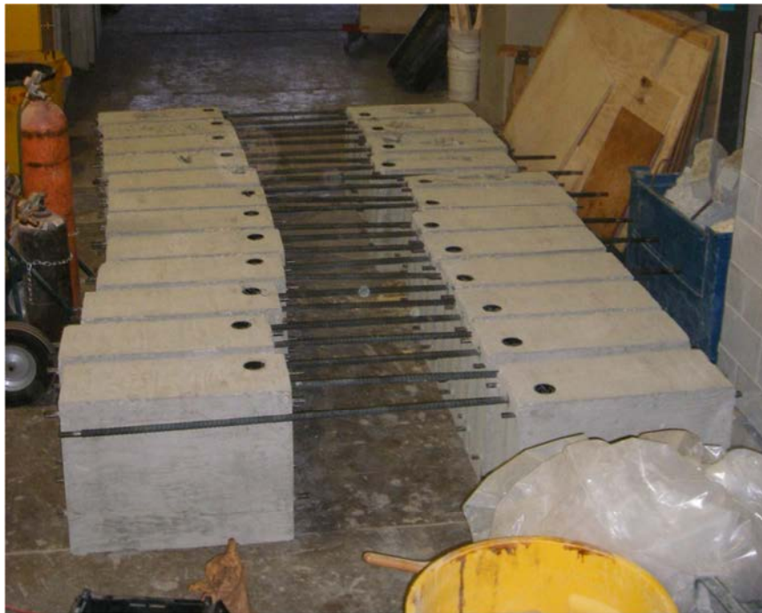
Figure 23 - Finished Specimen Showing Rebar Projection.
