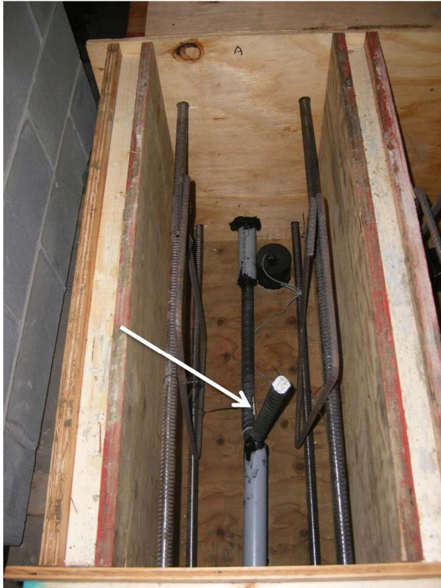
Figure 50 - Example Strain Gauge Location.
