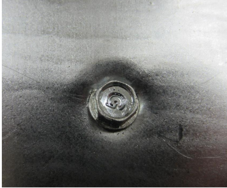
Figure 14: Bending Deformation Zone of the Metal Sheathing Panel [3].
