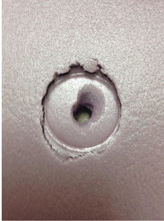
Figure 32: Crushed Insulation Member after Completed Washer Test.
