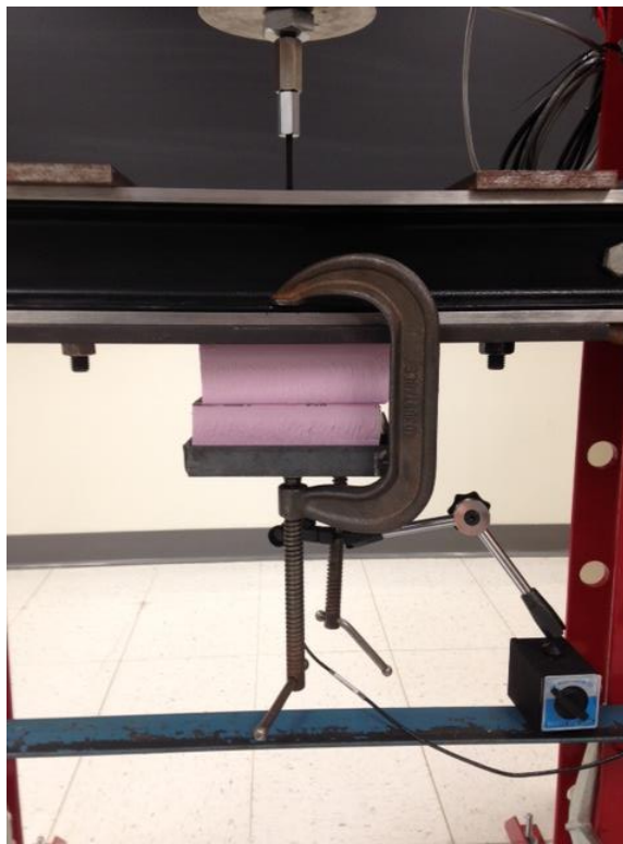
Figure 21: Frame Clamped onto Load Cell Channel.
