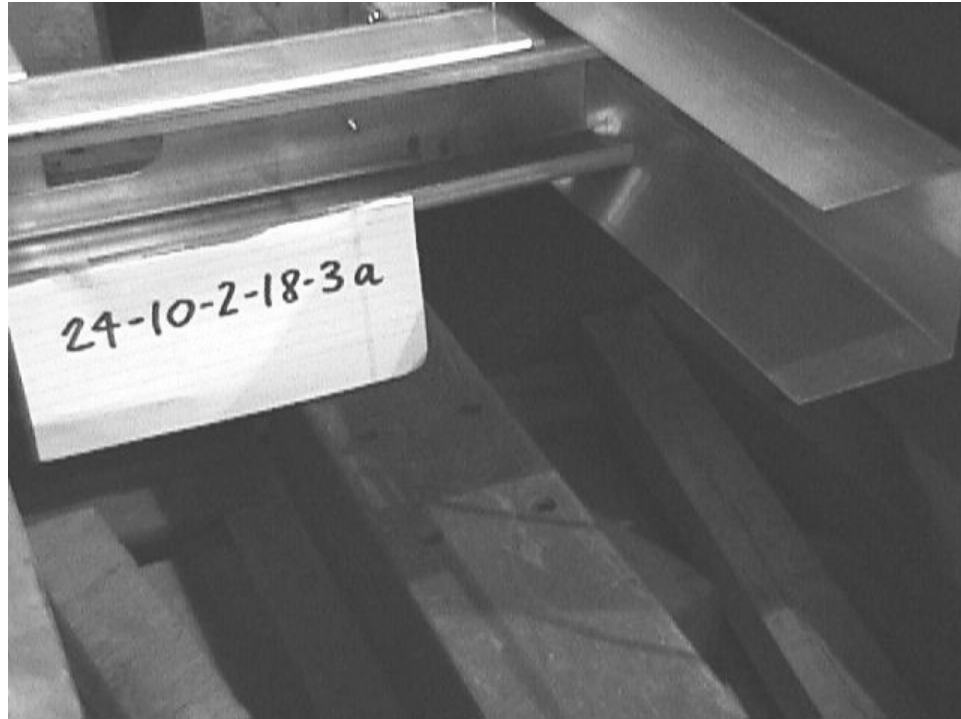
Figure 3.4-4 — Stud Flange Rotating During Test.
