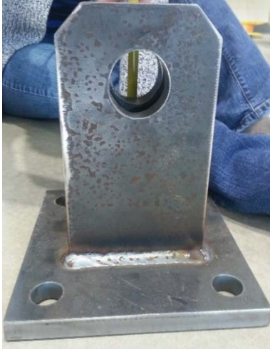
Figure 3.3-4a: Front View Connection from Actuator to Column Stub.
