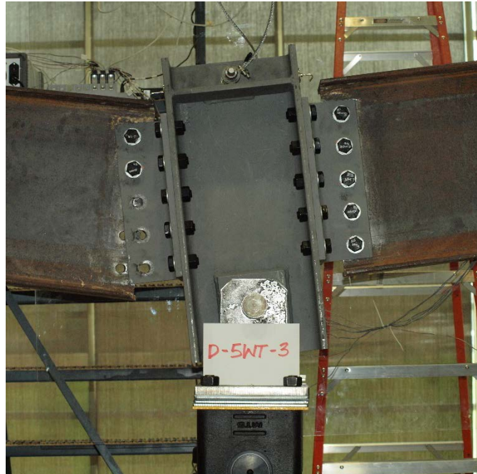
Figure 4.3.3.3-2: D5WT3 Post-Test Position.
