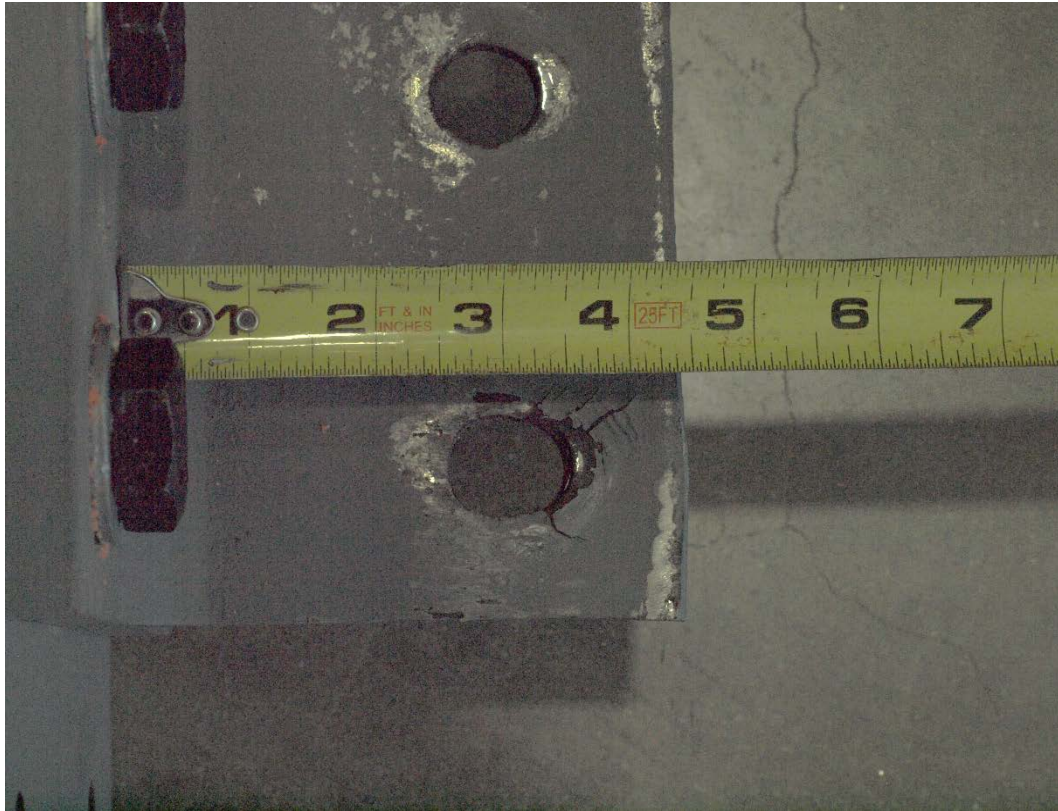
Figure 4.3.1.1-4: S3WT Right WT Specimen Post-Test.
