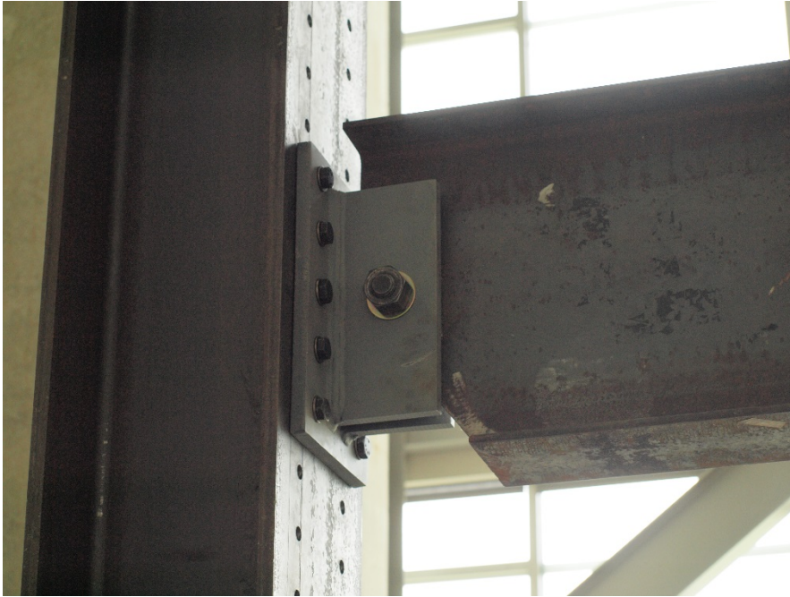
Figure 3.3-3 Pin Connection to Test Frame Column.
