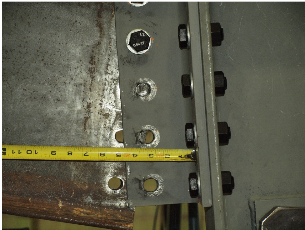
Figure 3.4.4-2: Typical Measurement of Column Stub Rotation.
