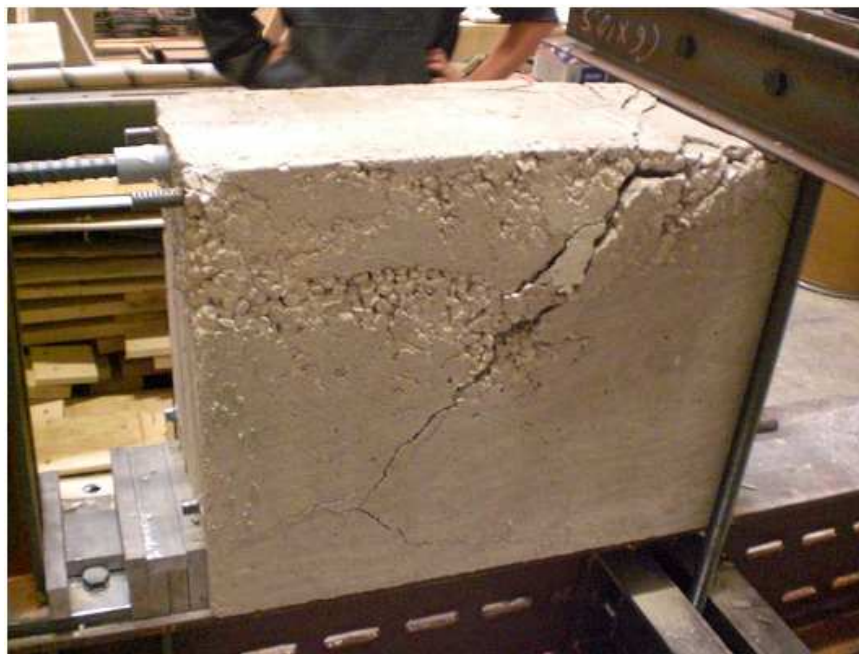
Figure 12: Typical Cracking Pattern of Shear Failure [3].
