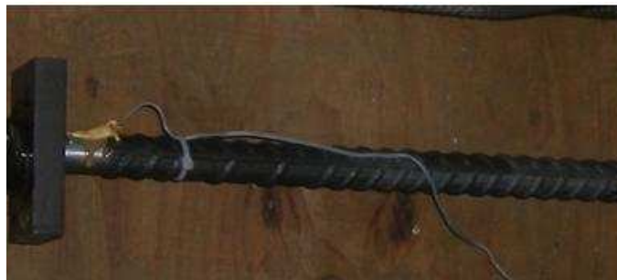
Figure 32: Headed Bar with Strain Gauge Attached.
