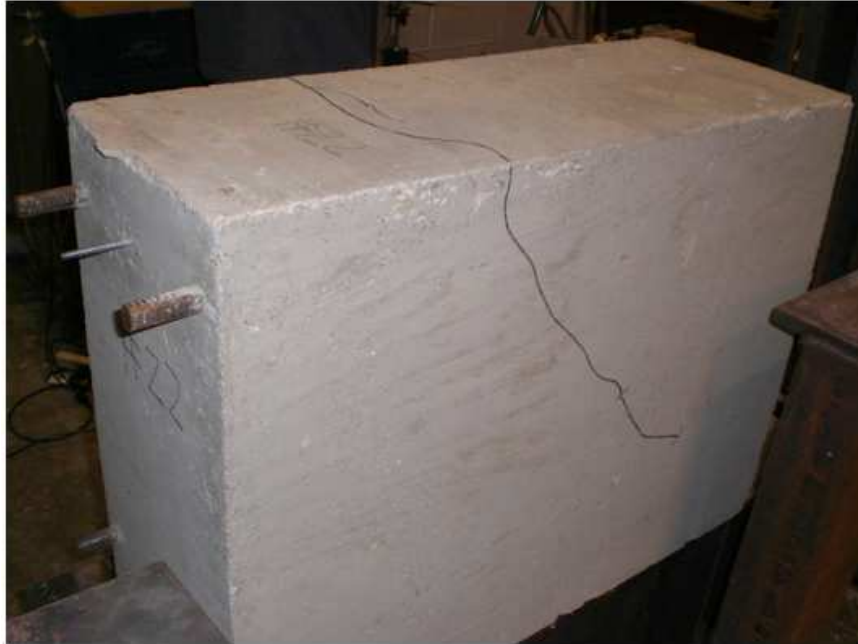
Figure 9: Typical Cracking Pattern of Specimens with Tension Yielding [3].
