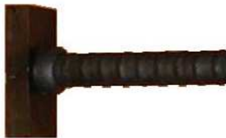
Figure 6: Headed Bar Specimen [3].
