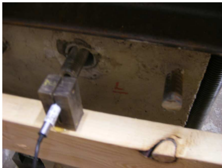
Figure 39: Head Slip LVDT.
