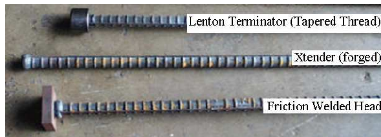
Figure 27: Types of Heads Tested [4].
