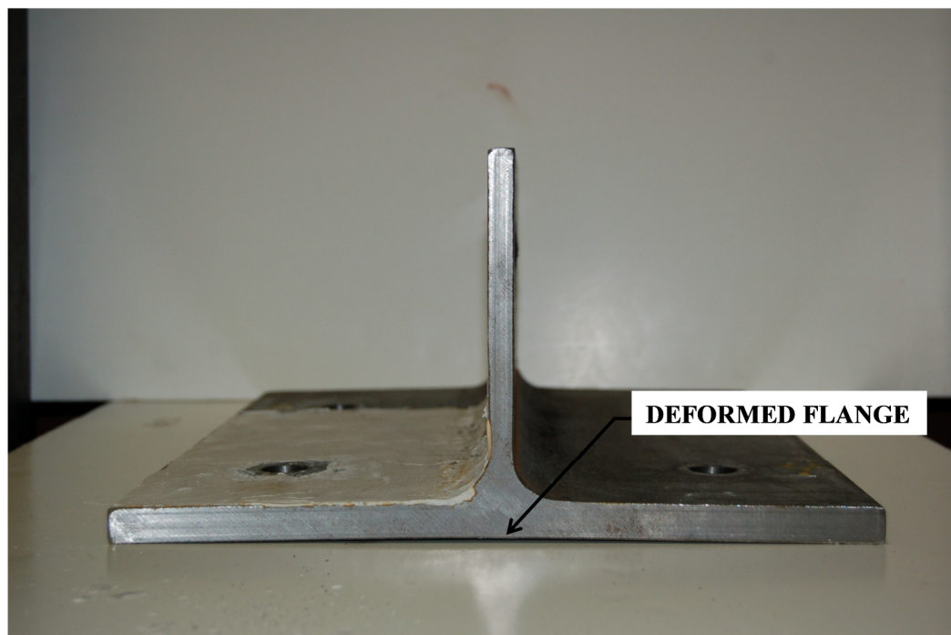
Figure 5.2.3-2: Deformed Shape for Specimen 2.5b Post-Testing.
