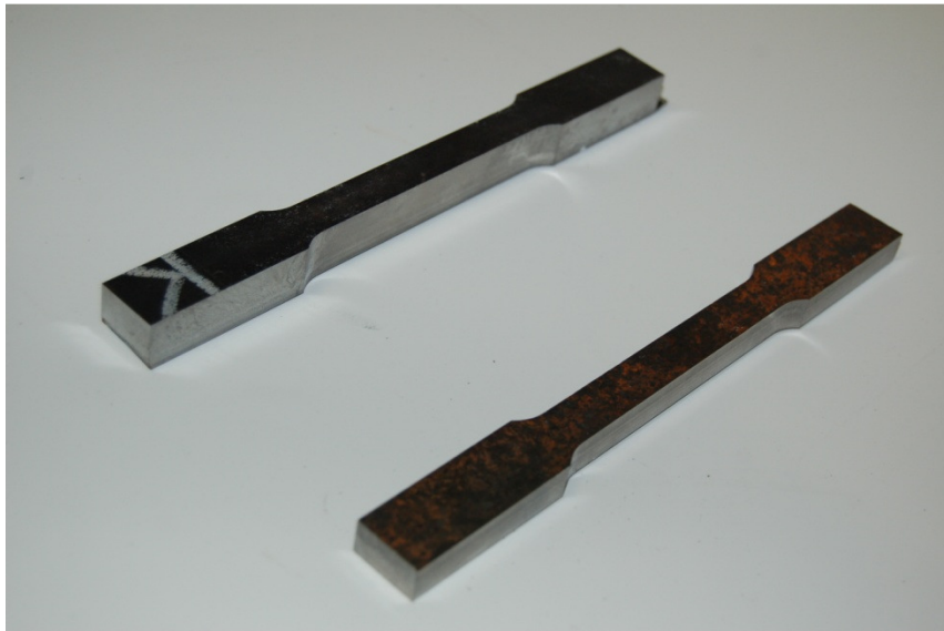
Figure 5.3-1: Dogbone-Shaped Specimens for WT6x32.5.
